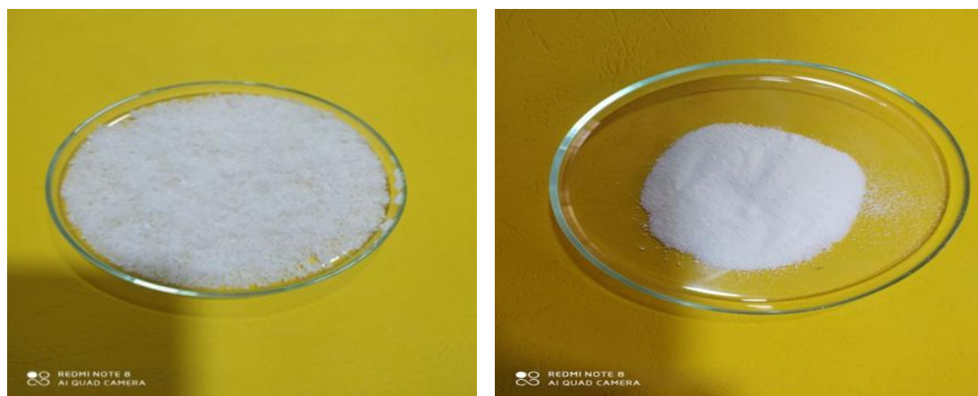
Fig. 1. a) Photos of nano binary oxide ZnO/SiO 2 by the Sol-Gel method before calcination and after calcination (b).
