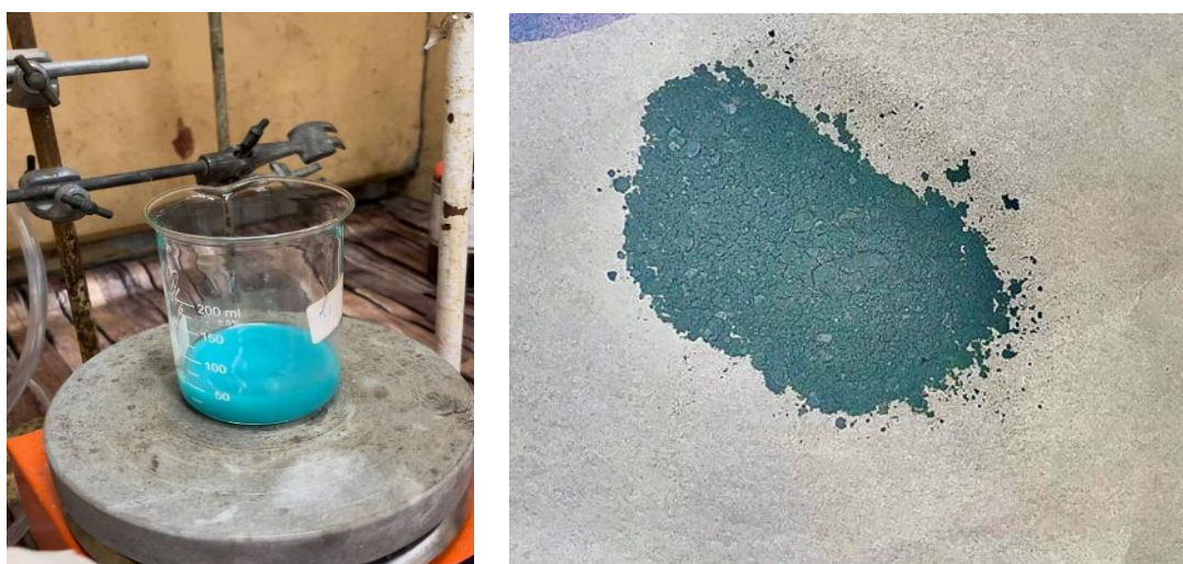
Fig. 1. Images of MoO 3 -NPs, synthesis by sol-gel methods.
