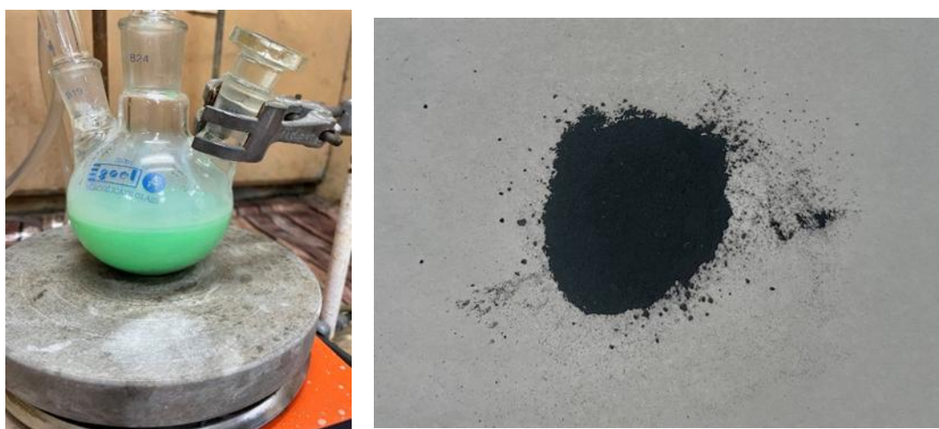
Fig. 2. NiO-NPs, synthesis by sol-gel methods.
