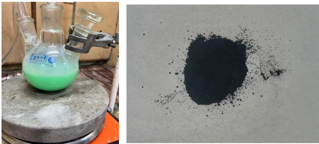
Fig. 2. NiO-NPs, synthesis by sol-gel methods.
