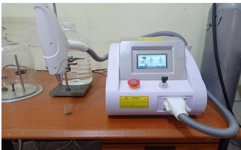
Fig. 2. PLA System using Nd:Yag laser.
