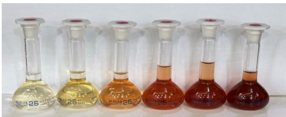
Fig. 2. AgNPs have been prepared by the reduction of aqueous solution AgNO 3 using Zamioculcas Zamiifolia leaves extract.
