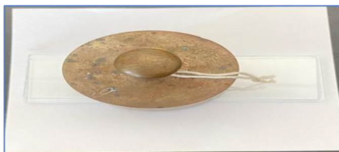
Fig. 1. Assembly for spreadability test.
