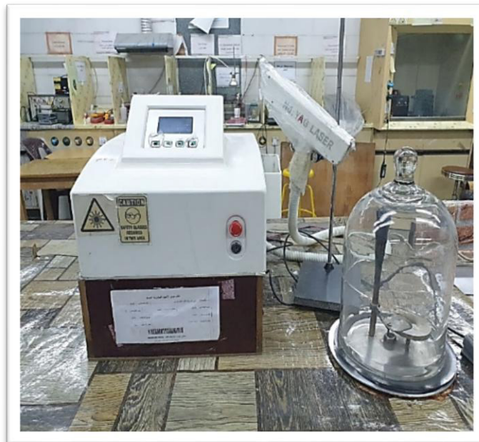
Fig. 1. Illustrate the parts of the PLD system
