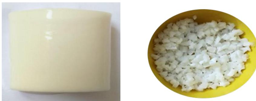
Fig. 1. Prepared CS-g-P(CMC-co-AM) nano hydrogel.
