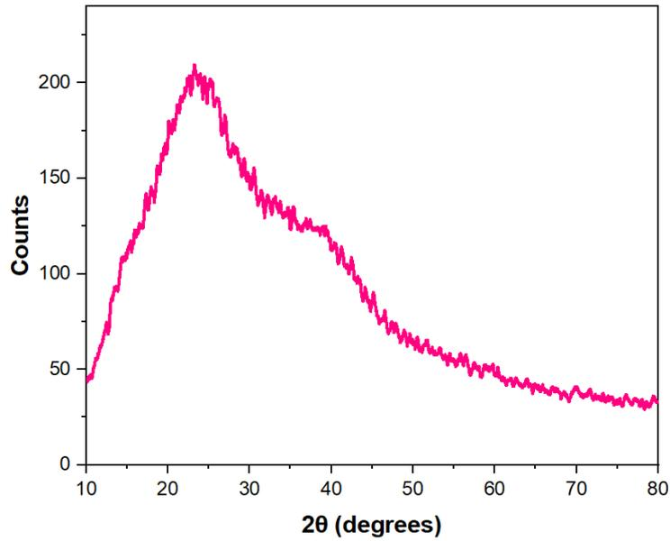
Fig. 3. XRD of prepared CS-g-P(CMC-co-AM) nano hydrogel.
