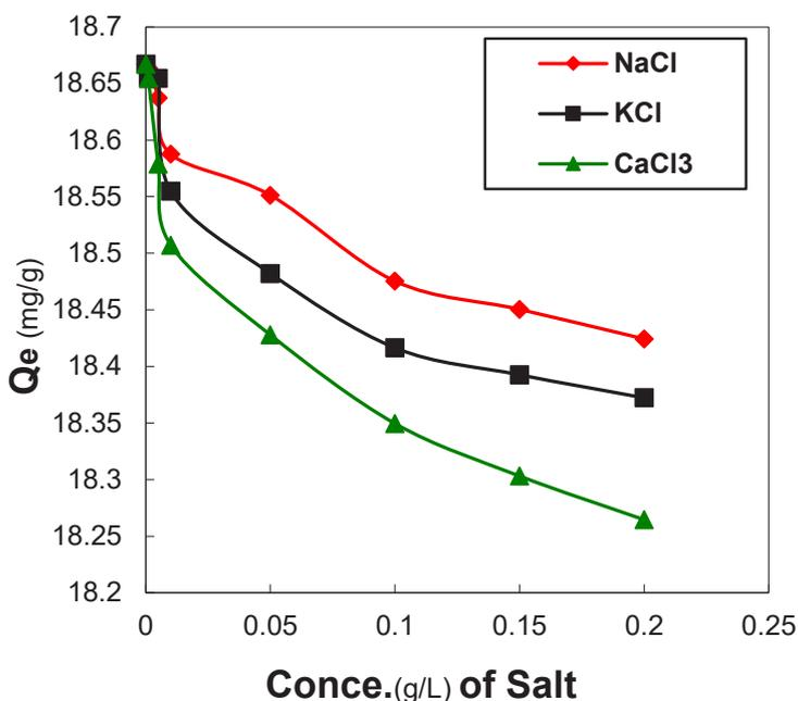
Fig. 10. Effect of different salts on adsorption of Cd (II) ions on prepared nano hydrogel.
