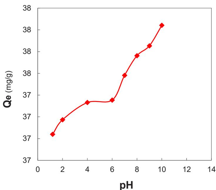
Fig. 7. Effect on pH on adsorption of Cd (II) ions on prepared nano hydrogel.
