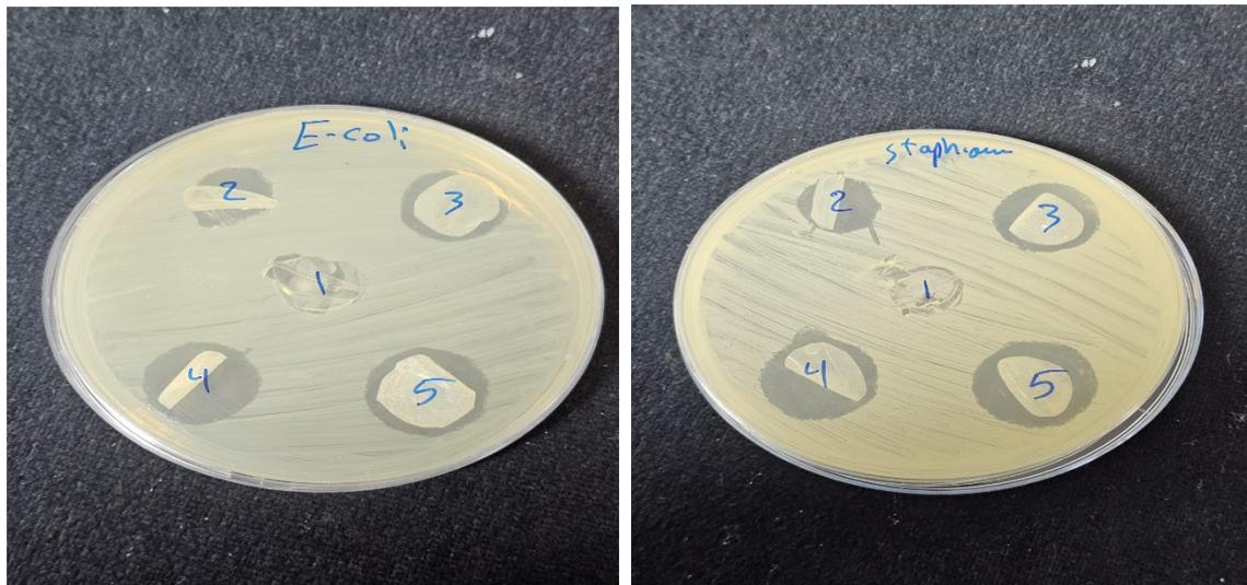
Fig. 10. Image for inhibition zones of  $PVA/Y_2O_3/SrCO_3$  nanocomposites with different concentration on *S. aureus* and *E. coli*
