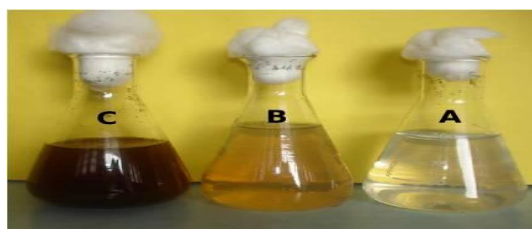
Fig. 1. Showed (A) FeNPs alone (B) biosynthesis FeNPs after 24hrs. (C) Biosynthesis FeNPs after 72 hrs.
