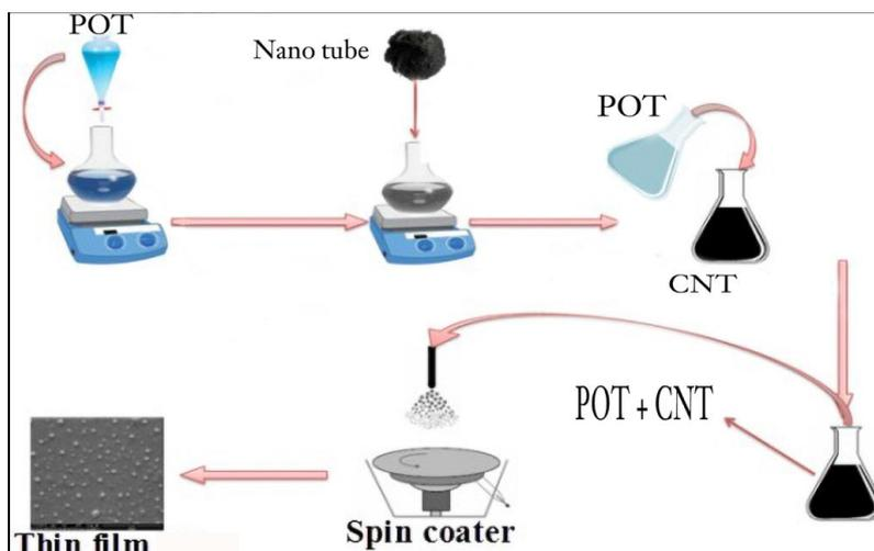
Fig. 1. Schematic representation of the film fabrication process for poly (O-Toluidine)-MWCNT films using the spin coating method
