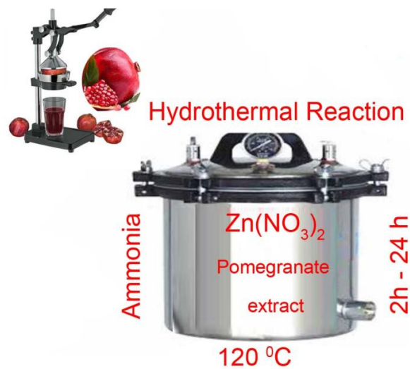
Fig. 1. Schematic of green synthesis of zinc oxide with hydrothermal reaction
