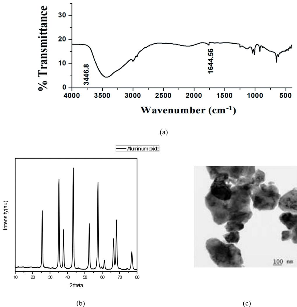
Fig. 1. Analysis results of Al<sub>2</sub>O<sub>3</sub> NPs: (a) FTIR spectroscopy, (b) XRD image, and (c) TEM image.
