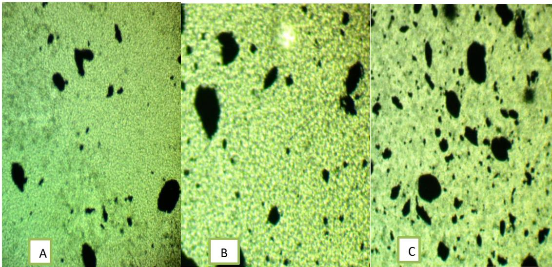
Fig. 2. Photomicrographs (100X) of nanocomposites a) PAAm-PEG :0.02wt.% Ag, b) PAAm-PEG:0.04wt.%Ag, and c) PAAm-PEG:0.06wt.%Ag.
