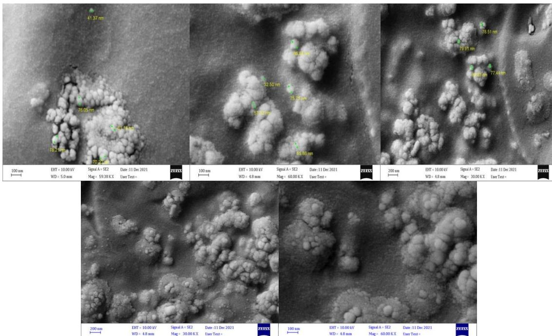
Fig. 4. SEM images of PAAm-PEG-Ag nanocomposite.
