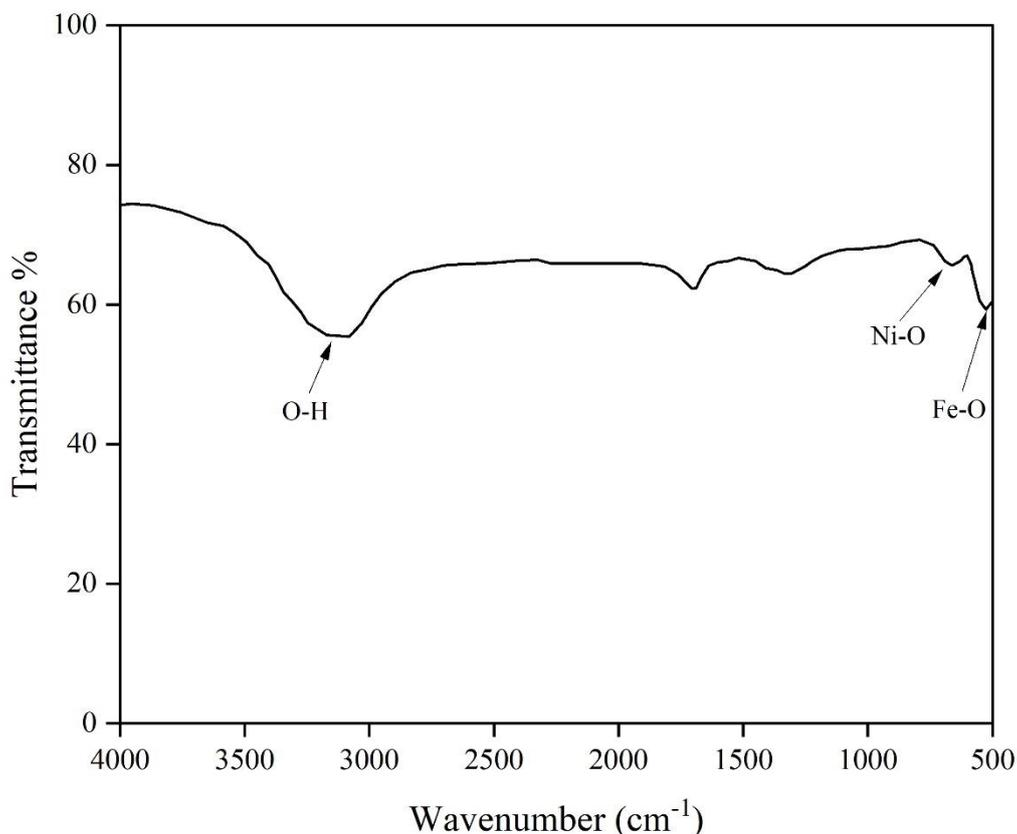
Fig. 2. FTIR spectrum of prepared  $\text{NiFe}_2\text{O}_4$  nanoparticles.
