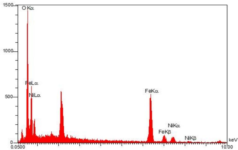
Fig. 4. EDS analysis of as-obtained NiFe<sub>2</sub>O<sub>4</sub> nanoparticles.
