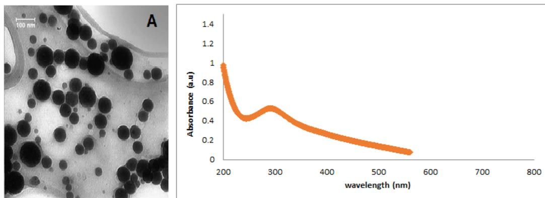
Fig. 3. A) TEM of spherical shaped colloidal synthesis of selenium nanoparticles in aqueous rosemary extract (CSSNANO). B) UV-visible absorption spectrum of the CSSNANO suspension
