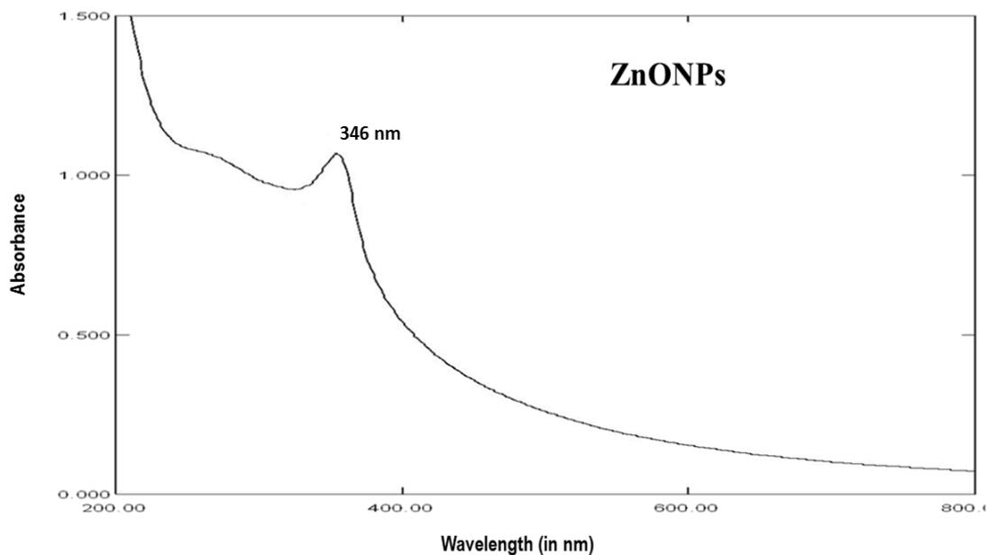
Fig. 1. UV-Vis spectra analysis of ZnONPs
