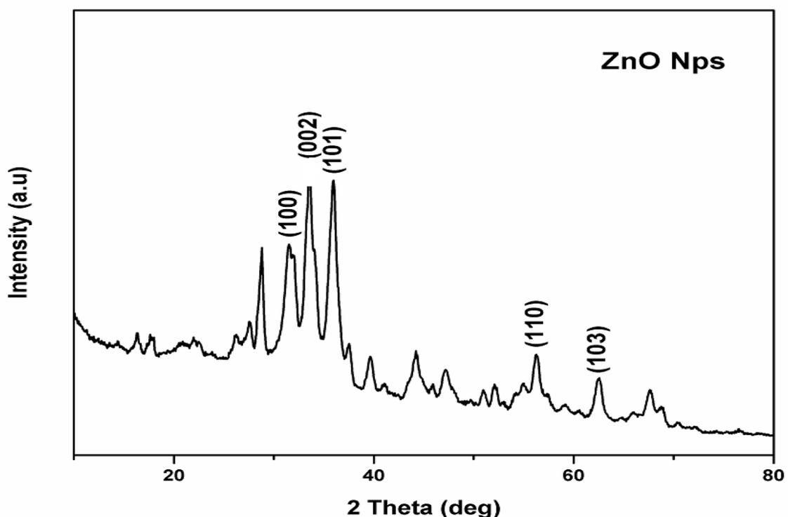
Fig. 4. PXRD analysis of ZnONPs
