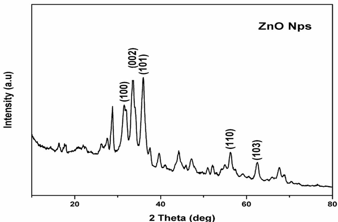
Fig. 4. PXRD analysis of ZnONPs
