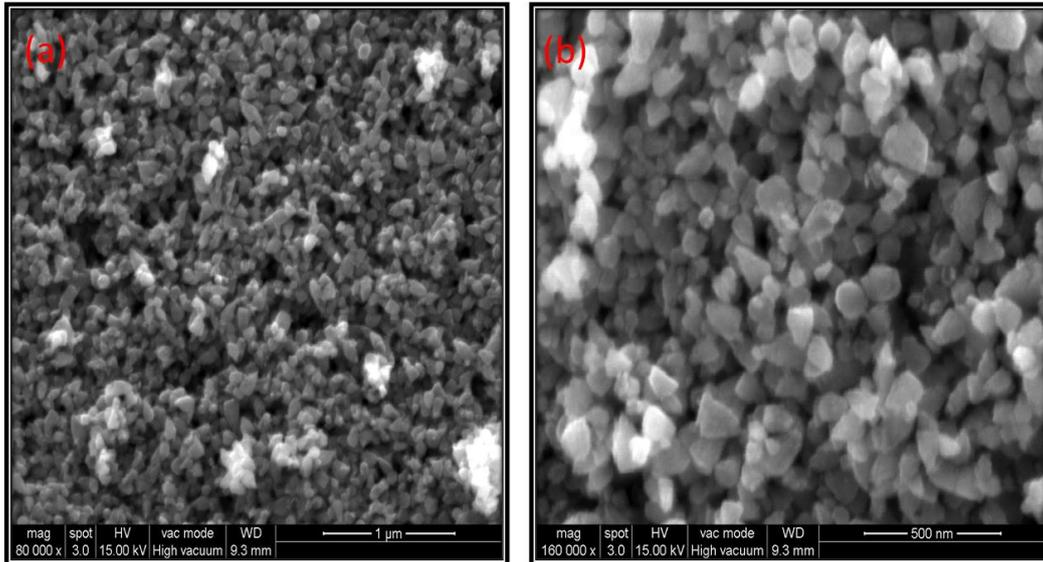
Fig. 2. Low (a) and High (b) magnification FESEM images of ZnONPs
