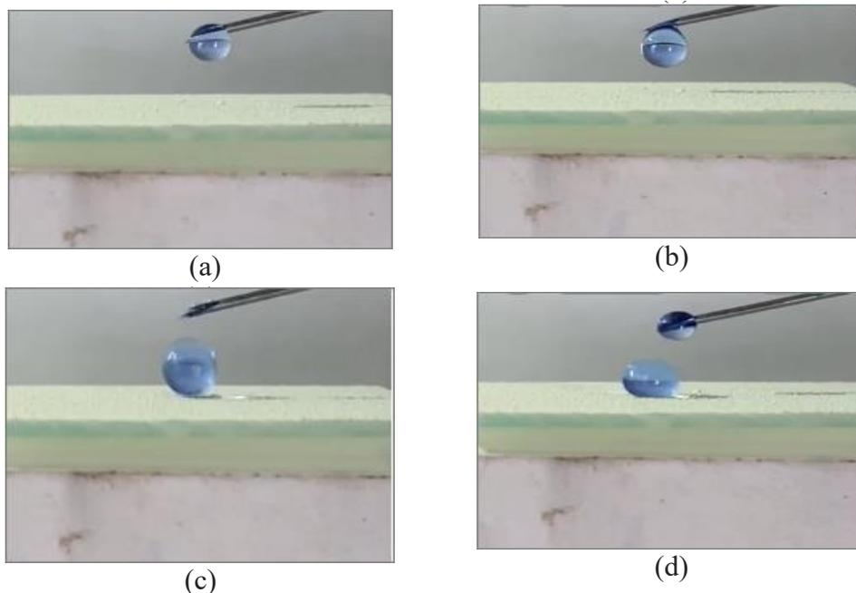
Fig. 2. The stages of a drop of water falling on the surface of the hydrophobic nanocomposite.
