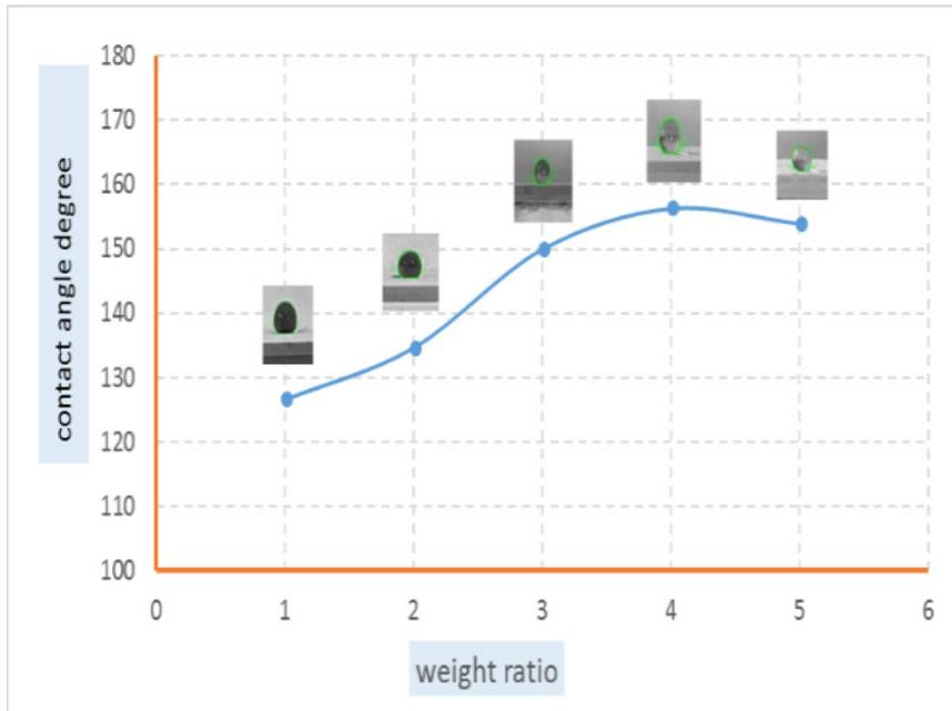
Fig. 4. The relation shape between  $\text{TiO}_2$  weight ratio and WCA.
