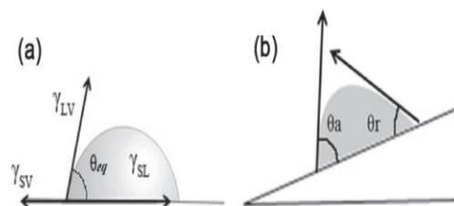
Fig. 1. Schematic illustration of (a) contact angle  $\theta$  on the flat solid surface and (b) a stable droplet on the tilted surface owing to the contact angle hysteresis, advancing angle  $\theta_a$  and receding angle  $\theta_r$  [18].
