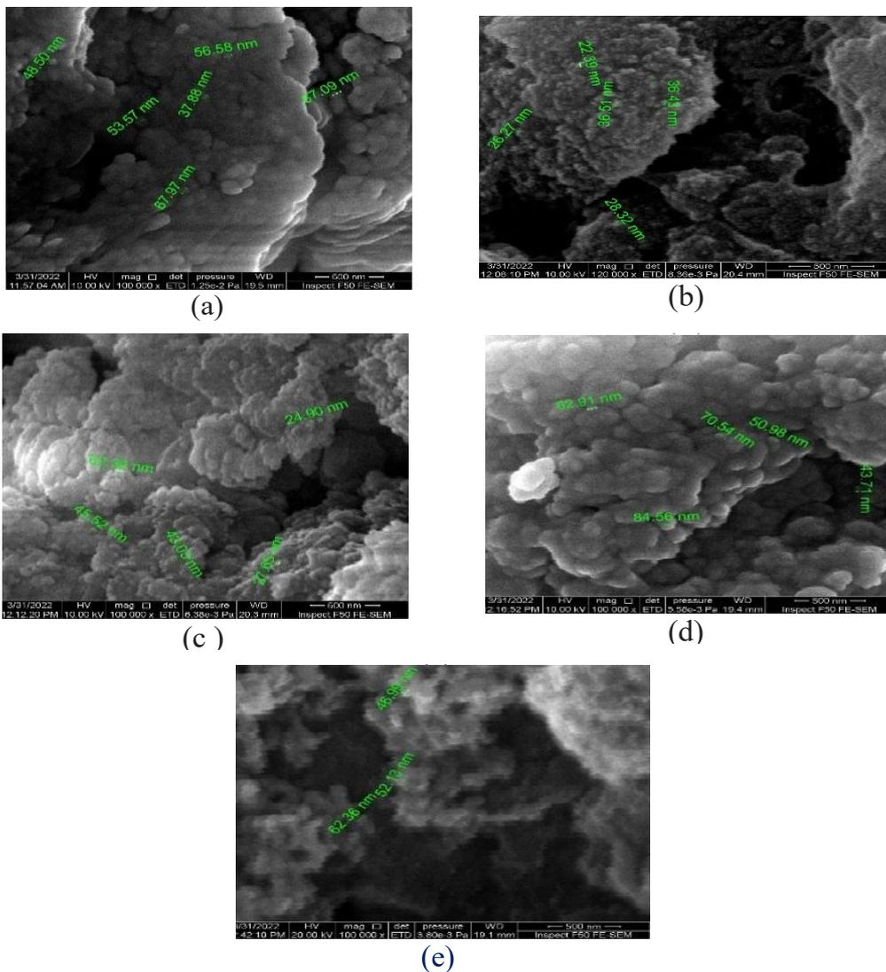
Fig. 3. FESEM images of films with (0, 10:1, 10:2, 10:3, 10:4) of  $(\text{SiO}_2:\text{TiO}_2)$  weight ratio.
