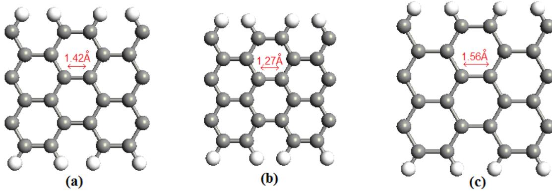
Fig. 1. (a) Graphene nanoribbon (GNR) in equilibrium. (b) GNR with comparative stress of %10 Pa. (c) GNR with tensile strain of %10 Pa.
