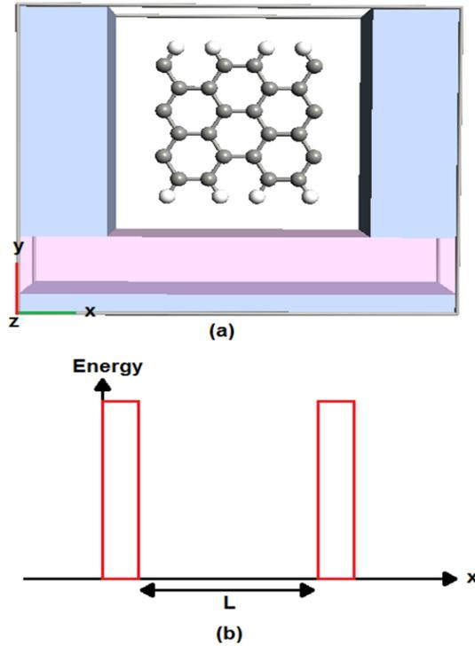
Fig. 2.(a) Graphene nanoribbon SET. (b) The energy profile vs channel length which indicates SET island as a quantum well.
