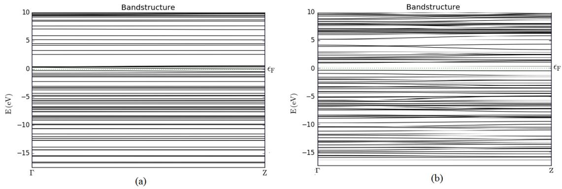
Fig. 6. The band structures of GNR with 24 carbon atoms (a) GNR band structure with compressive stress of 10 Pa on the island. (b) GNR band structure with tensile strain of 10 Pa on the island.
