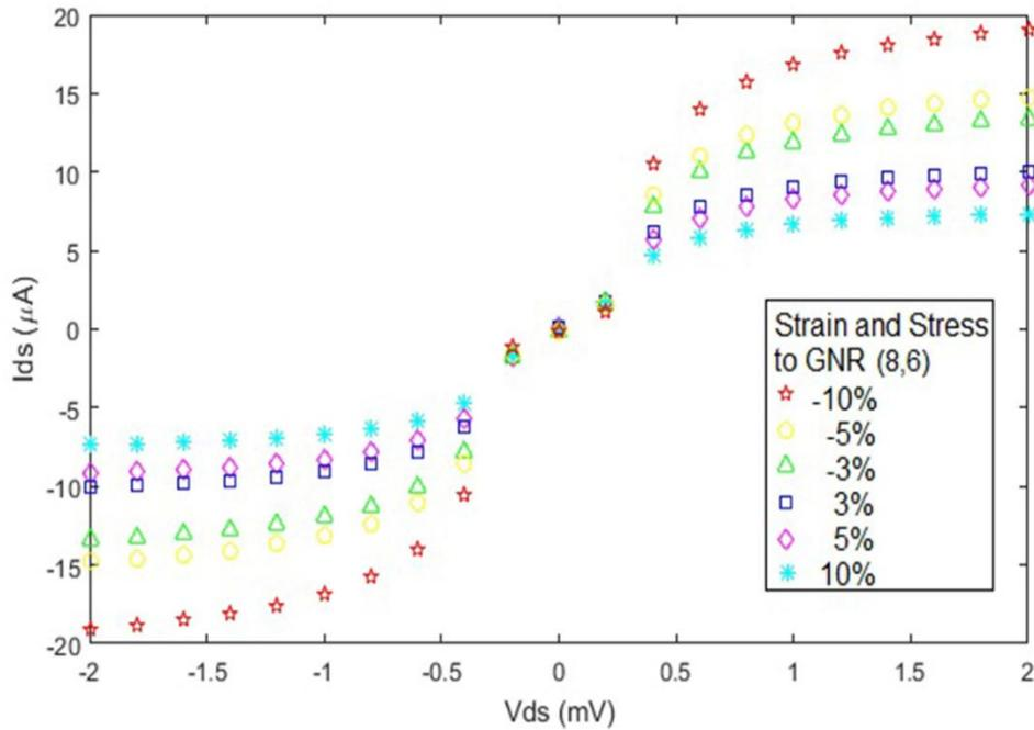
Fig. 3. The current vs. voltage diagram obtained from the proposed model for different value of compressive stresses and tensile strains on GNR island at 300 °K and  $V_{gs}$  is 1V.
