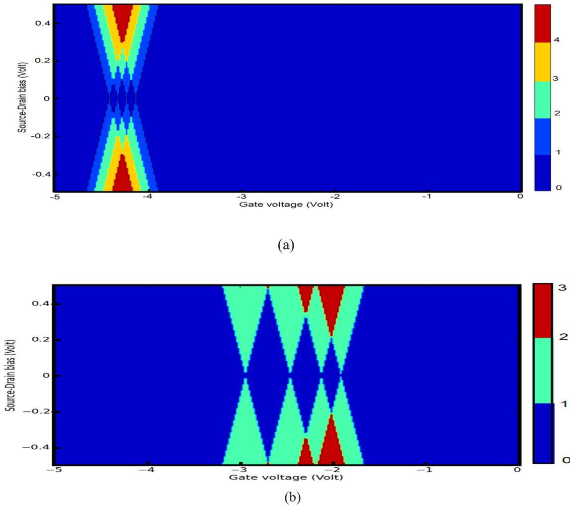
Fig. 7. The charge stability diagrams of GNR SET (a)  $V_g - V_{ds}$  with compressive stress of 10 Pa on the island. (b)  $V_g - V_{ds}$  with tensile strain of 10 Pa on the island. (The color bar on the right represents the corresponding charge states in the diagram).
