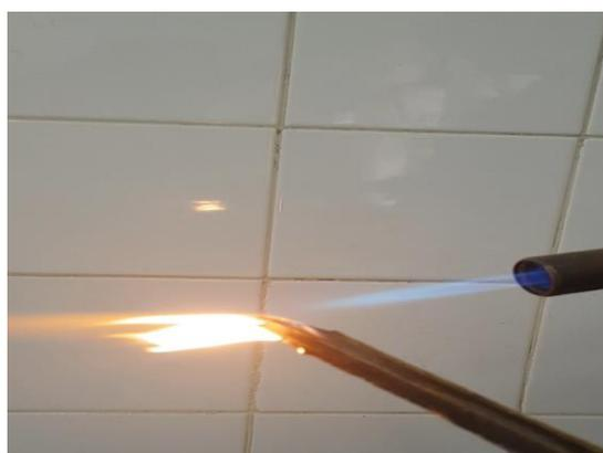
Fig. 6. UL-94 test of prepared nanocomposite
