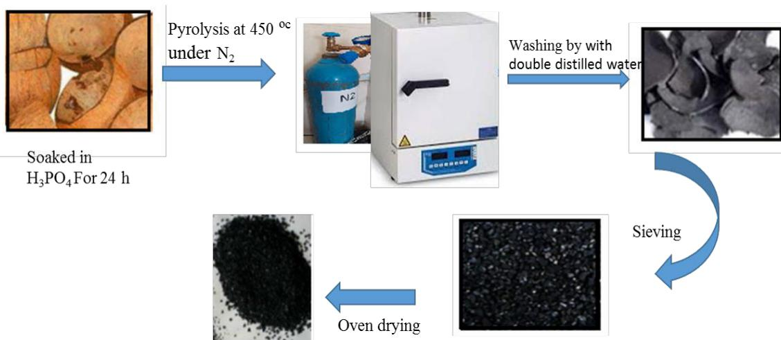
Fig.2. Schematic of activate carbon preparation from coconut shell
