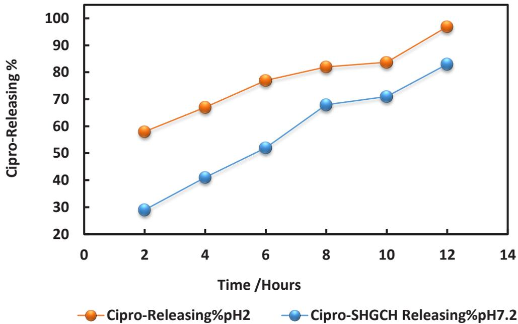
Fig. 7. The drug release amount of Cipro-SH-CH NPs at pH 2 and pH 7.2 at 37 °C at 340 nm using uv-vis spectrophotometry
