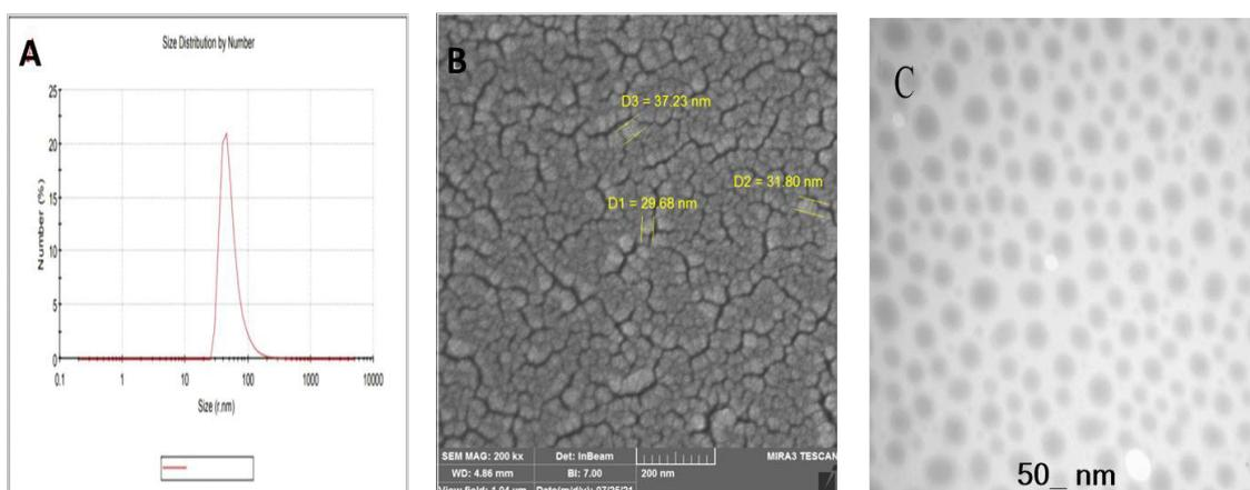
Fig. 4. (A) The average particle size distribution of Cipro loaded shellac-chitosan NPs using DLS instrument(B) The FESEM image of shellac – chitosan nanoparticles prepared by mixing 0.25% of glutamic-chitosan with 0.25% shellac (C) TEM image of Cipro-loaded SH-CH nanoparticles (prepared by mixing SH-CH 0.25 wt.% with Cipro 0.25 wt.%).
