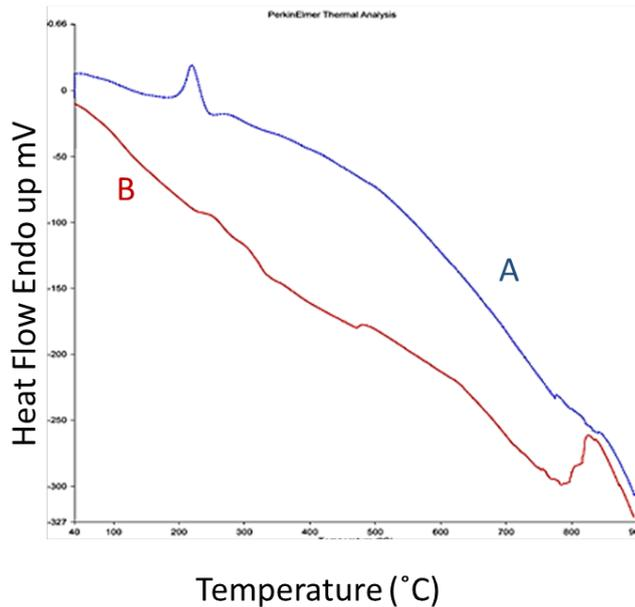
Fig. 6. DSC thermograms of (A) SH-CH NPs and (B) Cipro-loaded shellac-chitosan nanoparticles with CG 0.25 wt.%, SH 0.25 wt.%, and Cipro 0.25 wt.% in a 1:1:1 ratio.
