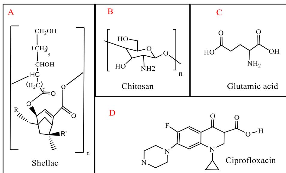
Fig. 1. The chemical structure of; A: Shellac, B: chitosan, C: Glutamic acid, and D: Ciprofloxacin drug
