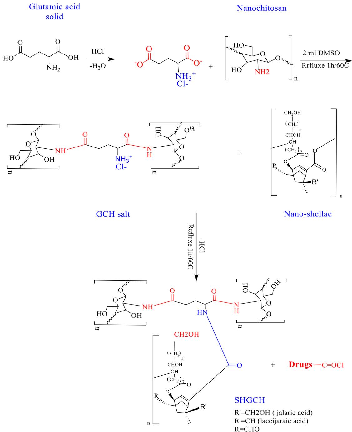
Fig. 3. A Schematic represents the preparation steps of Cipro loaded SH-CH NPs
