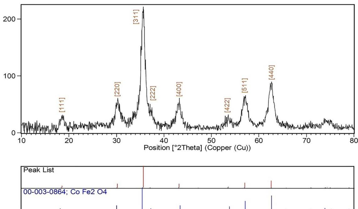
Fig. 1. The XRD graph of CoFe<sub>2</sub>O<sub>4</sub> nanoparticles
