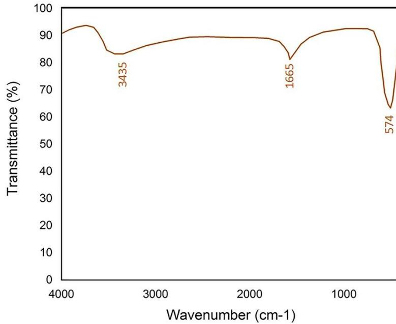
Fig. 2. FT-IR spectrum of CoFe<sub>2</sub>O<sub>4</sub> nanoparticles
