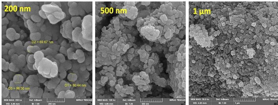
Fig. 5. FE-SEM images of as-prepared  $\text{CoFe}_2\text{O}_4$  nanoparticles
