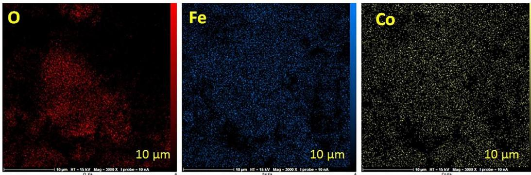
Fig. 3. The elemental mapping of CoFe<sub>2</sub>O<sub>4</sub> nanoparticles
