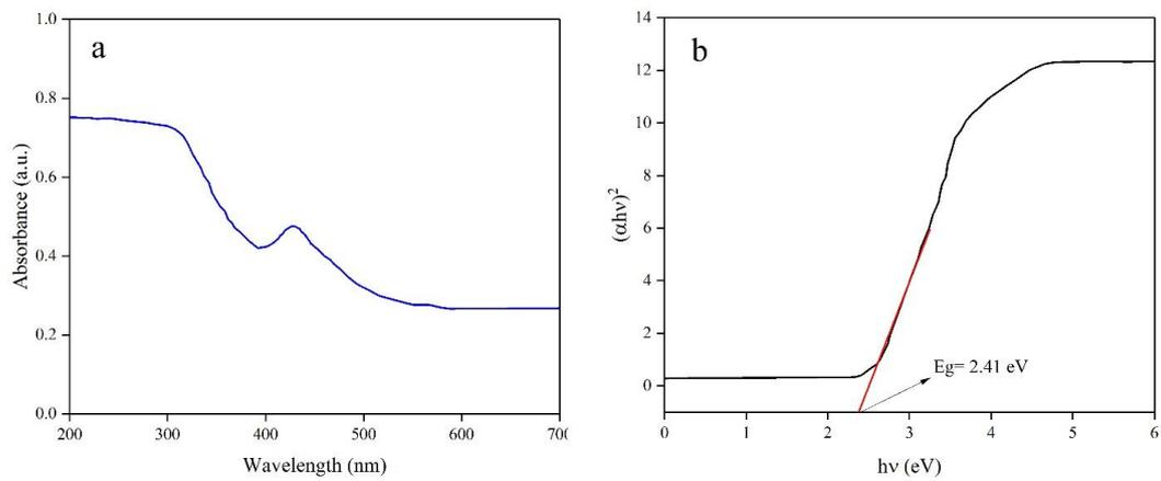
Fig. 6. a) UV-Vis analysis b) optical band gap of prepared  $\text{CoFe}_2\text{O}_4$  nanoparticles
