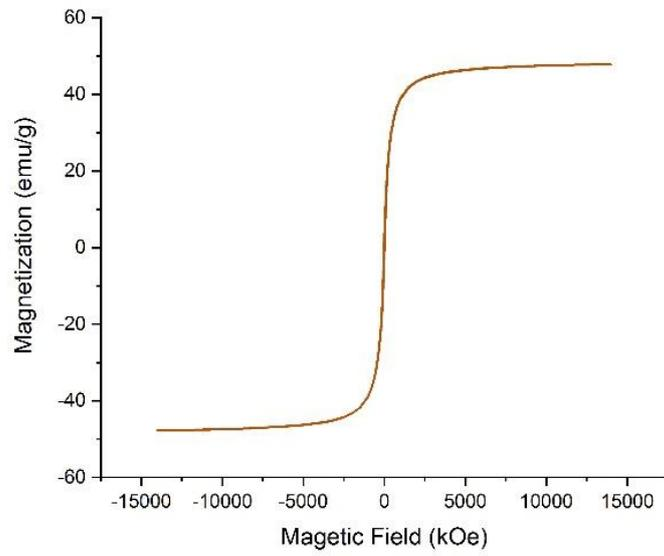
Fig. 4. VSM curve of  $\text{CoFe}_2\text{O}_4$  nanoparticles
