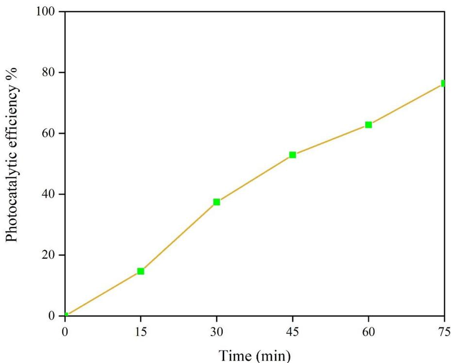
Fig. 7. Photodegradation of Reactive Violet 5 under visible light after 75 min.
