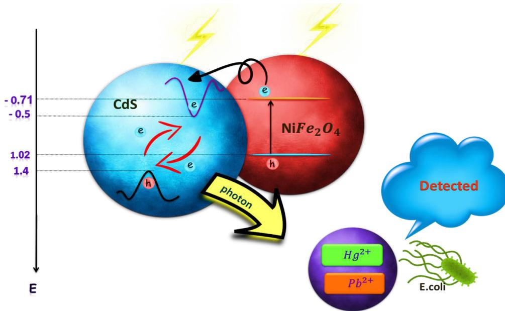
Fig. 13. Schematic of the photoluminescence mechanism of  $\text{NiFe}_2\text{O}_4$ -CdS nanostructure
