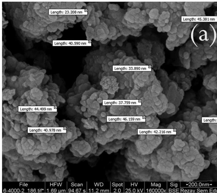
Fig. 4. SEM image of NiFe<sub>2</sub>O<sub>4</sub> nanoparticles product by microwave method
