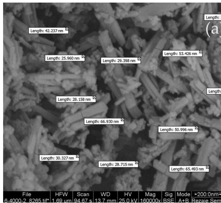
Fig. 6. SEM image of CdS nanoparticles synthesized applying CTAB
