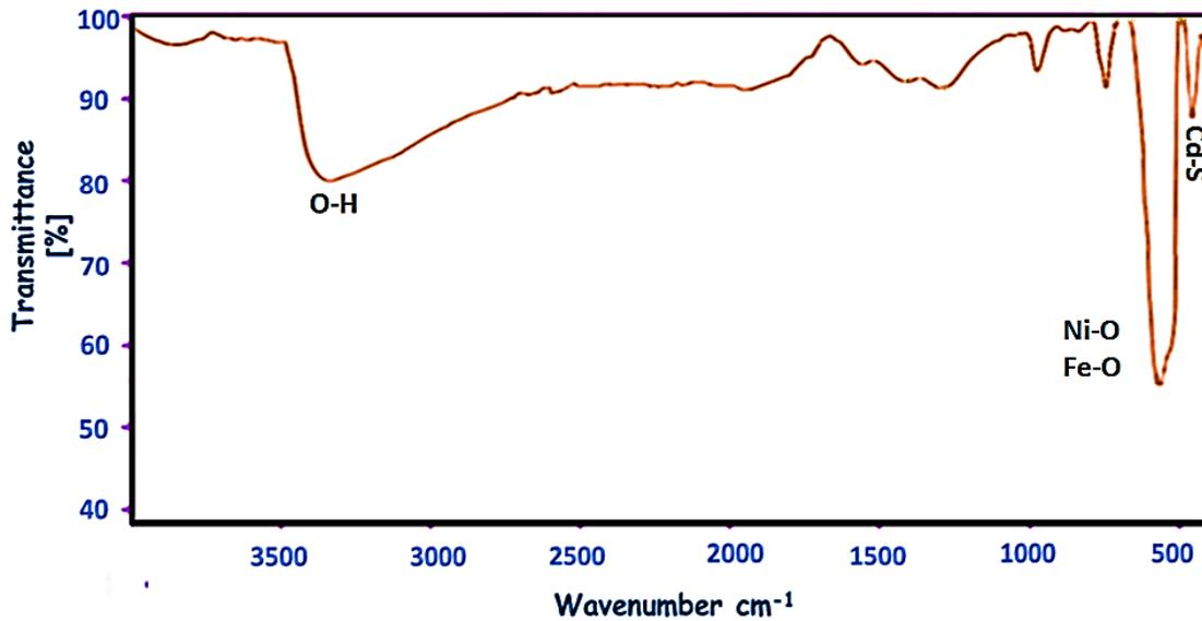
Fig. 9. FT-IR spectrum of NiFe<sub>2</sub>O<sub>4</sub>-CdS nanocomposite
