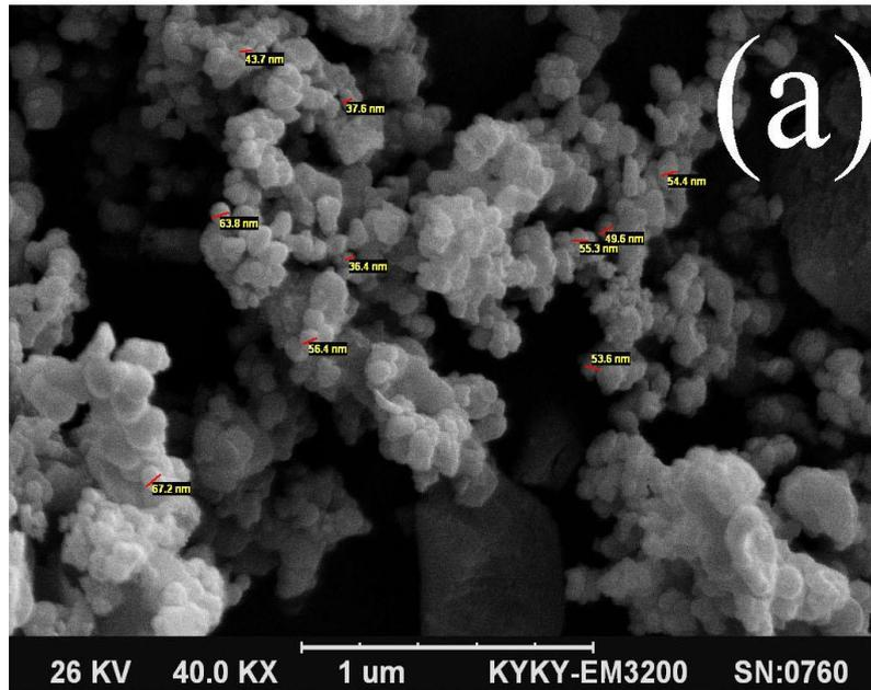
Fig. 5. SEM image of CdS nanoparticles without using any surfactants
