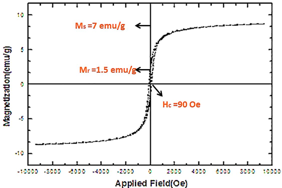
Fig.11. VSM graph of  $\text{NiFe}_2\text{O}_4$ -CdS nanocomposite
