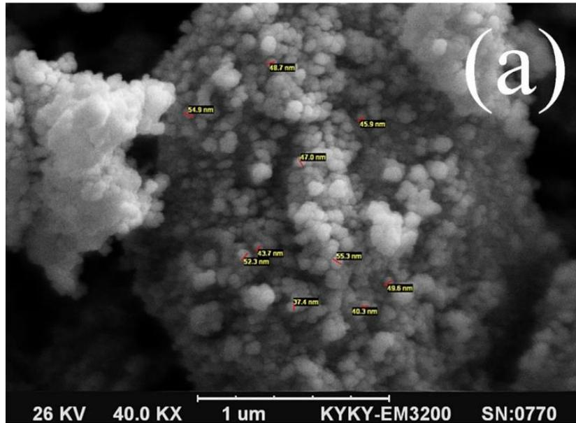
Fig. 3. SEM image of NiFe<sub>2</sub>O<sub>4</sub> nanoparticles product by hydrothermal method
