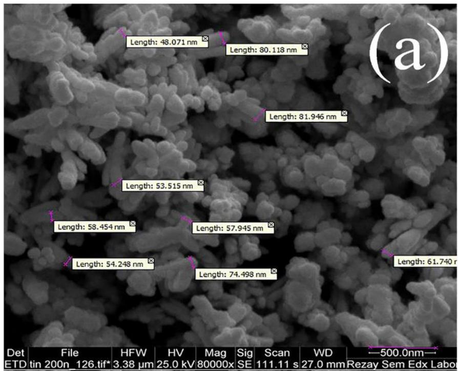
Fig. 8. SEM image of NiFe<sub>2</sub>O<sub>4</sub>-CdS nanocomposite
