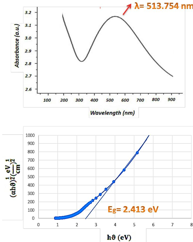
Fig. 12. UV-Vis absorption and band gap estimation of CdS nanoparticles
