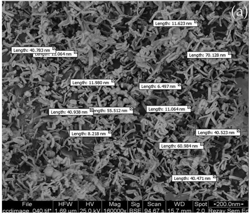
Fig. 7. SEM image of CdS nanoparticles synthesized in the presence of grapefruit extract
