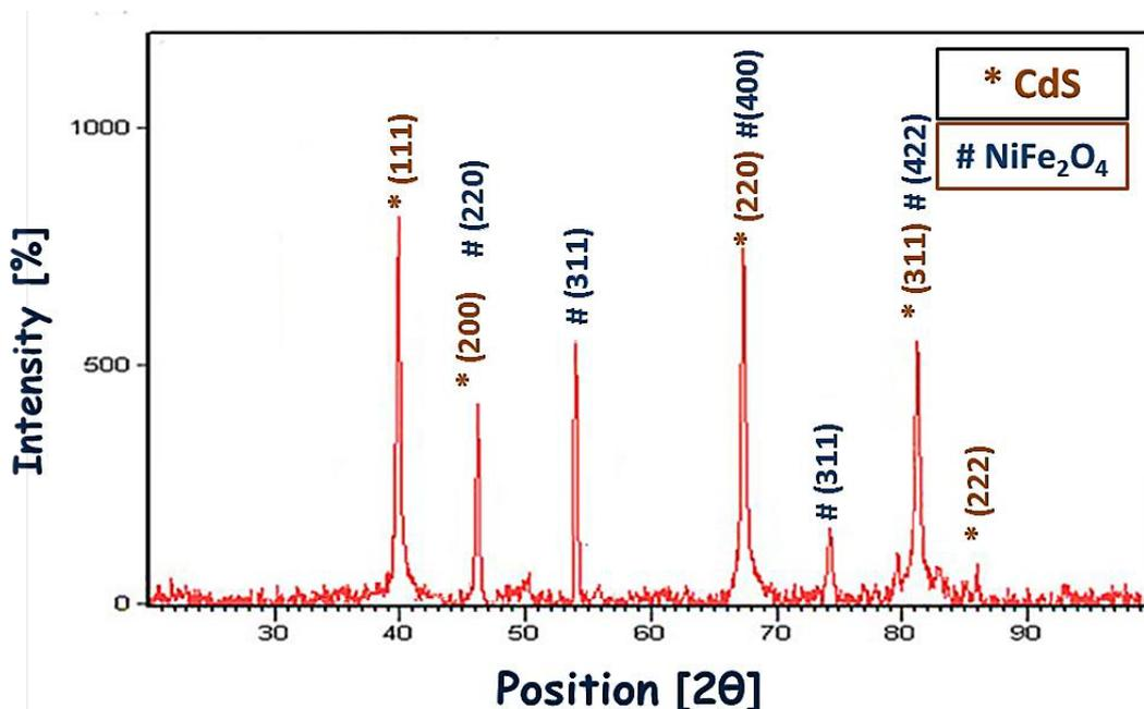
Fig. 2. XRD pattern of a NiFe<sub>2</sub>O<sub>4</sub> - CdS nanocomposite
