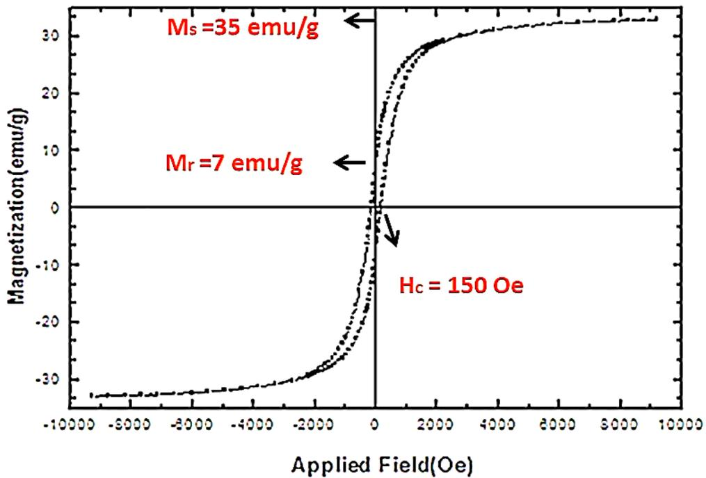
Fig. 10. VSM graph of NiFe<sub>2</sub>O<sub>4</sub> nanoparticles
