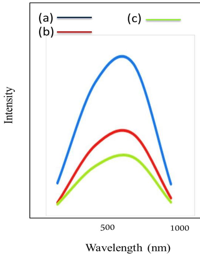
Fig. 14. (a) PL of nanocomposite by adding (b) Pb(II) (c) Hg (II)
