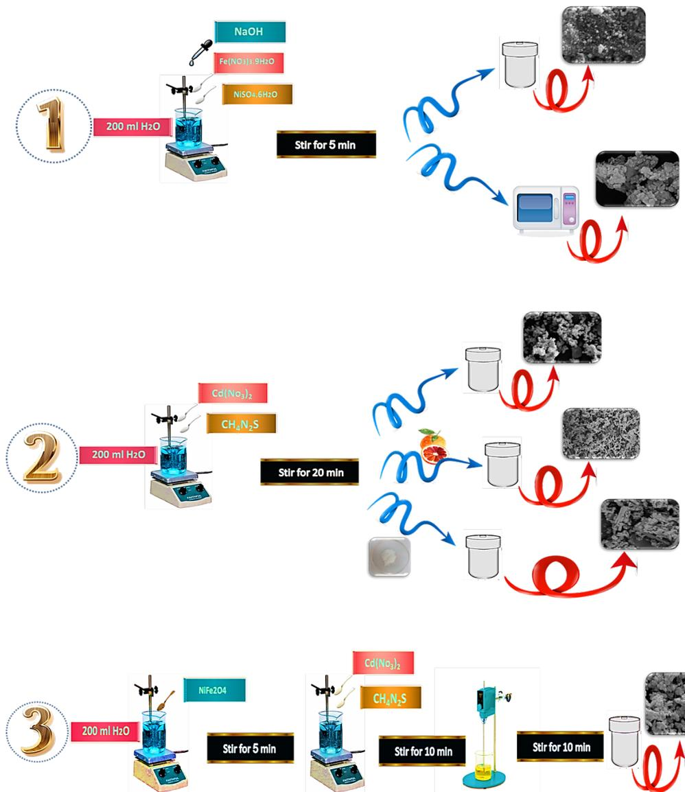
Fig. 1. Schematic of synthesis of  $\text{NiFe}_2\text{O}_4$ , CdS and  $\text{NiFe}_2\text{O}_4$ -CdS
