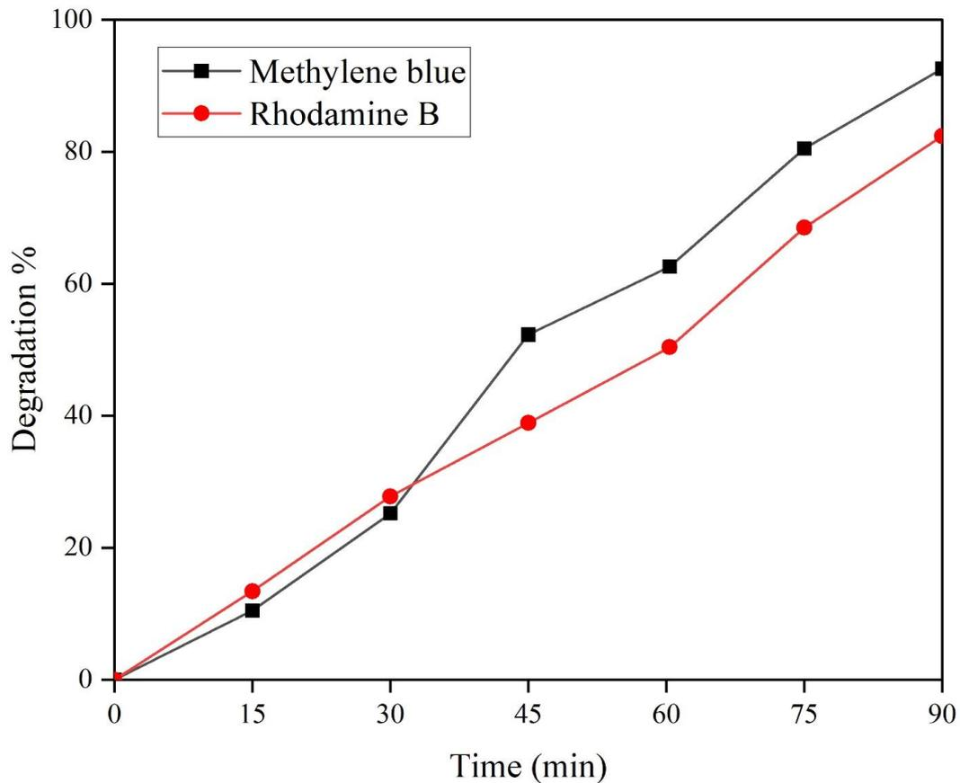
Fig. 6. Photocatalytic activity of ZnMoO<sub>4</sub> nanoparticles for removal of methylene blue and rhodamine B.
