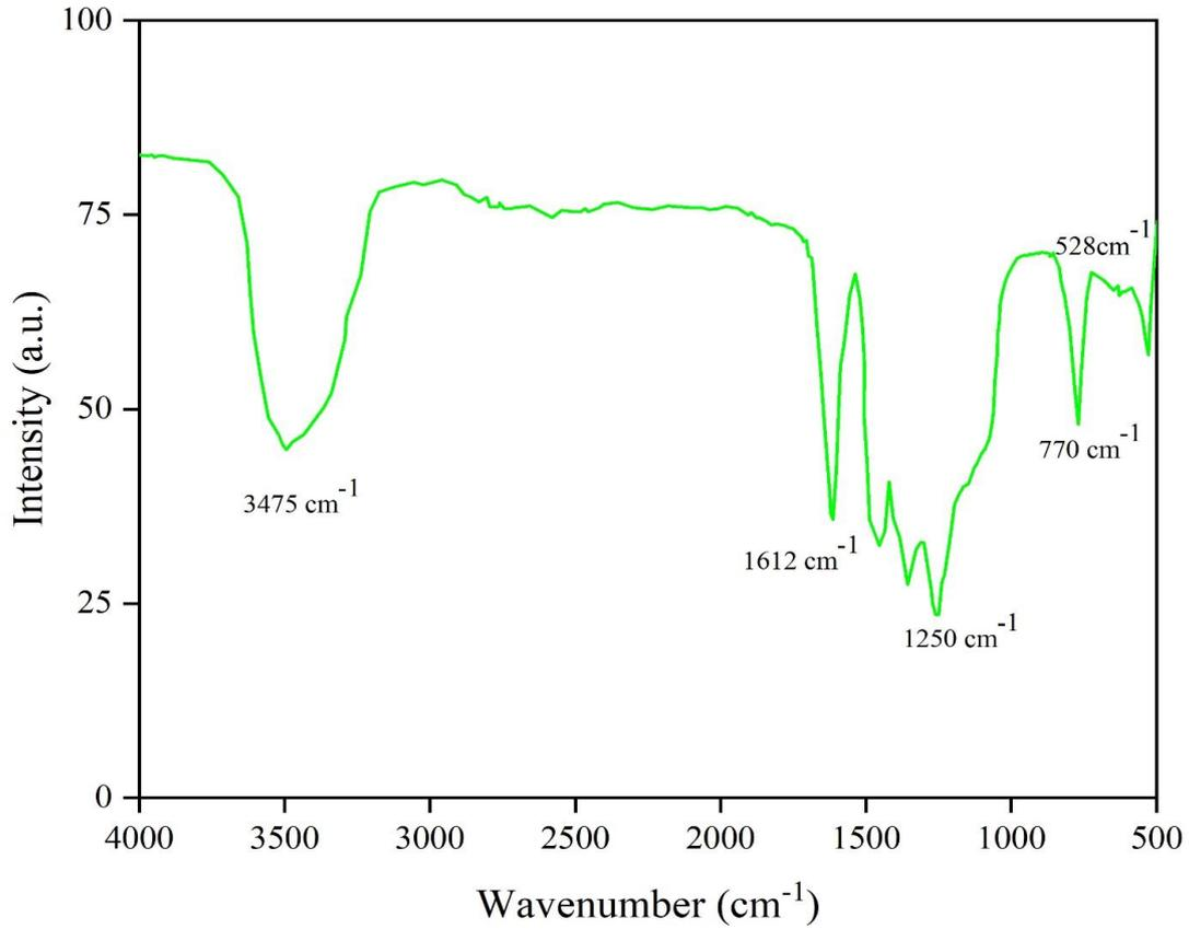
Fig. 2. FTIR spectrum of prepared ZnMoO<sub>4</sub> nanoparticles.
