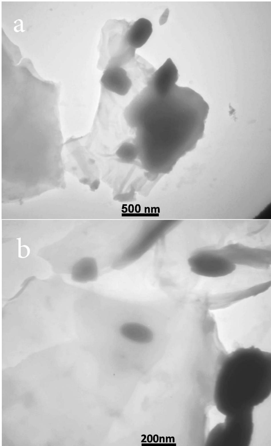
Fig. 4. The TEM images of synthesized ZnMoO<sub>4</sub> nanoparticles at different magnifications.
