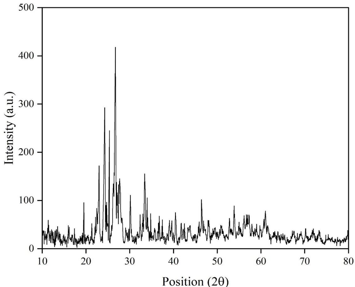
Fig. 1. XRD pattern of prepared ZnMoO<sub>4</sub> nanoparticles.
