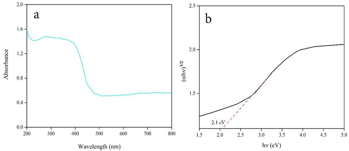
Fig. 5. . a) UV-vis diffuse reflectance spectra and b) band gap energy of prepared ZnMoO<sub>4</sub> nanoparticles.
