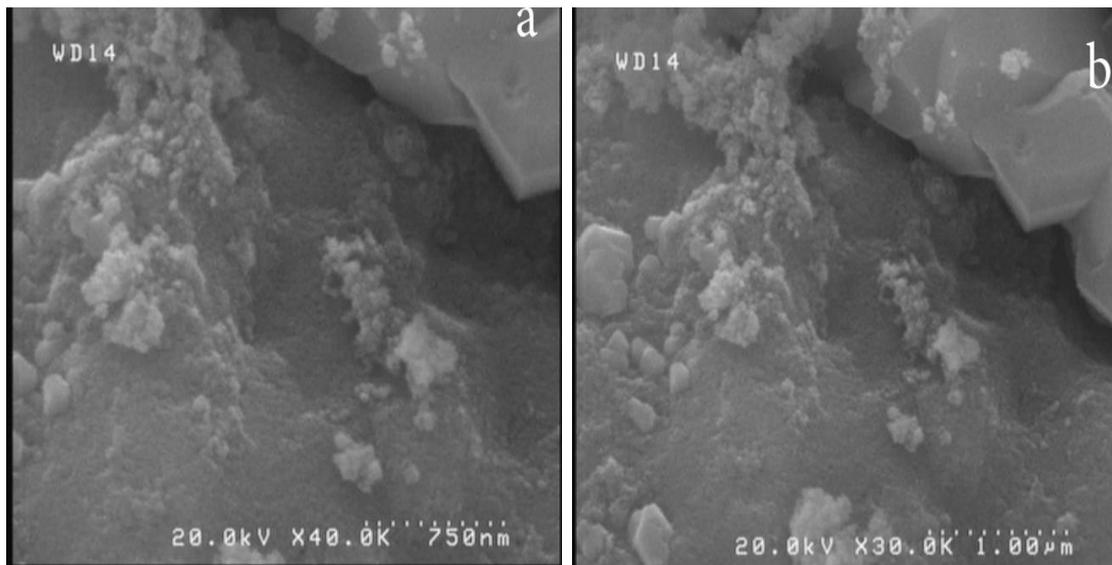
Fig. 3. The SEM images of synthesized ZnMoO<sub>4</sub> nanoparticles at different magnifications.
