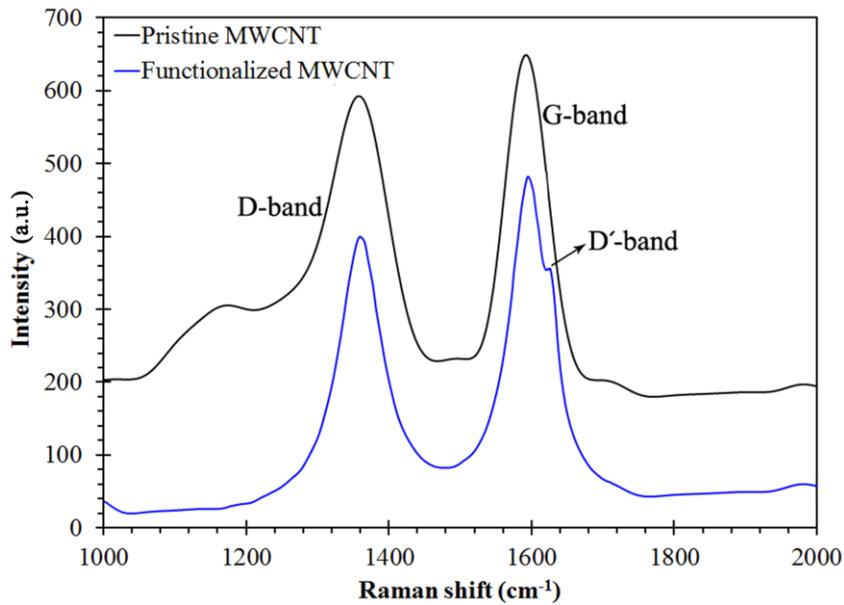
Fig. 2. Raman spectra of pristine and functionalized multi-walled carbon nanotubes (MWCNT-COOH).
