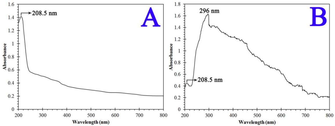
Fig. 4. UV-Vis spectra of A: pristine and B: functionalized multi-walled carbon nanotubes (MWCNT-COOH).
