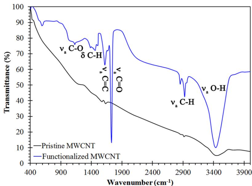
Fig. 1. FT-IR spectra of pristine and functionalized multi-walled carbon nanotubes (MWCNT-COOH).
