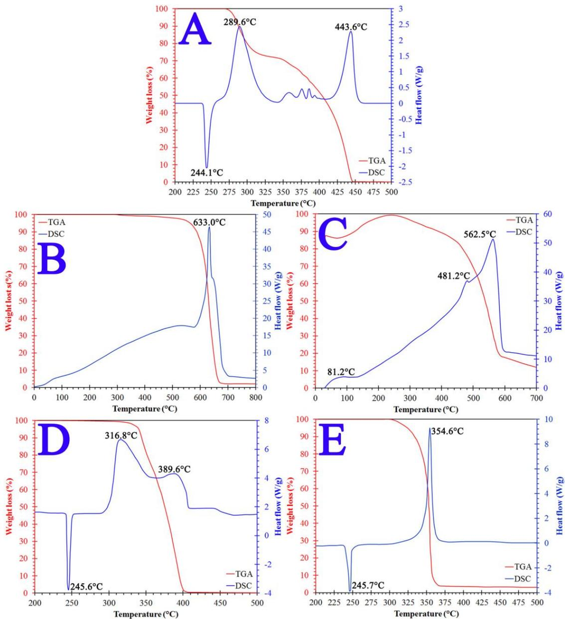
Fig. 7. TGA and DSC curves of A: AP, B: pristine MWCNTs, C: functionalized multi-walled carbon nanotubes (MWCNT-COOH) D: AP/MWCNTs, and E: AP/MWCNT-COOH composite at rate of 10°C/min.
