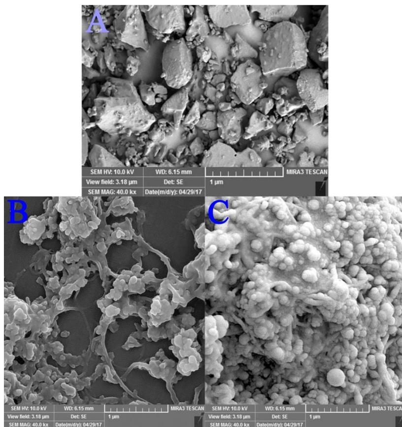
Fig. 6. FE-SEM images of A: ammonium perchlorate (AP) and its composite with B: pristine and C: functionalized multi-walled carbon nanotubes.
