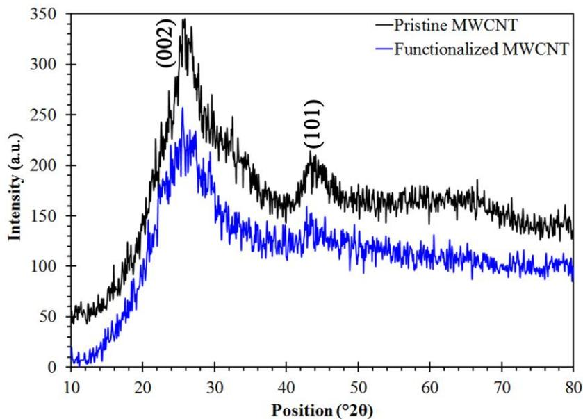
Fig. 3. XRD patterns of pristine and functionalized multi-walled carbon nanotubes (MWCNT-COOH).
