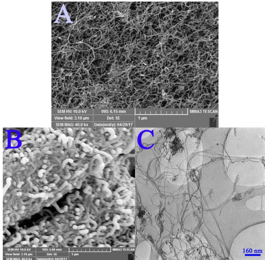
Fig. 5. A: FE-SEM image of pristine MWCNTs, B: FE-SEM and C: TEM images of functionalized multi-walled carbon nanotubes (MWCNT-COOH).
