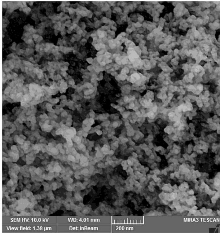
Fig. 4. SEM image of copper nanoparticles
