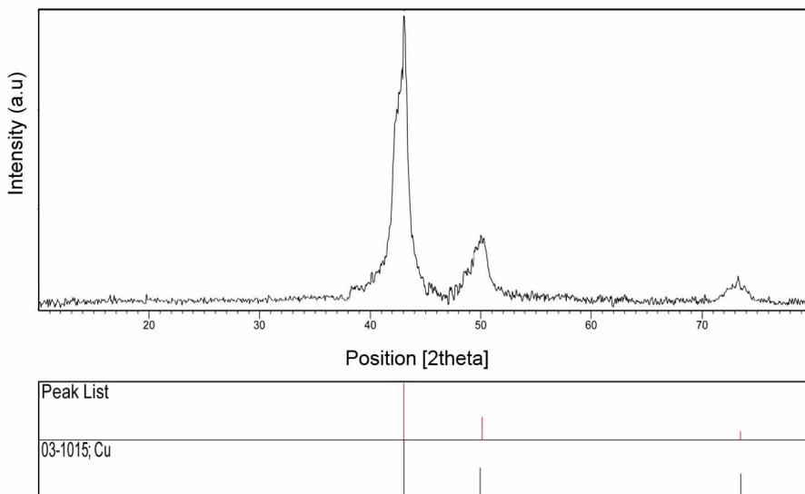
Fig. 5. XRD pattern of copper nanoparticles
