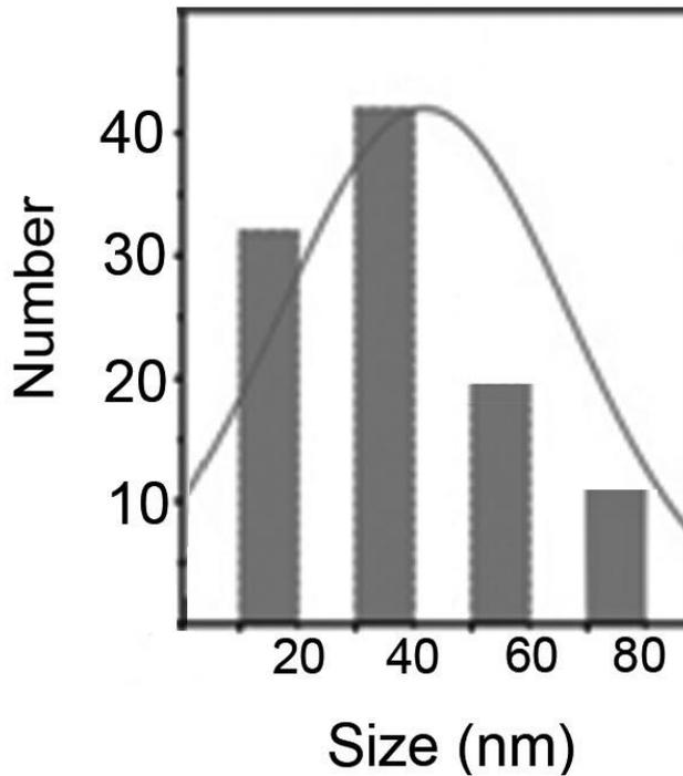
Fig. 6. Particle size distribution profile of copper nanoparticles
