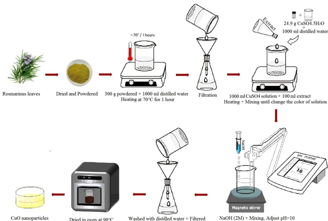
Fig. 1. Schematic presentation of copper nanoparticles synthesis using Rosemary extract
