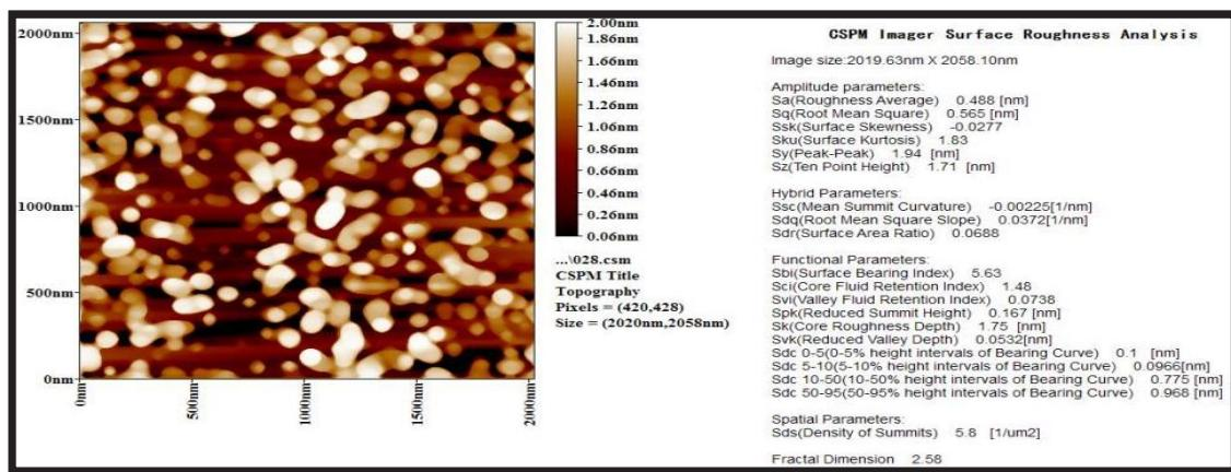
Fig. 2. Atomic force microscopy images of the Xerogel/MTX nanocomposite A two-dimensional image showing all the details of the molecules.
