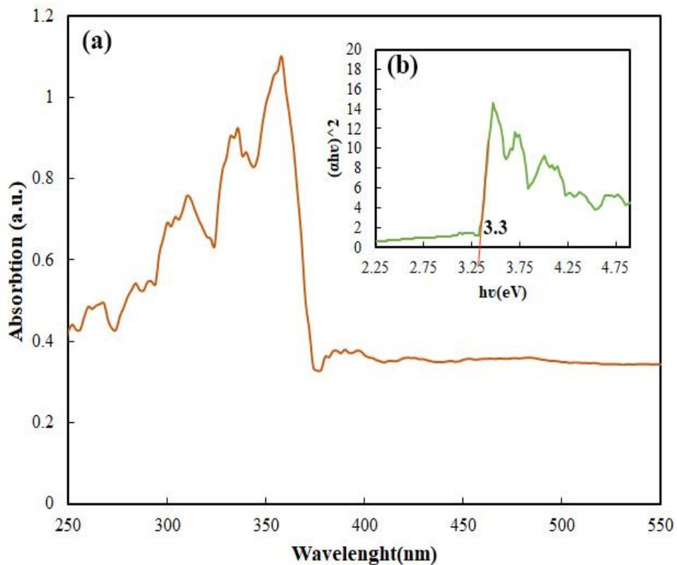
Fig. 6. (a) UV-Vis diffuse reflectance spectrum (DRS) of the MnCo<sub>2</sub>O<sub>4</sub>/Co<sub>3</sub>O<sub>4</sub> Nanocomposites prepared at 10 min in 900 W, and (b) the plot of  $(\alpha h\nu)^2$  against  $h\nu$  to determine the band gaps.
