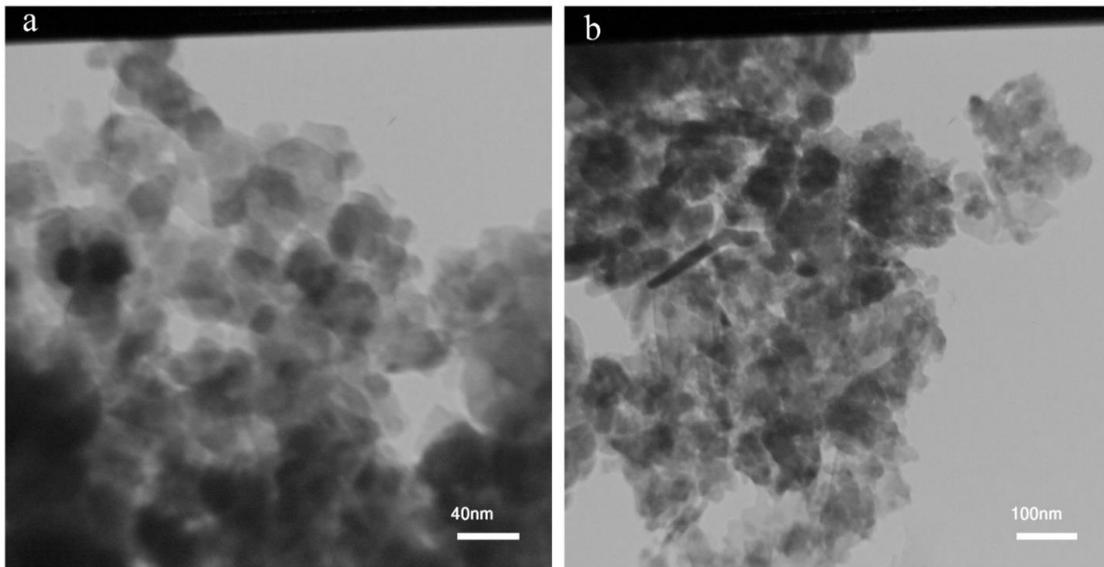
Fig. 5. TEM images of the MnCo<sub>2</sub>O<sub>4</sub>/Co<sub>3</sub>O<sub>4</sub> Nanocomposites prepared at 10 min in 900 W
