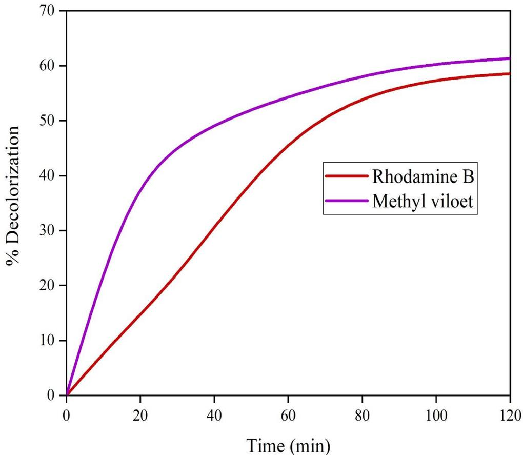
Fig. 7. Photocatalytic activity of MnCo<sub>2</sub>O<sub>4</sub>/ Co<sub>3</sub>O<sub>4</sub> nanocomposites against the rhodamine B and methyl violet
