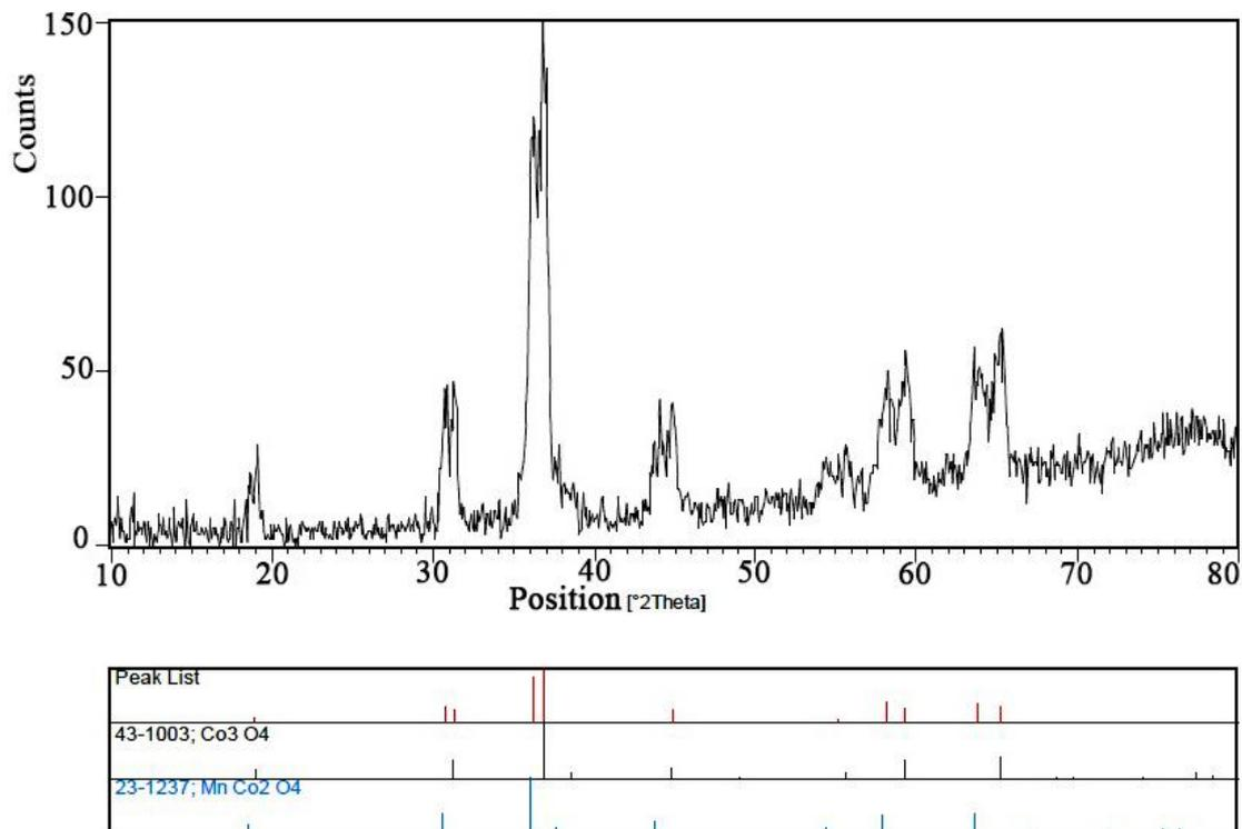
Fig. 1. XRD pattern of MnCo<sub>2</sub>O<sub>4</sub>/Co<sub>3</sub>O<sub>4</sub> Nanocomposites prepared at 10 min in 900 W.
