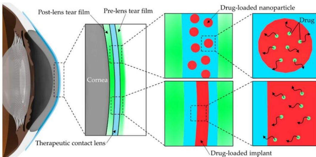
Fig. 5. Schematic of drug release onto the ocular surface from drug-eluting therapeutic contact lens. Typical polymeric vehicles for therapeutic contact lenses include drug-loaded polymeric nanoparticles and drug-loaded polymeric implants inside contact lenses.
