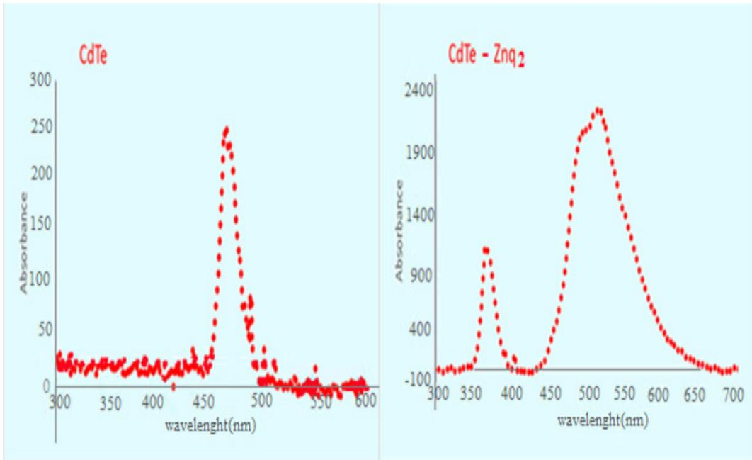
Fig. 13. PL comparison of the CdTe quantum dot spectrum and CdTe-Znq<sub>2</sub>
