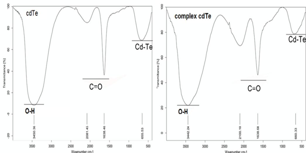
Fig. 15. FT-IR spectra of the CdTe quantum dot and its complex
