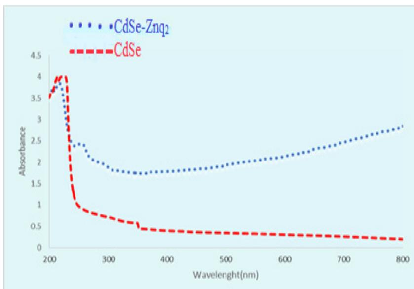
Fig. 9. Comparison of the absorption spectra of CdSe and CdSe-Znq<sub>2</sub>
