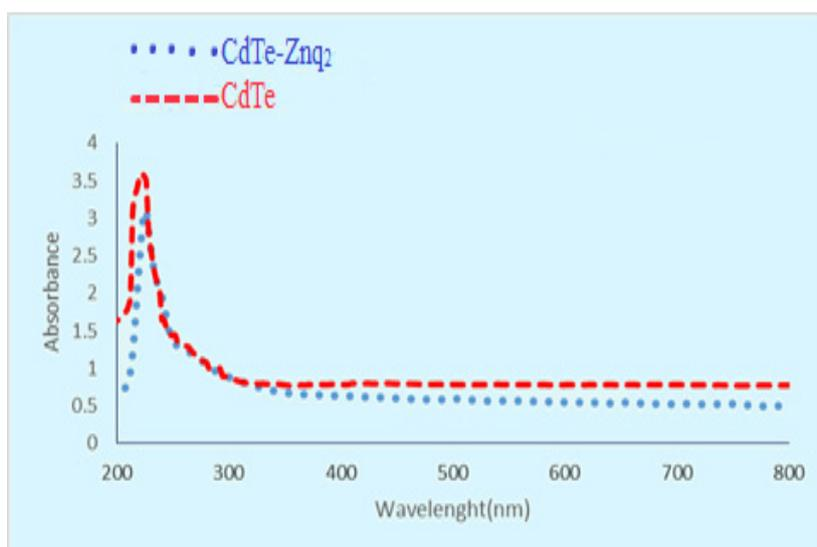
Fig. 10. Comparison of the absorption spectra of CdTe and CdTe-Znq<sub>2</sub>
