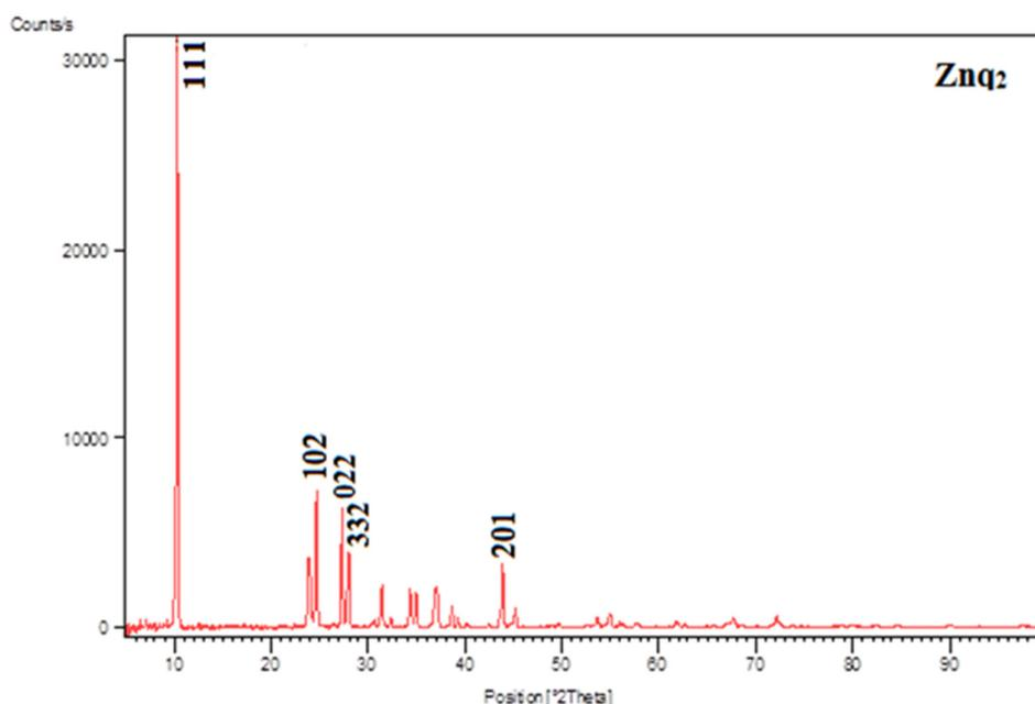
Fig. 1. XRD pattern of Znq<sub>2</sub>
