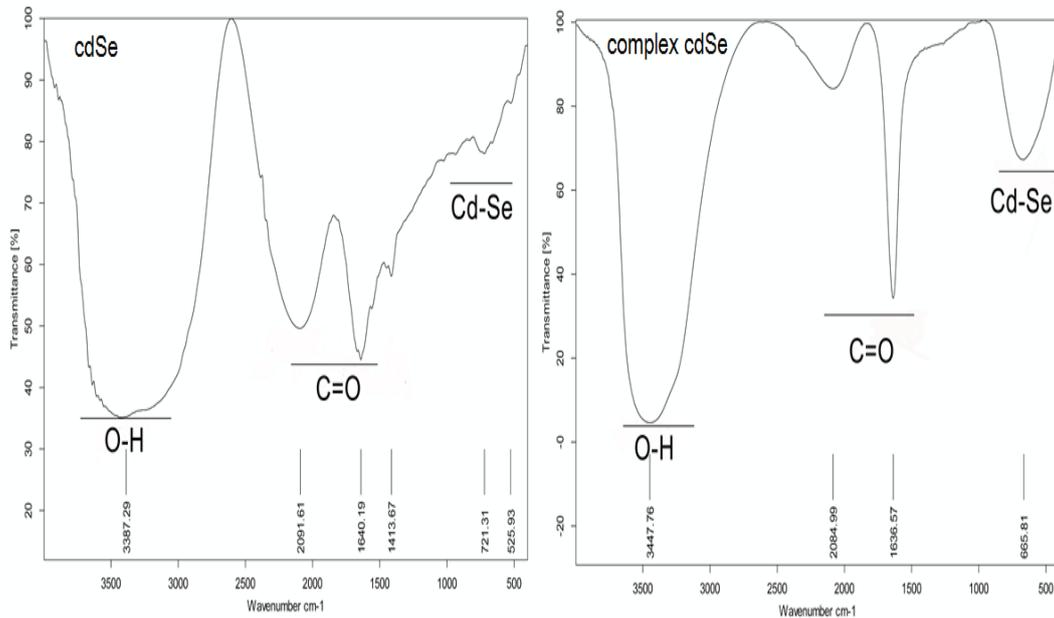
Fig. 14. FT-IR spectra of the CdSe quantum dot and its complex
