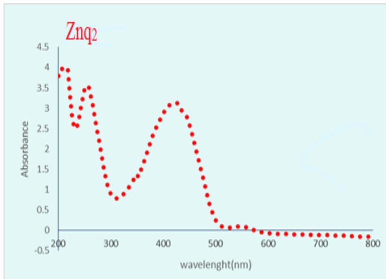
Fig. 8. Znq<sub>2</sub> absorption spectrum
