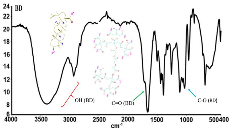
Fig 5. FTIR spectrum of BD, confirming physically BA loading into dendrimer nanocarrier.
