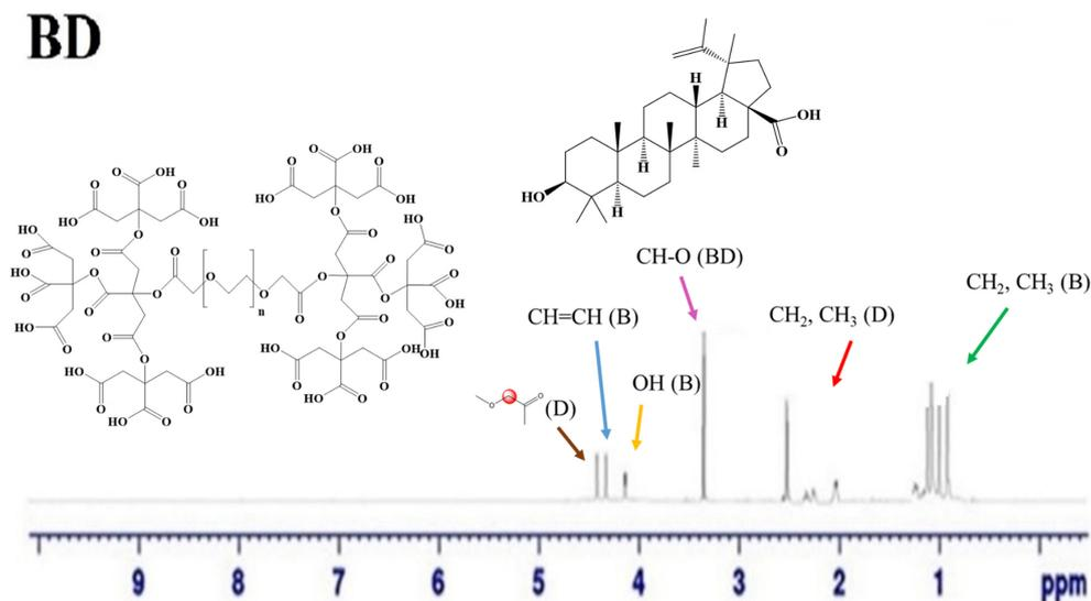
Fig 6. <sup>1</sup>H NMR spectrum of betulinic acid dendrimer (BD), indicating that BA was loaded into dendrimer nanocarrier.
