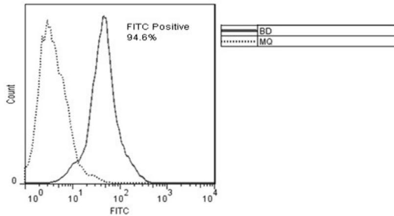
Fig 7. Cellular uptake of betulinic acid dendrimer (BD) into macrophages, measured by flow cytometry method which was equal to 95%.
