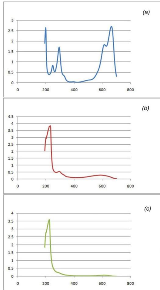
Fig. 9. UV-Vis spectra of degradation of methylene blue a) 0 min, b) 30 min in the presence of ZnS nanoparticles, c) 30 min in the presence of nano composite
