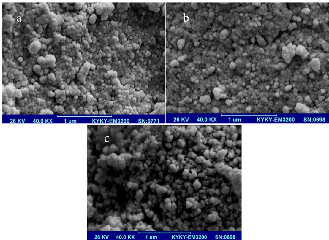
Fig. 4. SEM images of a)  $\text{Fe}_2\text{O}_3$  with NaOH deposition factor b)  $\text{Fe}_3\text{O}_4$  with  $\text{C}_6\text{H}_{10}\text{O}_5$  deposition factor c) iron oxide-zinc sulphide nano-composite
