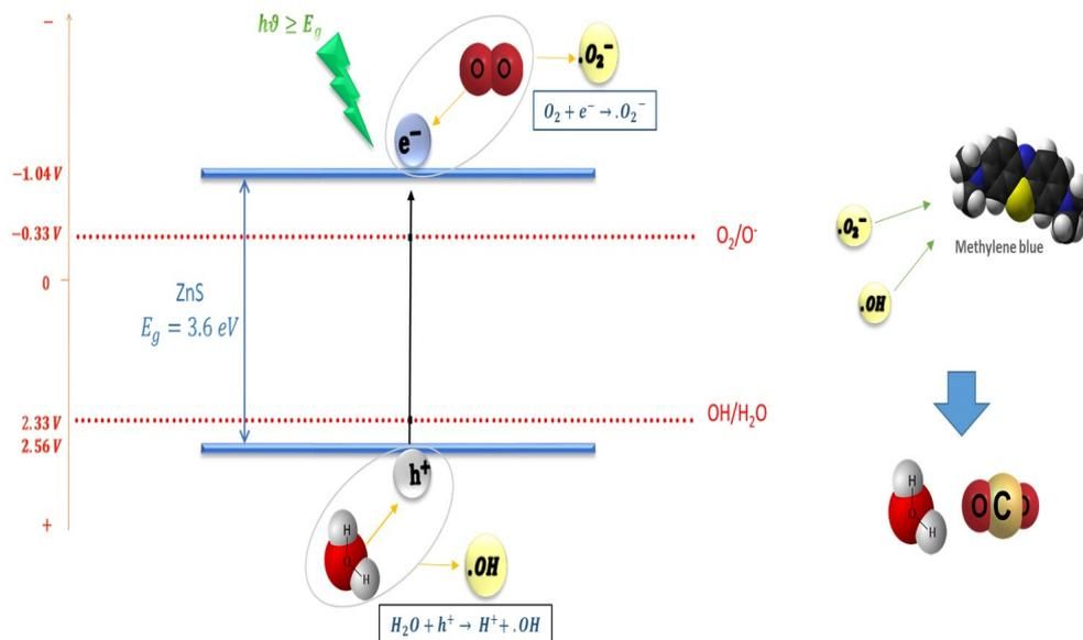
Fig. 10. Schematic of the mechanism of photocatalytic properties of iron oxide/zinc sulphide nano-composite under UV light
