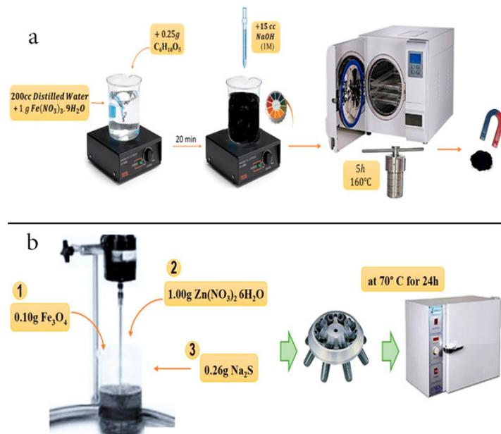
Fig. 1. a) Schematic of  $\text{Fe}_3\text{O}_4$  nanoparticles preparation b) Schematic of nano-composite preparation
