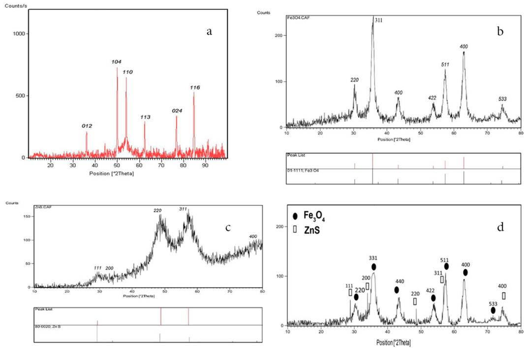
Fig. 2. XRD patterns of a)  $Fe_2O_3$  nanoparticles b)  $Fe_3O_4$  nanoparticles c) ZnS nanoparticles d) iron oxide-zinc sulphide nano-composite
