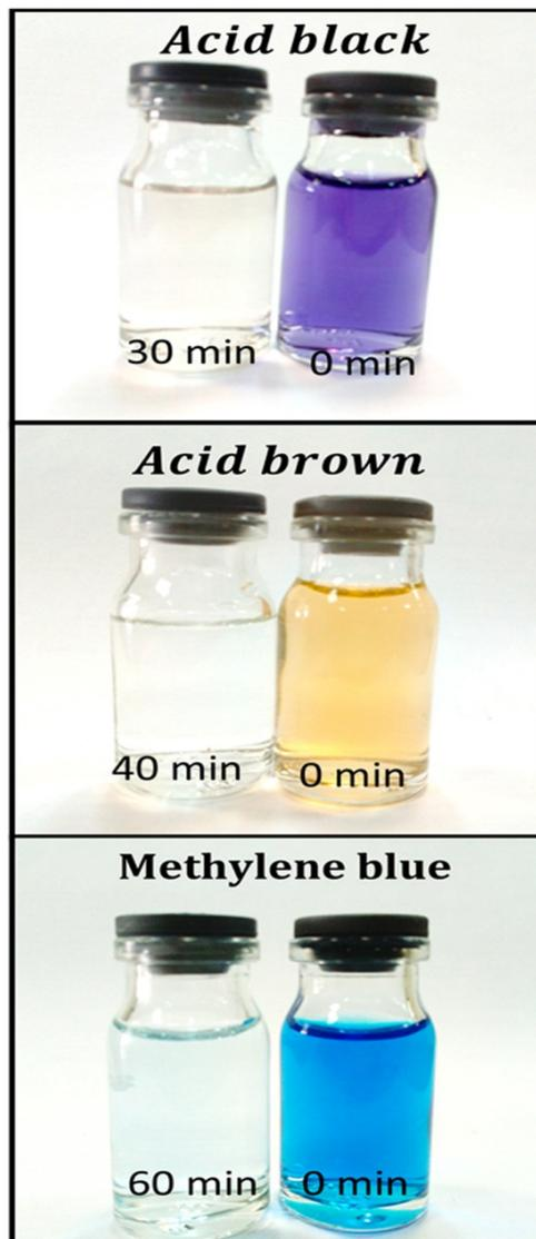
Fig. 12. Photocatalytic activity of iron oxide-zinc sulphide nano-composite
