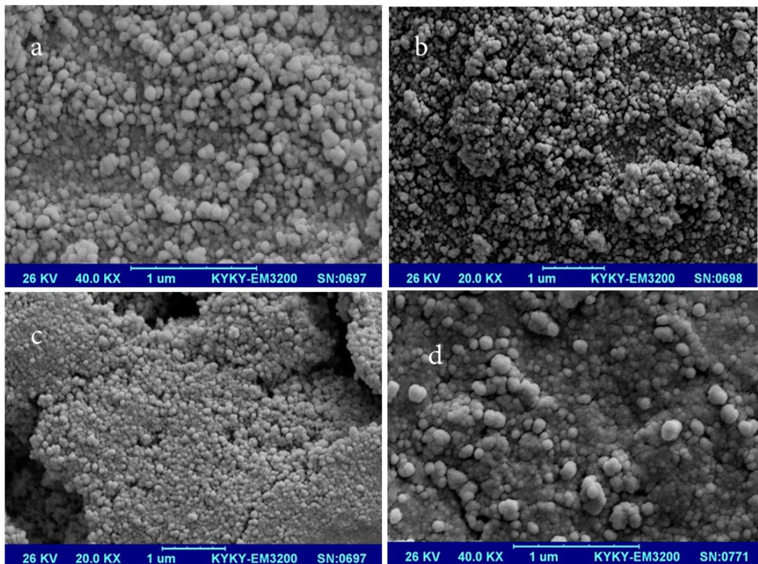
Fig. 3. SEM images of a) zinc sulphide with CH<sub>4</sub>N<sub>2</sub>S deposition factor b) zinc sulphide with C<sub>6</sub>H<sub>10</sub>O<sub>5</sub> deposition factor c) zinc sulphide with Na<sub>2</sub>S deposition factor d) Fe<sub>2</sub>O<sub>3</sub> with NH<sub>3</sub> deposition factor
