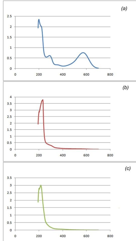
Fig. 7. UV-Vis spectra of degradation of acid black a) 0 min, b) 30 min in the presence of ZnS nanoparticles, c) 30 min in the presence of nano composite
