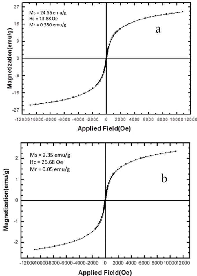
Fig. 5. Hysteresis loops of a) iron oxide nanoparticles b) iron oxide-zinc sulphide nano-composite
