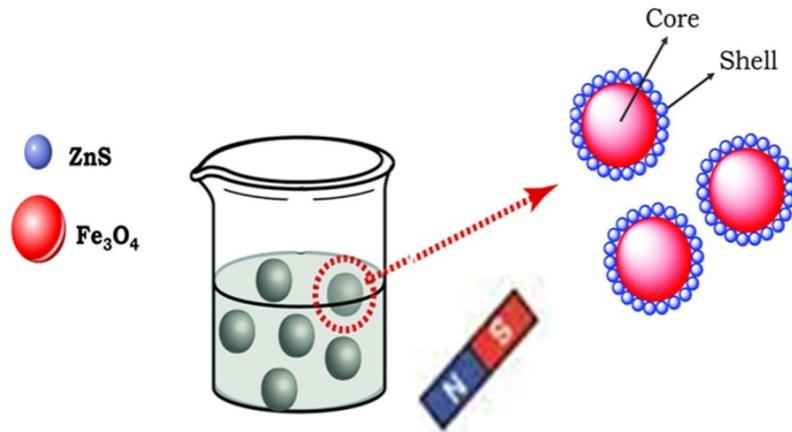
Fig. 11. Schematic of core-shell formation
