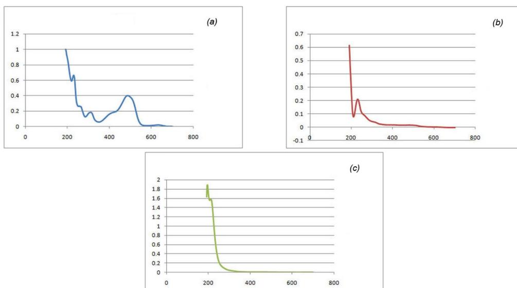
Fig. 8. UV-Vis spectra of degradation of acid brown a) 0 min, b) 30 min in the presence of ZnS nanoparticles, c) 30 min in the presence of nano composite
