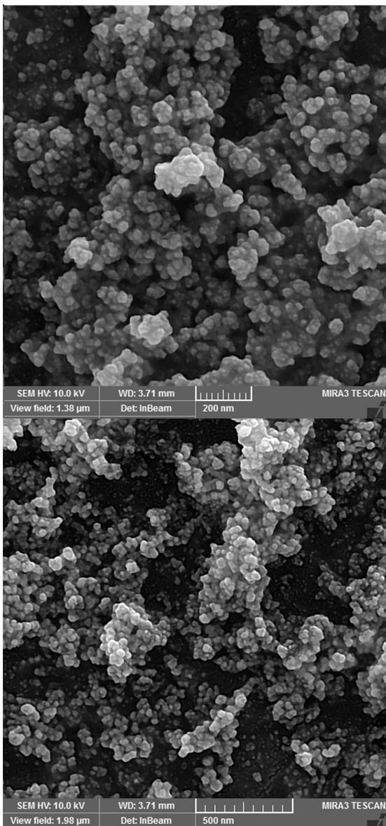
Fig. 4. SEM images of the Mg(OH)<sub>2</sub> nanoparticles
