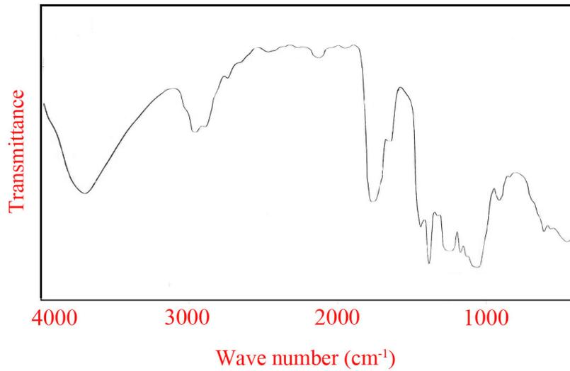
Fig. 6. FT-IR spectrum of the  $Mg(OH)_2$  nanoparticles
