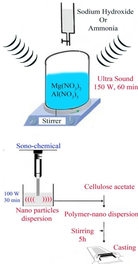
Fig. 1. Schematic of nanoparticle and nanocomposites preparation
