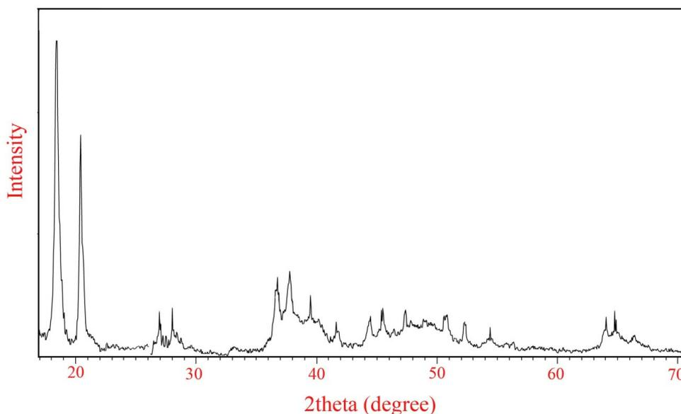
Fig. 3. XRD pattern of the Al(OH)<sub>3</sub> nanoparticles
