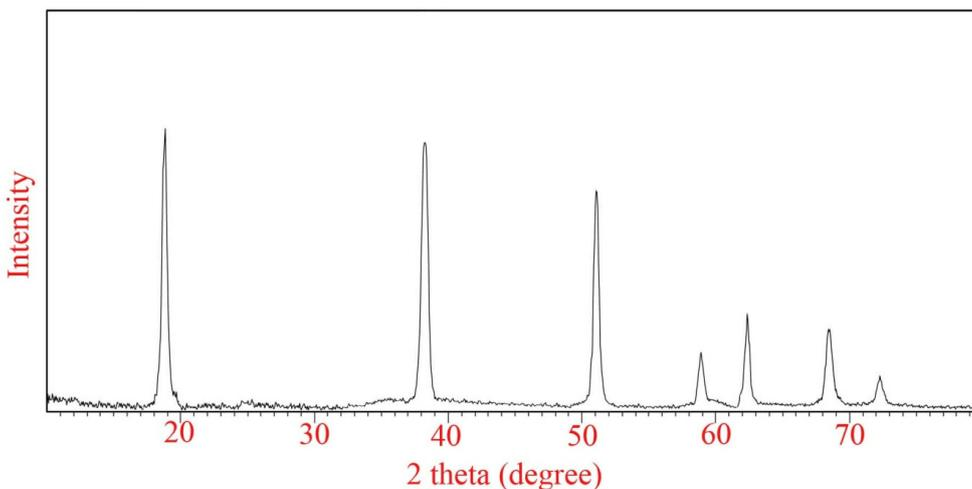
Fig. 2. XRD pattern of the Mg(OH)<sub>2</sub> nanoparticles
