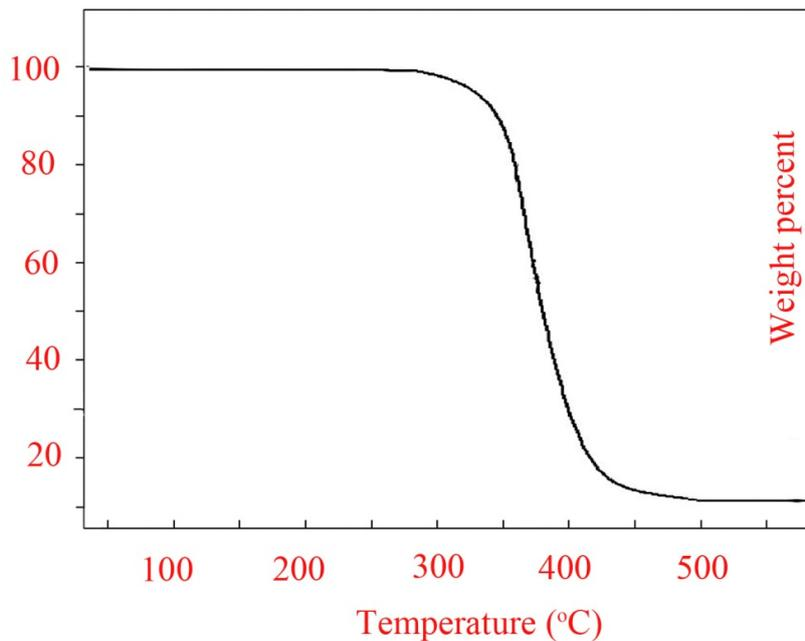
Fig. 7. TGA spectrum of the CA- $Mg(OH)_2$  nanocomposite
