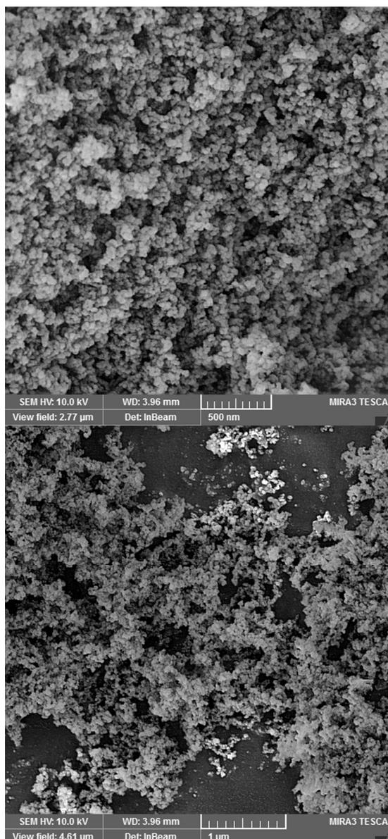
Fig. 5. SEM images of the Al(OH)<sub>3</sub> nanoparticles
