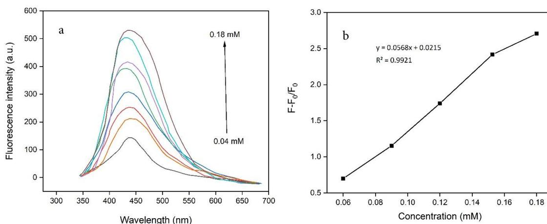
Fig. 6. a) Fluorescence emission spectra of carbon quantum dots- Cr(VI) in the presence of different concentration of ascorbic acid 0-0.18 mM b) linear correlation fluorescence intensity of carbon quantum dots- Cr(VI)-ascorbic acid and concentration of ascorbic acid.
