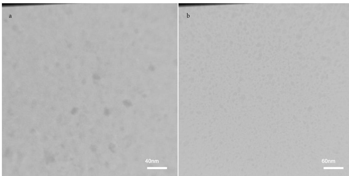
Fig. 3. TEM images of prepared carbon quantum dots
