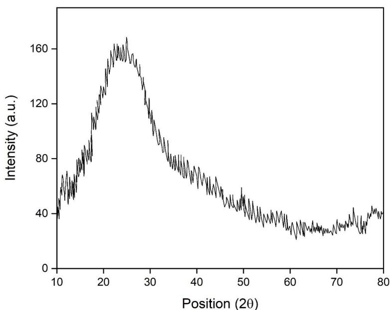
Fig. 1. XRD pattern of prepared carbon quantum dots
