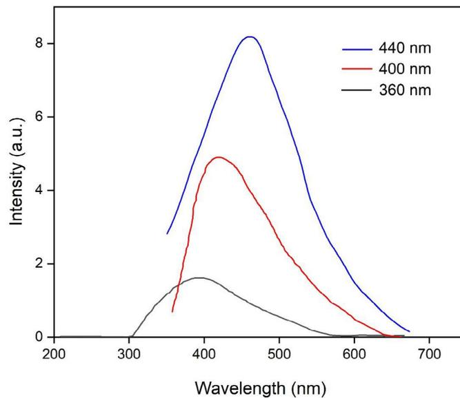
Fig. 5. The photoluminescence spectra of carbon quantum dots obtained by exciting the sample at different excitation
