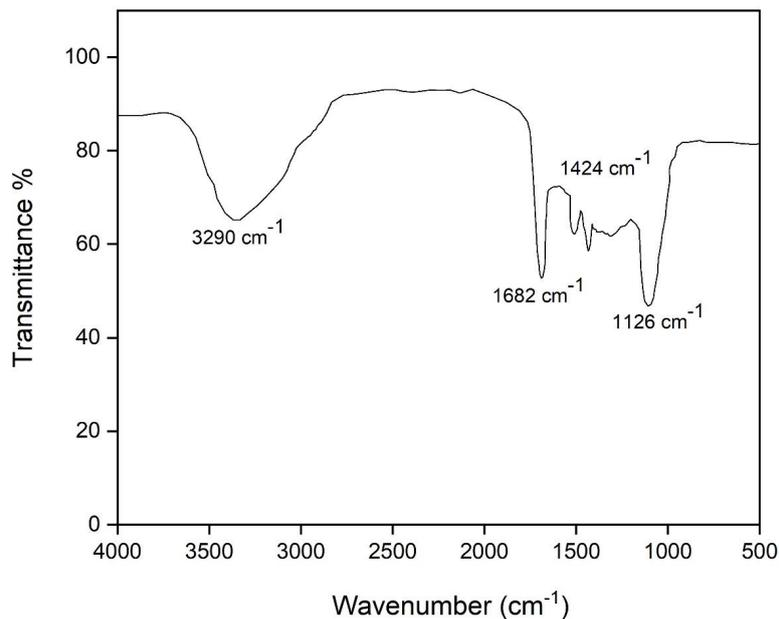
Fig. 2. FTIR spectra of prepared carbon quantum dots
