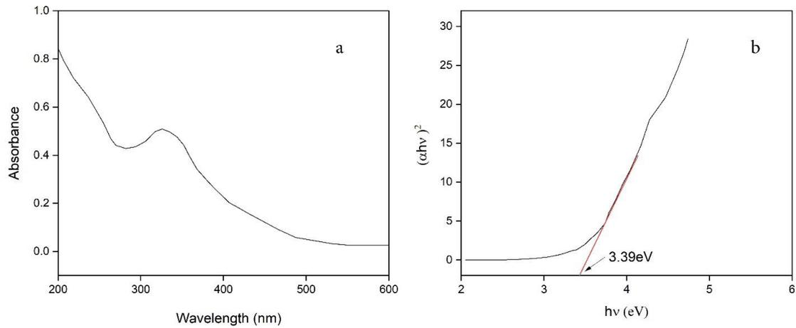
Fig. 4. a) UV-Vis absorption spectra and b) calculated band gap for carbon quantum dots
