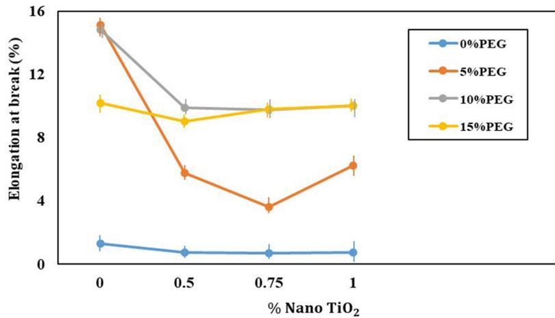
Fig. 7. Comparison of different wt. percentages between elongation and concentrations of nano TiO<sub>2</sub> and PEG as Reinforcement.
