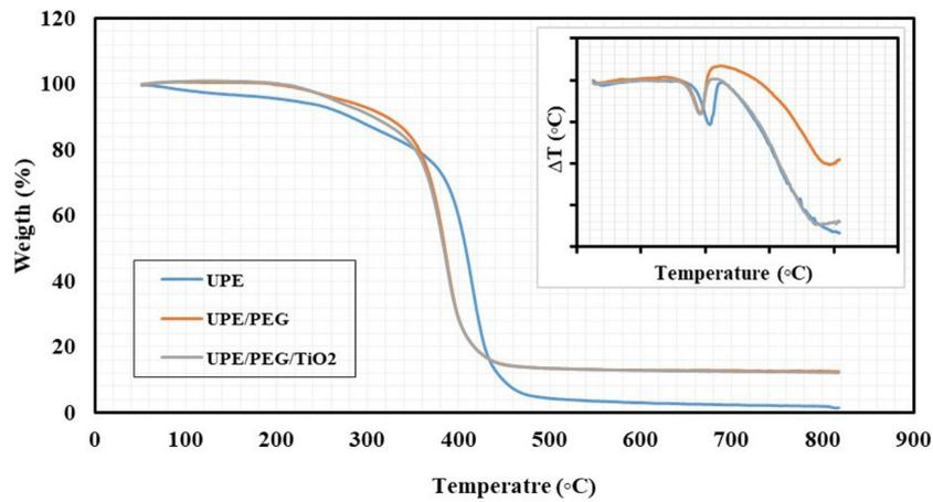
Fig. 8. TGA and DTA thermograms of UPE, UPE/PEG and UPE/PEG/TiO<sub>2</sub> nanocomposite.
