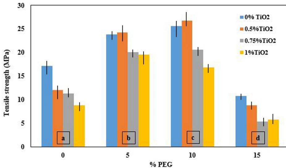
Fig. 5. Comparison of different wt. percentages between tensile strength and concentrations of nano TiO<sub>2</sub> and PEG as Reinforcement.
