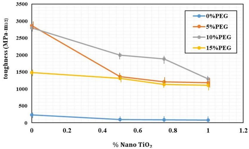
Fig. 6. Comparison of different wt. percentages between toughness and concentrations of nano TiO<sub>2</sub> and PEG as Reinforcement.
