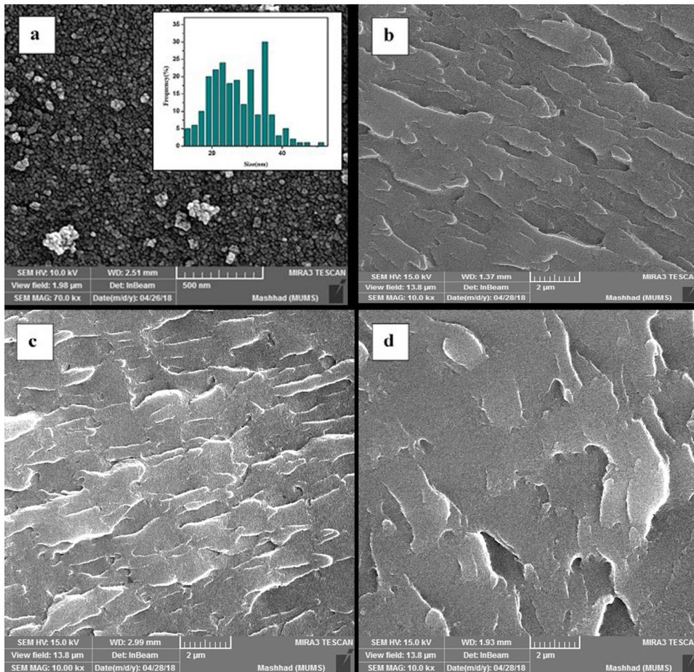
Fig. 3. SEM micrographs of fracture surface of (a) TiO<sub>2</sub>, (b) pure UPE, (c) UPE/PEG and (d) UPE/PEG/TiO<sub>2</sub>
