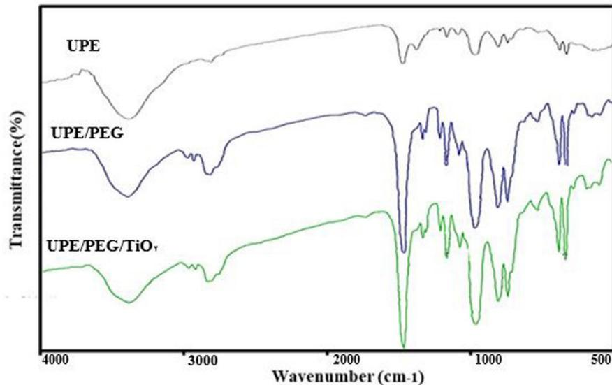
Fig. 4. FT-IR spectra of TiO<sub>2</sub>, UPE, UPE/PEG and UPE/PEG/TiO<sub>2</sub> nanocomposites.
