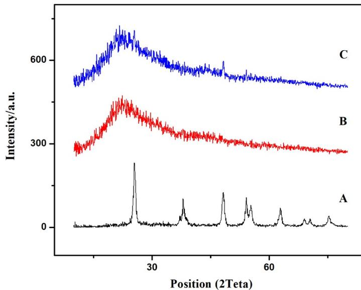
Fig. 2. XRD patterns of (A) TiO<sub>2</sub> nanoparticles, (B) unsaturated polyester and (C) UPE/PEG/TiO<sub>2</sub> nanocomposite
