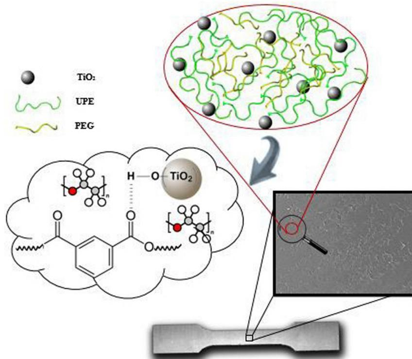
Fig. 1. Representation of the interaction fillers-polymer matrix.
