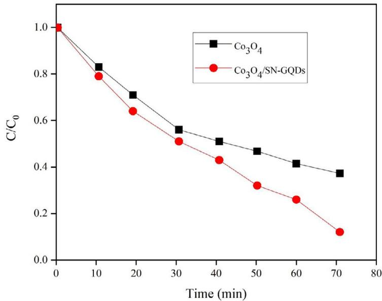
Fig. 6. Photocatalytic performance of prepared  $\text{Co}_3\text{O}_4$  nanoparticles and  $\text{Co}_3\text{O}_4/\text{SN-GQDs}$  nanocomposites against methylene blue
