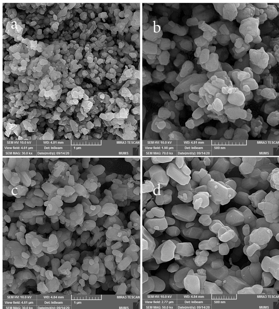
Fig. 3. SEM images of a,b)  $\text{Co}_3\text{O}_4$  nanoparticles c,d)  $\text{Co}_3\text{O}_4$ /SN-GQDs nanocomposites at two magnifications
