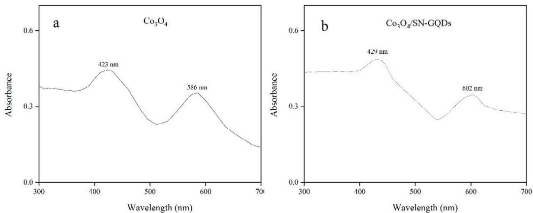
Fig. 5. UV-Vis analysis of prepared a)  $\text{Co}_3\text{O}_4$  nanoparticles b)  $\text{Co}_3\text{O}_4/\text{SN-GQDs}$  nanocomposites
