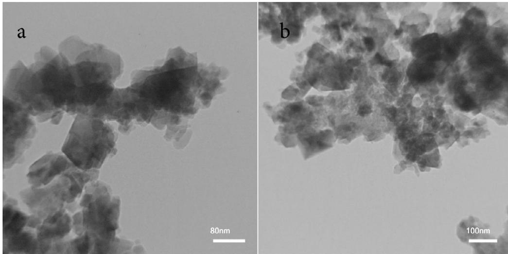
Fig. 4. TEM images of prepared Co<sub>3</sub>O<sub>4</sub>/SN-GQDs nanocomposites
