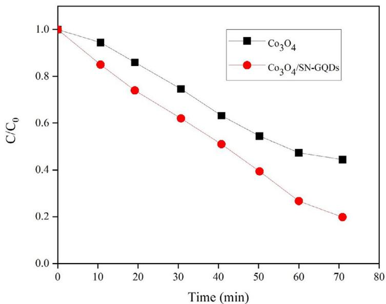
Fig. 7. Photocatalytic performance of prepared  $\text{Co}_3\text{O}_4$  nanoparticles and  $\text{Co}_3\text{O}_4/\text{SN-GQDs}$  nanocomposites against methyl orange
