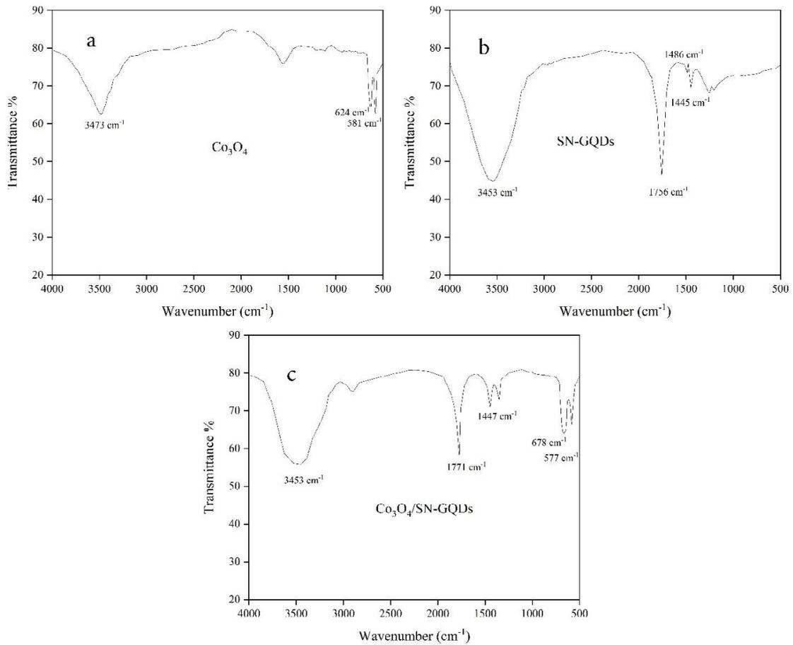
Fig. 2. FTIR spectrum of prepared a) Co<sub>3</sub>O<sub>4</sub> nanoparticles b) SN-GQDs and c) Co<sub>3</sub>O<sub>4</sub>/SN-GQDs nanocomposites
