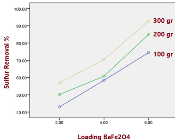
Fig. 7. Average removal efficiency percentage of Hydrogen sulfide in different weights and concentrations
