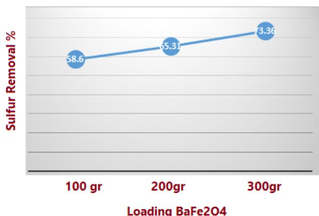
Fig.6. Average efficiency percentage of Hydrogen sulfide removal in different weights
