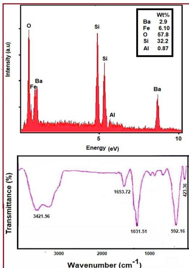
Fig.4. (a) FT-IR spectrum (b) EDX from sample 5
