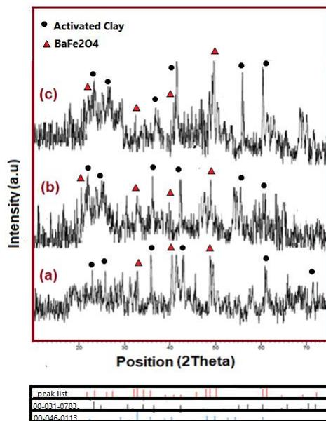
Fig. 3. XRD patterns of as-prepared nanocomposites; (a) sample 3, (b) Sample 4, (c) sample 5
