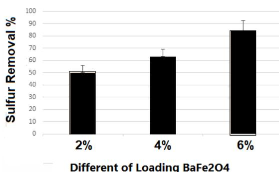
Fig. 5. Average efficiency percentage of Hydrogen sulfide removal in different concentrations
