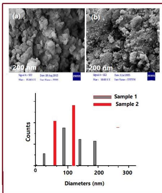
Fig. 1. FESEM micrographs of nanoferrite (a) sample 1, (c) sample 2
