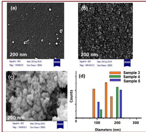
Fig. 2. FESEM micrographs of nanocomposites (a) sample 3, (b) sample 4 (c) sample 5
