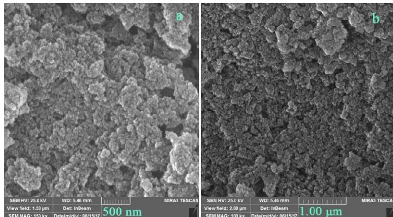
Fig. 8. FESEM images of SrMnO<sub>3</sub>/Ag nanostructures (sample 6)
