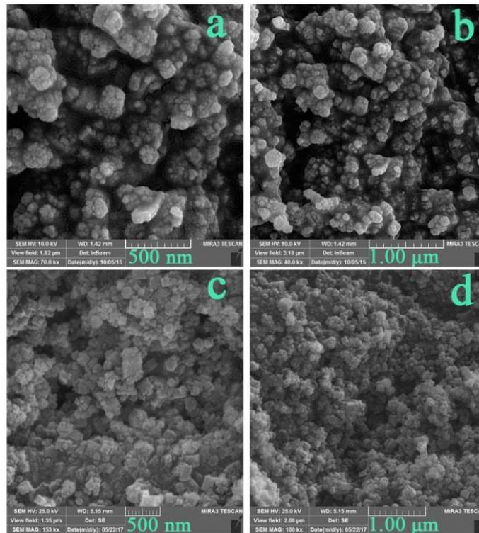
Fig. 6. FESEM images of the samples obtained by various alkaline agents; NH<sub>3</sub> (a, b), and TEPA (c, d)
