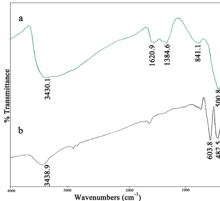
Fig. 5. FT-IR spectra of (a) SrMnO<sub>3</sub> nanostructures (sample 5 before calcination) and (b) SrMnO<sub>3</sub> nanostructures after calcination (sample 5)
