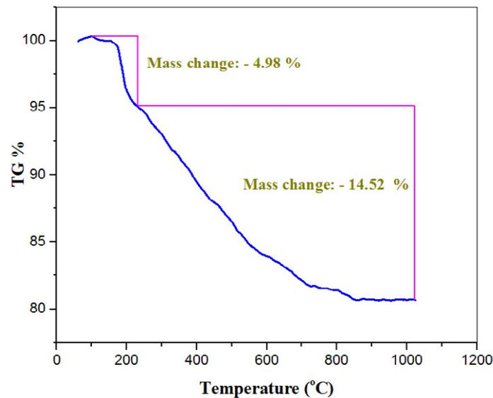
Fig. 2. TGA curve of as-formed nanostructures (sample no. 1 before calcination stage).
