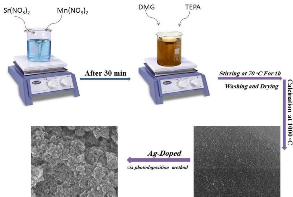
Fig. 1. Schematic diagram of the synthesis of SrMnO<sub>3</sub>/Ag nanostructures
