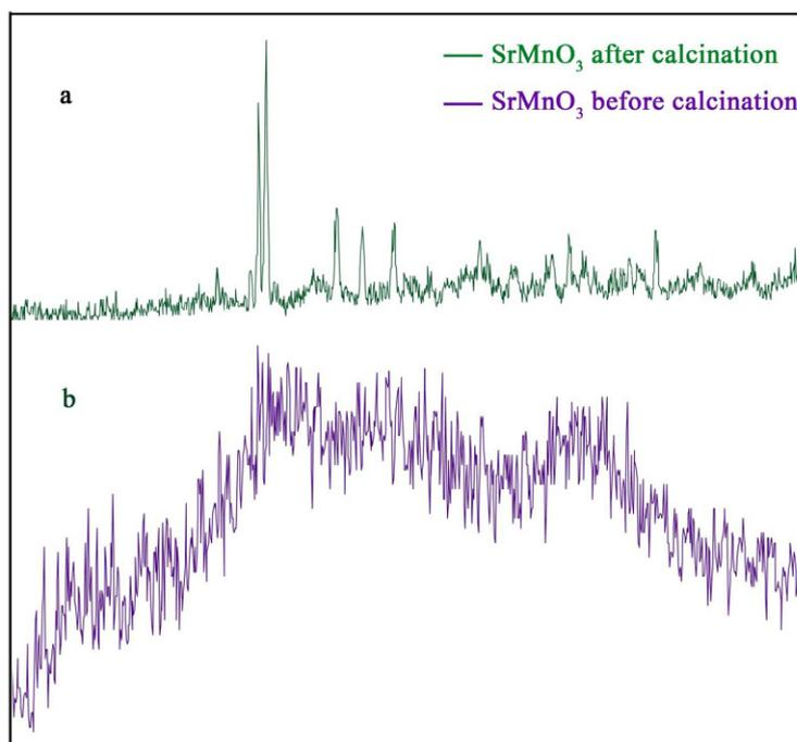
Fig. 3. XRD patterns of (a) SrMnO<sub>3</sub> calcinated at 1000 °C and (b) SrMnO<sub>3</sub> before calcination
