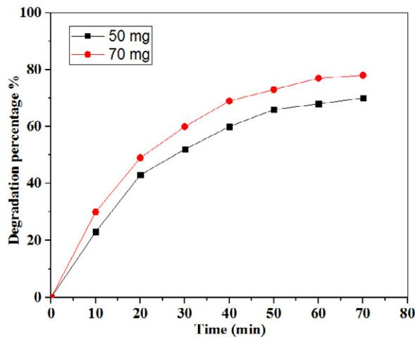
Fig 14. The influence of the concentration of photocatalyst (sample 6) on the photocatalytic performance for degradation of rhodamine B
