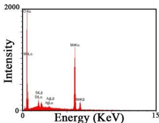
Fig. 4. EDS pattern of SrMnO<sub>3</sub>/Ag nanostructures
