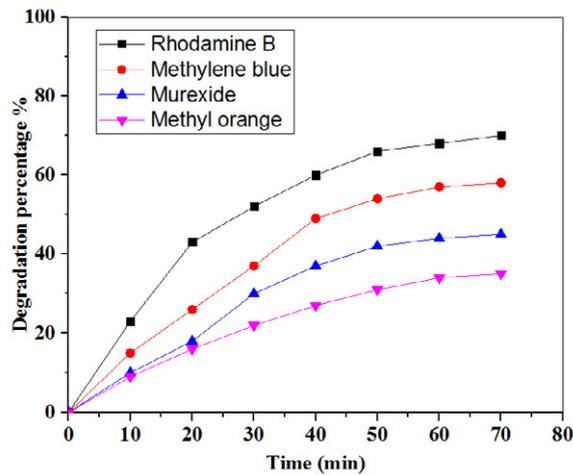
Fig. 13. The photocatalytic behavior of SrMnO<sub>3</sub>/Ag nanostructures (sample 6) on decomposition of rhodamine B, methyl orange, methylene blue and murexide
