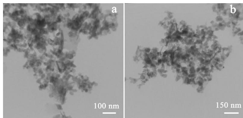
Fig. 9. TEM images of SrMnO<sub>3</sub>/Ag nanostructures (sample no. 6).
