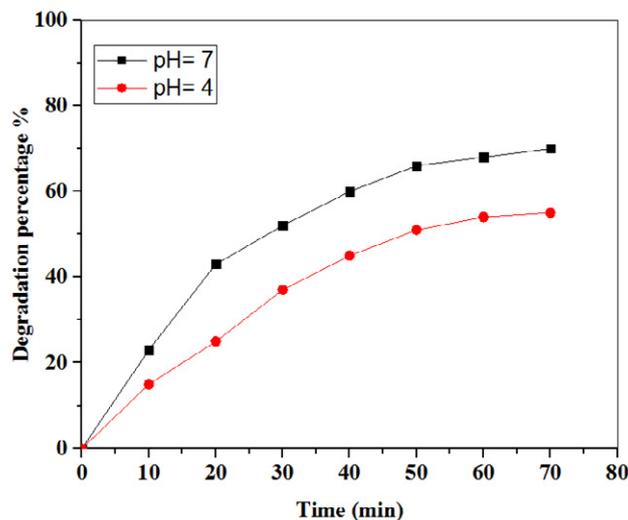
Fig. 15. Effect of pH on the photocatalytic decomposition of rhodamine B
