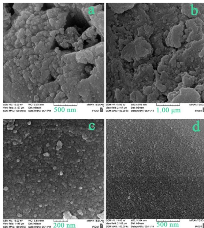
Fig. 7. FESEM images of the products prepared by different capping agents; 2-hydroxy-1-naphthaldehyde (a, b), DMG (c, d)
