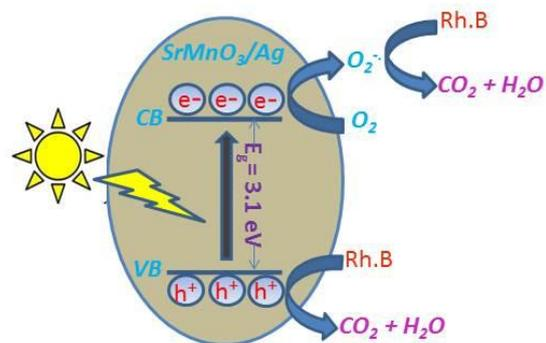
Fig. 11. Schematic diagram of the reaction mechanism of rhodamine B photodegradation by SrMnO<sub>3</sub>/Ag
