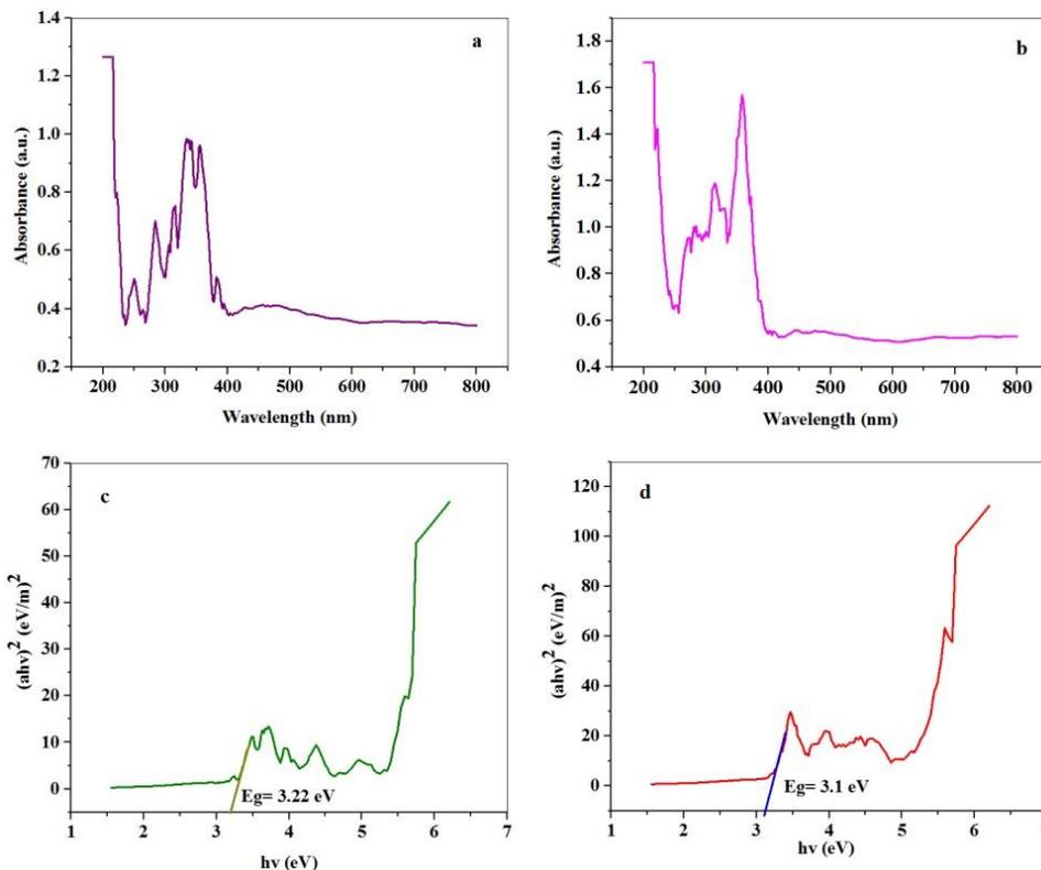
Fig. 10. UV-Vis diffuse reflectance spectrum and plot to determine the band gap of the SrMnO<sub>3</sub> (sample 5) (a and c) and UV-Vis diffuse reflectance spectrum and plot to determine the band gap of the SrMnO<sub>3</sub>/Ag nanostructures (sample 6) (b and d)
