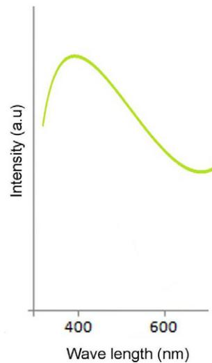
Fig. 8. UV-vis absorption analysis of carbon dot nanoparticles
