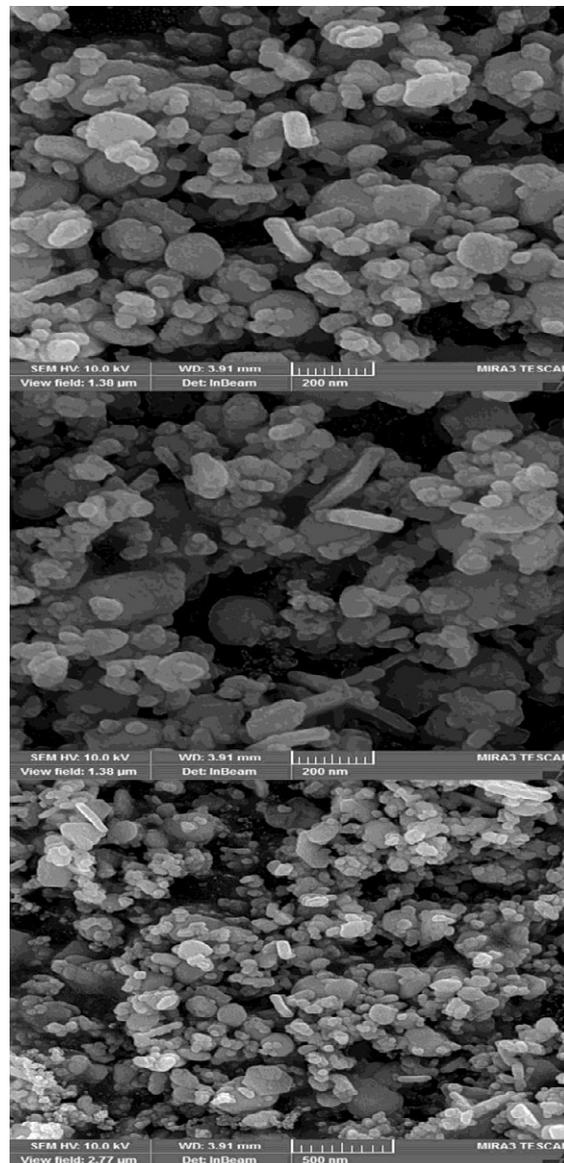
Fig. 5. SEM image of  $\text{CuFe}_2\text{O}_4$  nanoparticles 10 min 600W
