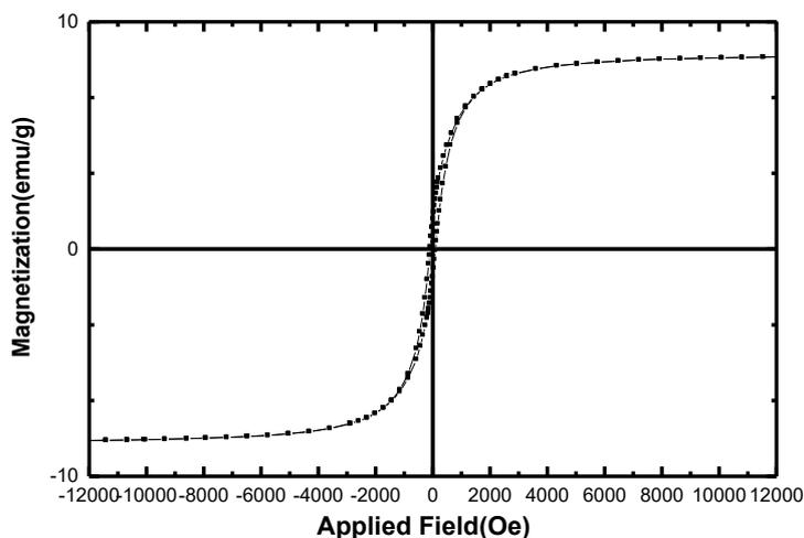
Fig. 10. VSM curve of  $\text{CuFe}_2\text{O}_4$ -carbon dot nanocomposite
