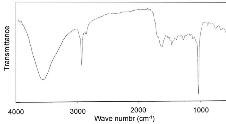
Fig. 4. FT-IR spectrum of  $\text{CuFe}_2\text{O}_4$ -carbon dot
