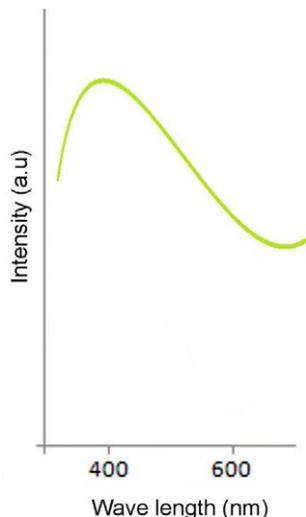
Fig. 8. UV-vis absorption analysis of carbon dot nanoparticles
