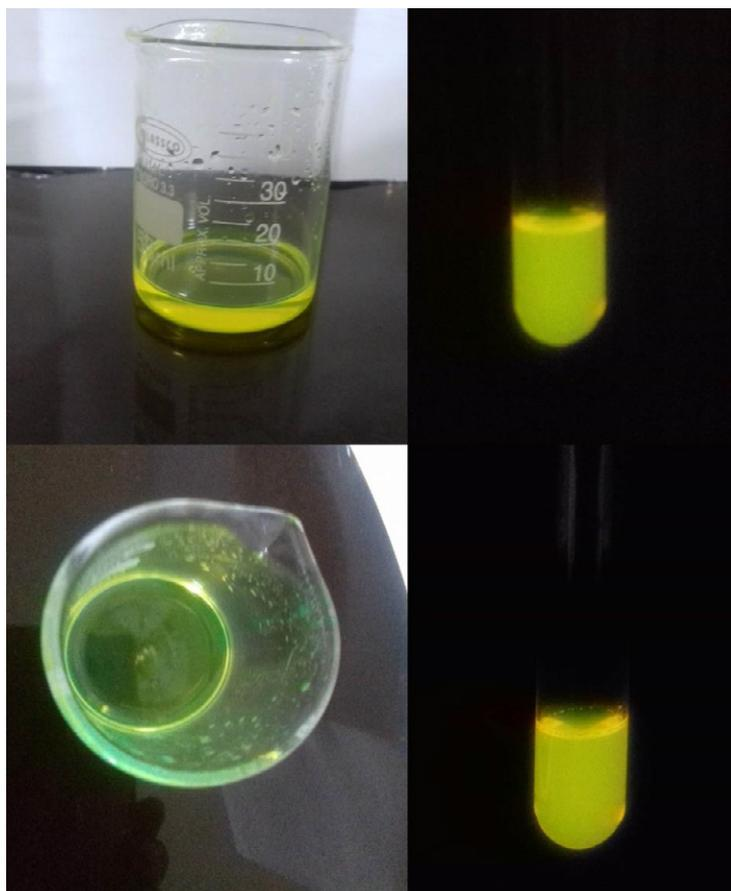
Fig. 2. Carbon quantum dot under UV irradiation
