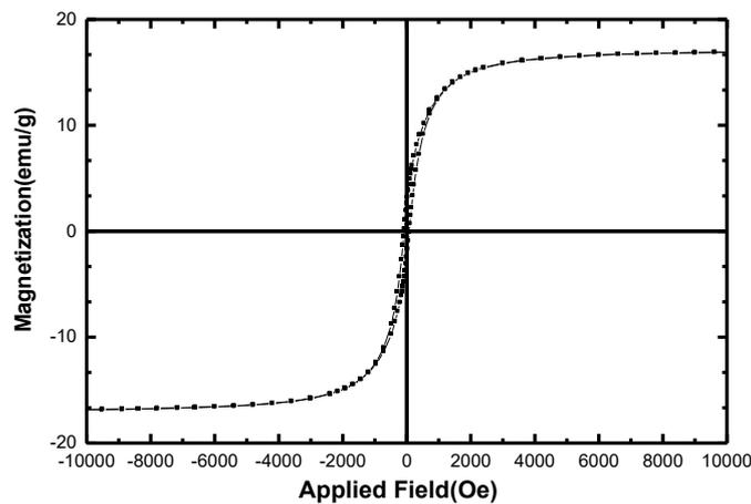
Fig. 9. VSM curve of  $\text{CuFe}_2\text{O}_4$  nanoparticles
