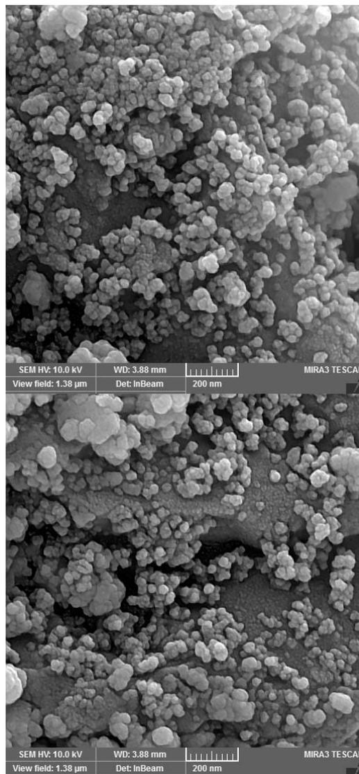
Fig. 7. SEM images of  $\text{CuFe}_2\text{O}_4$ -carbon dot at 200 °C for 24h
