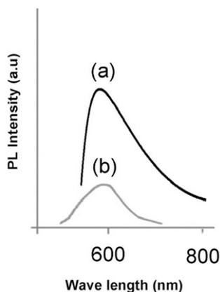
Fig. 11. PL spectra of products at 200 °C (a) pure (b) after addition of  $\text{Hg(II)}$  ions
