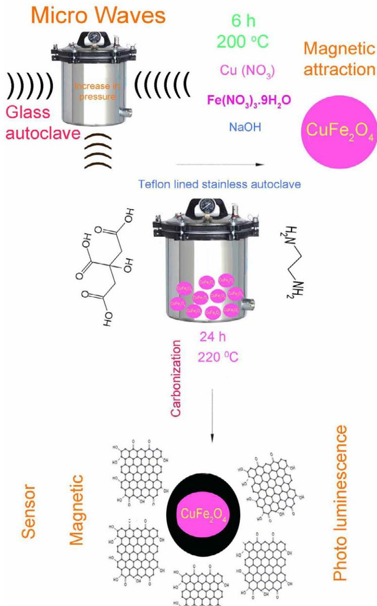
Fig. 1. Schematic of preparation of copper ferrite-carbon dot nanocomposite
