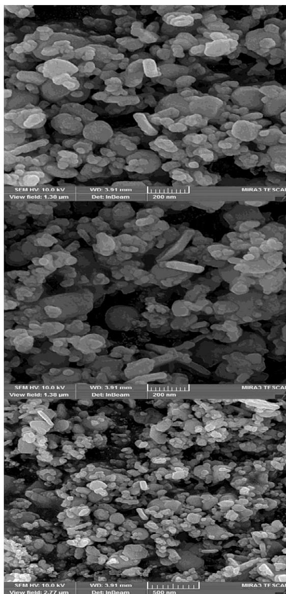
Fig. 5. SEM image of  $\text{CuFe}_2\text{O}_4$  nanoparticles 10 min 600W
