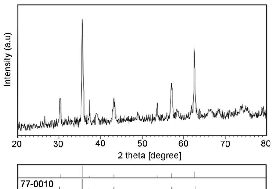
Fig. 3. XRD patterns of  $\text{CuFe}_2\text{O}_4$ -carbon dot nano composite
