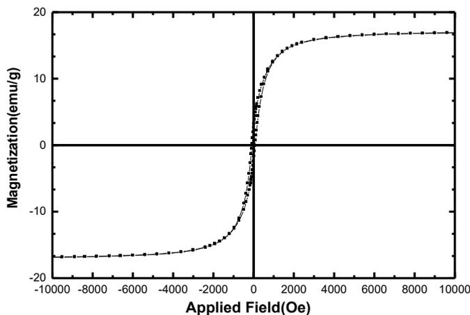
Fig. 9. VSM curve of CuFe<sub>2</sub>O<sub>4</sub> nanoparticles
