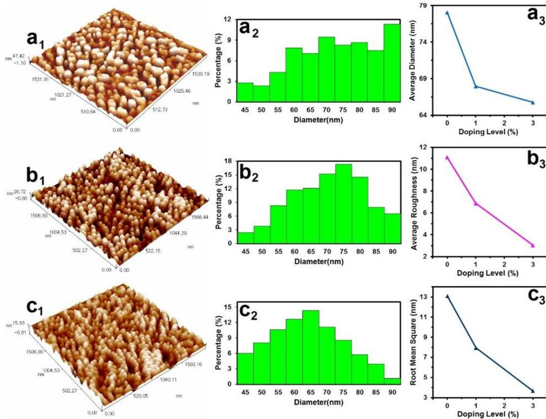
Fig. 3. AFM images of the prepared films (a<sub>1</sub>, b<sub>1</sub> and c<sub>1</sub>), granularly distributed (a<sub>2</sub>, b<sub>2</sub> and c<sub>2</sub>), and variation of AFM parameters via doping (a<sub>3</sub>, b<sub>3</sub> and c<sub>3</sub>).
