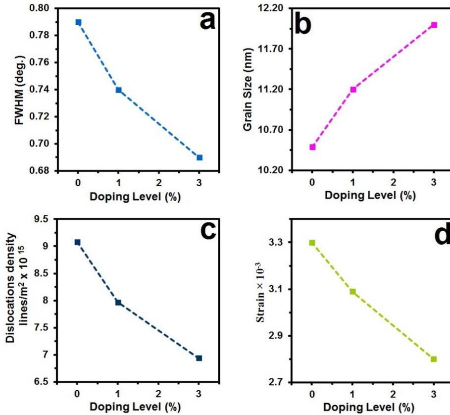
Fig. 2. FWHM (a), Grain size (b), Dislocation (c), and Strain (d) of the prepared films.
