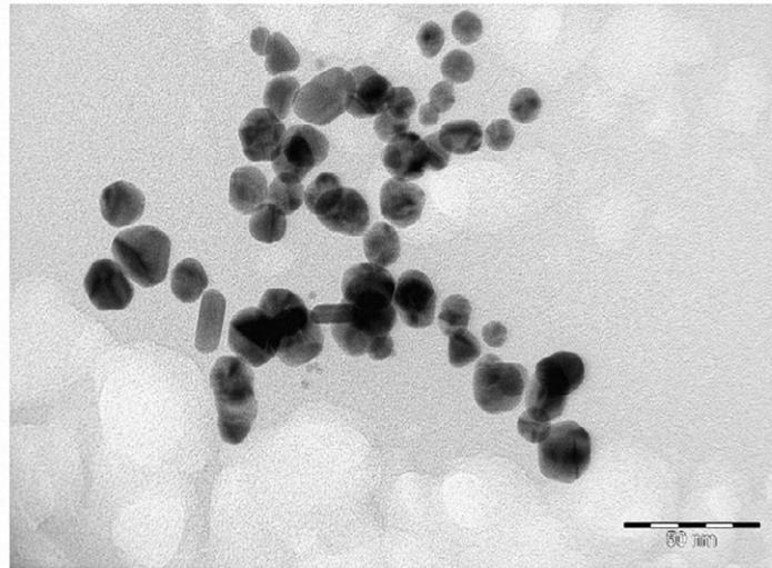
Fig. 5. TEM image of gold nanoparticles.
