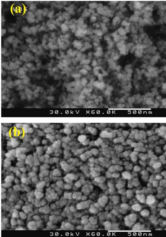
Fig. 2. SEM images of  $\text{Fe}_3\text{O}_4$  nanoparticles, prepared by (a)  $\text{NH}_3$  addition (b)  $\text{NaOH}$  addition
