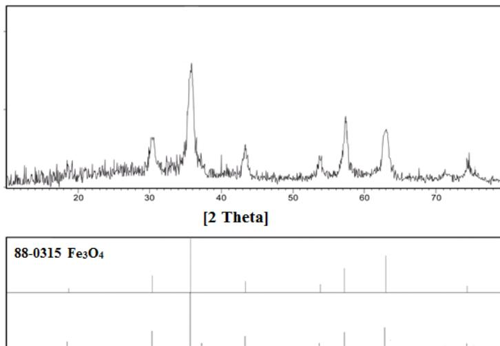
Fig. 4. XRD pattern of magnetite nanoparticles
