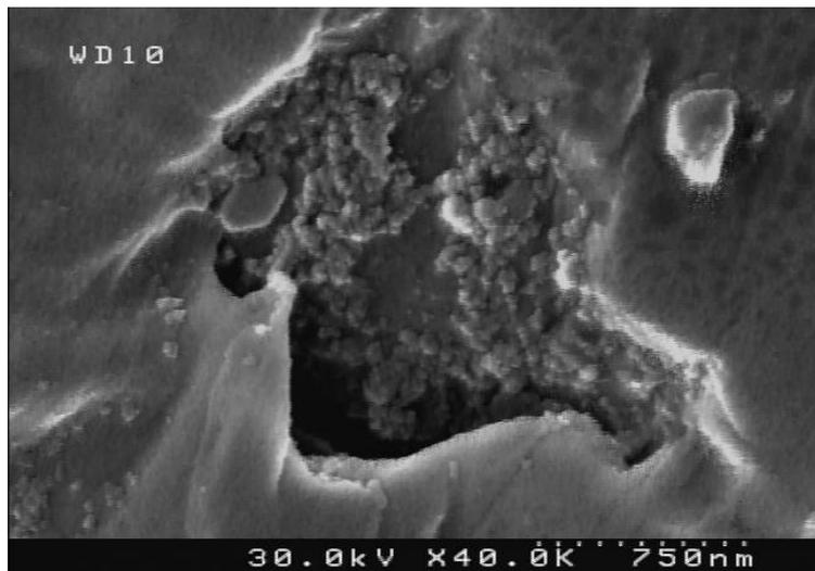
Fig. 6. SEM images of prepared nanocomposite (PS/ZnO+ Graphene oxide)
