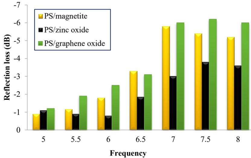
Fig. 8. Reflection loss for the prepared nanocomposites (frequency range: 5 to 8 GHz)
