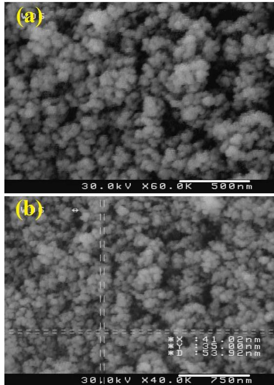
Fig. 3. SEM images of  $\text{ZnO}$  nanoparticles prepared by (a,b)  $\text{NH}_3$  addition
