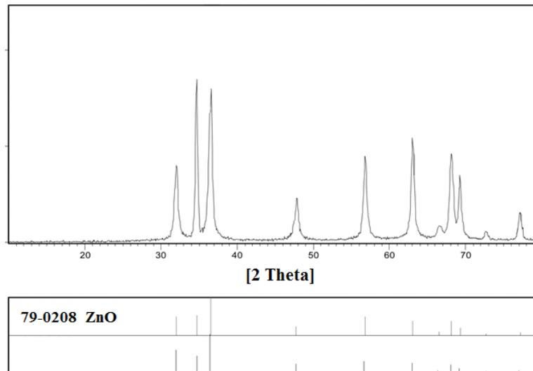
Fig. 5. XRD pattern of zinc oxide nanoparticles
