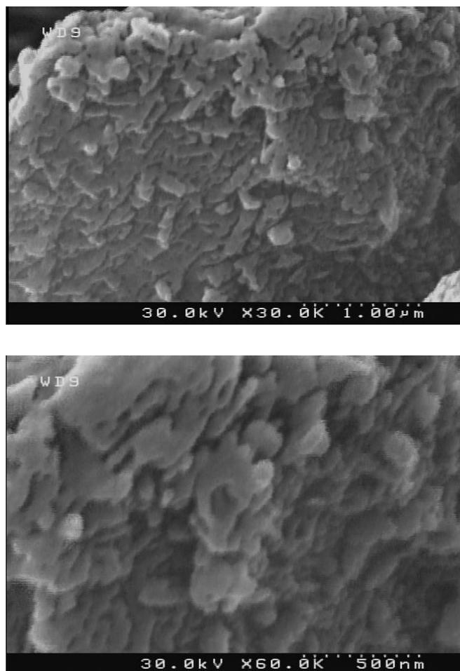
Fig. 1. SEM images of  $\text{Fe}_3\text{O}_4$  nanoparticles prepared by NaOH addition at 250 ml of water
