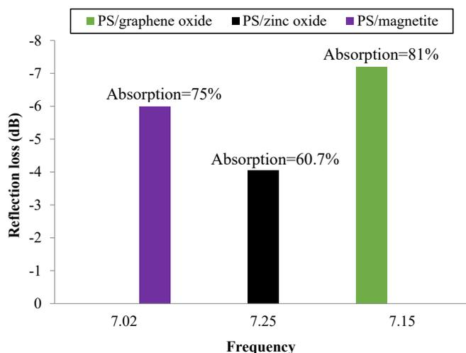
Fig. 9. Maximum reflection loss and absorption percentage of the prepared nanocomposites
