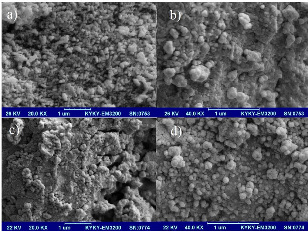
Fig. 6. SEM images of calcium ferrite nanoparticles a) with salicylic acid calcined at 500 °C, b) by applying KOH, c) by using starch and d) prepared at 200 ml of water.
