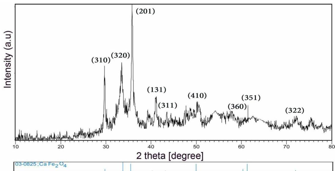
Fig. 2. XRD pattern of  $\text{CaFe}_2\text{O}_4$  nanoparticles.
