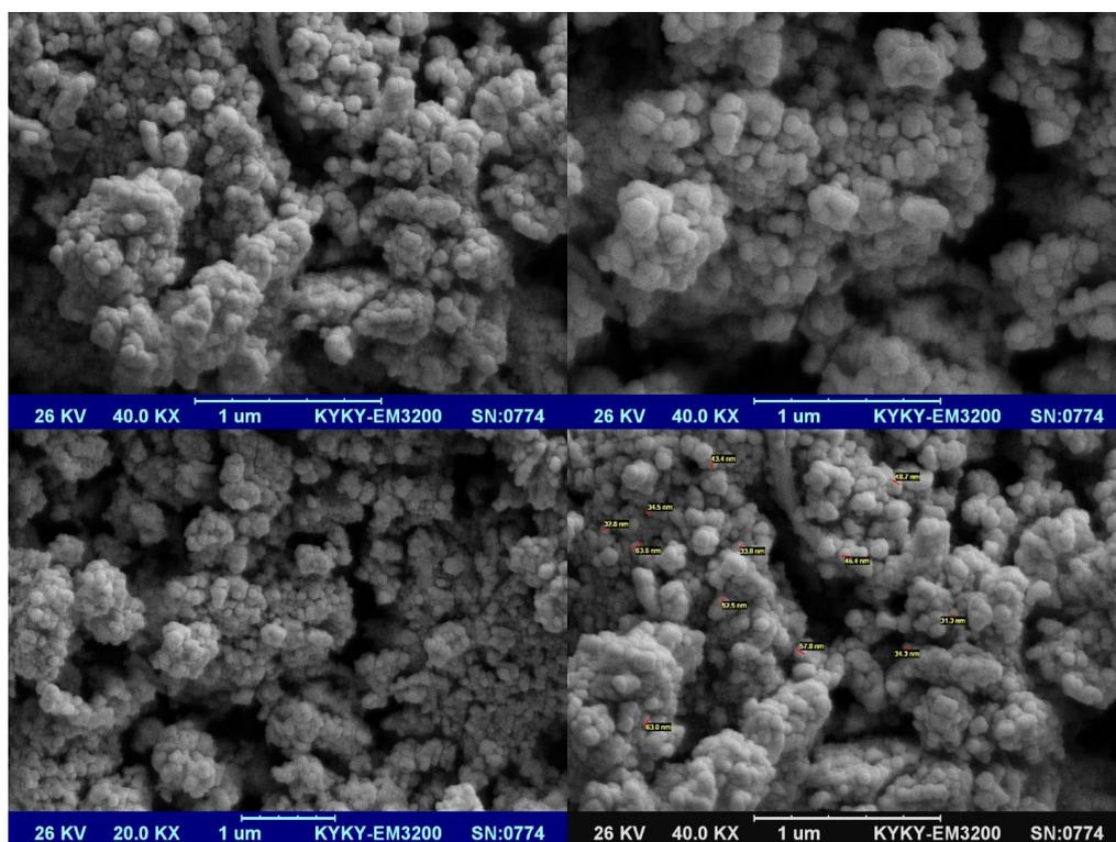
Fig. 9. SEM images of  $\text{CaFe}_2\text{O}_4\text{-CeO}_2$  nanocomposite
