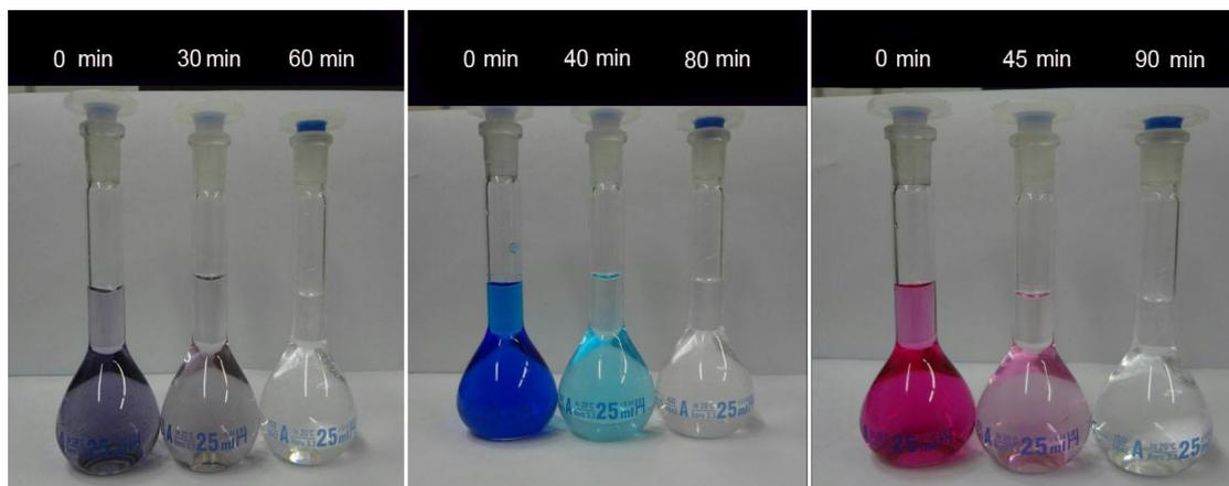
Fig. 15. Photo-degradation of (a) acid black 1 (b) acid blue 92 and (c) acid violet 43
