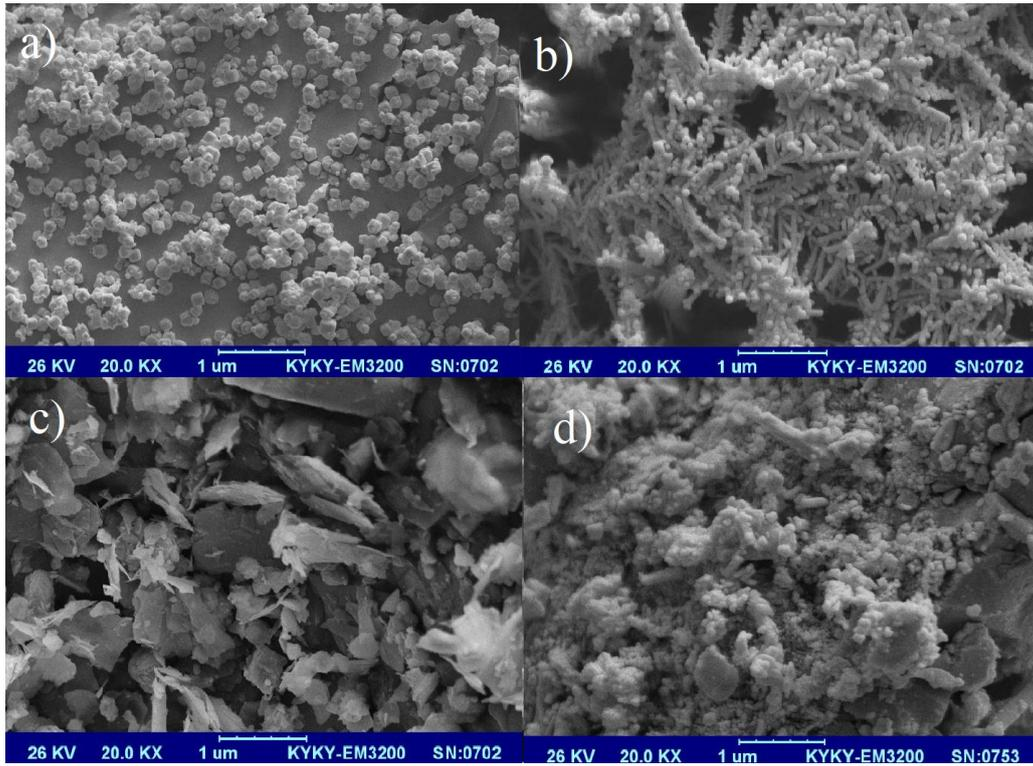
Fig. 5. SEM images of calcium ferrite nanoparticles with a) glucose, b) starch, c) poly vinyl pyrrolidone and d) gelatin.
