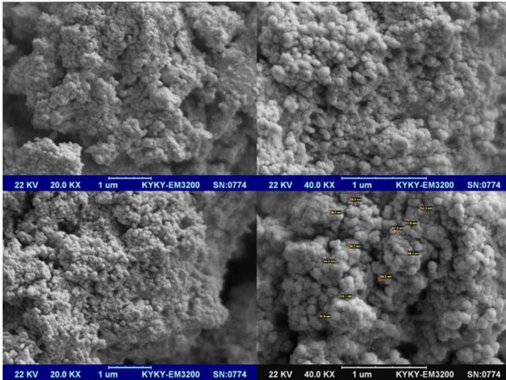
Fig. 7. SEM images of calcium ferrite nanoparticles via hydrothermal method
