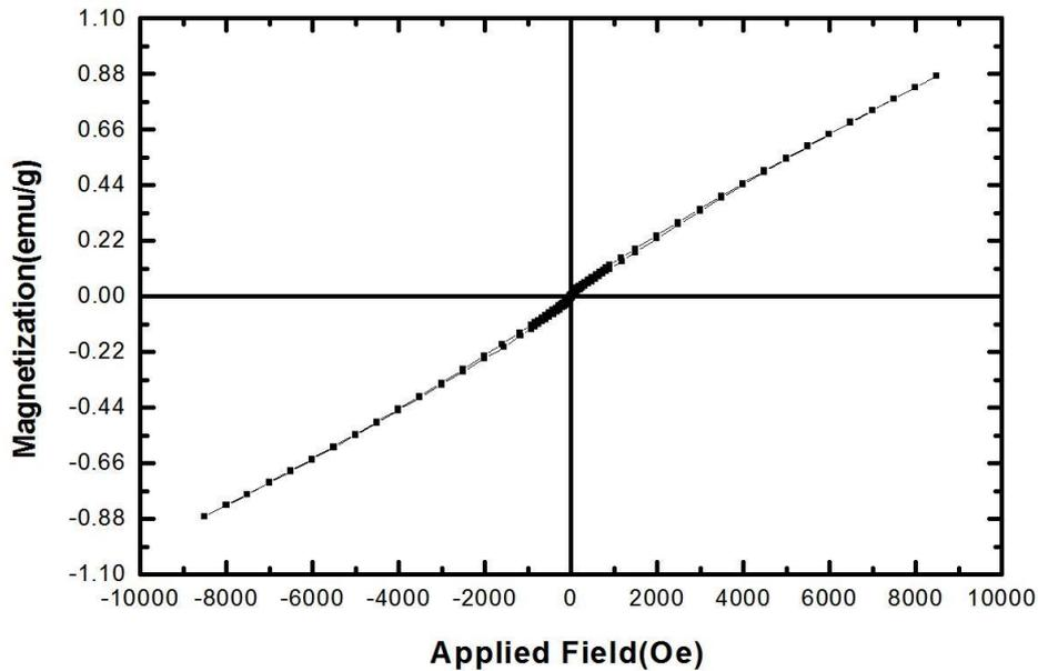
Fig. 11. VSM curve of room- temperature prepared calcium ferrite nanoparticles
