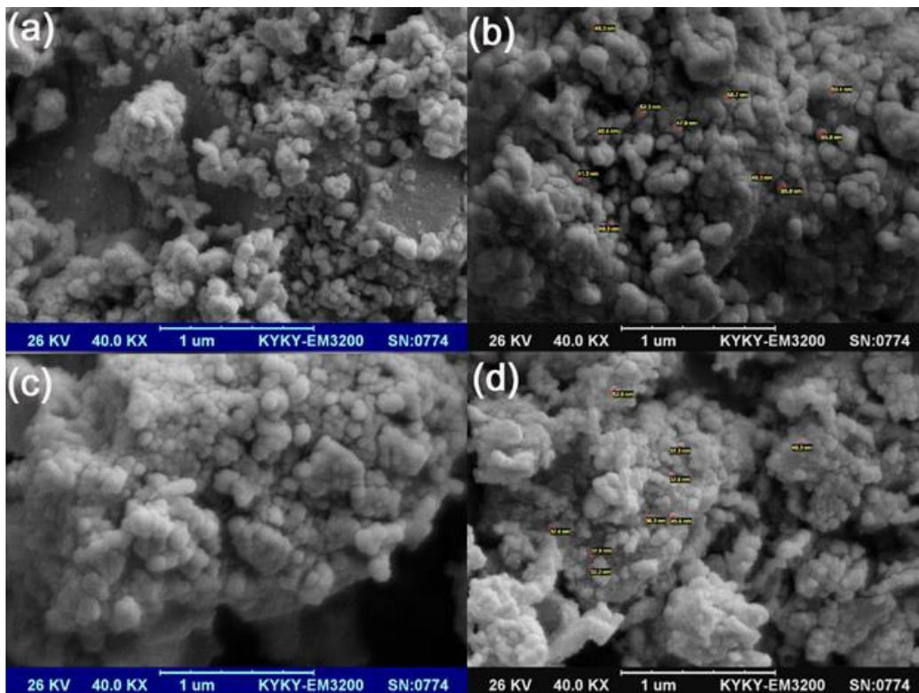
Fig. 8. (a,b) SEM images of the room temperature prepared  $\text{CeO}_2$ , (c,d) SEM images of the  $\text{CeO}_2$  that calcined at  $500\text{ }^\circ\text{C}$
