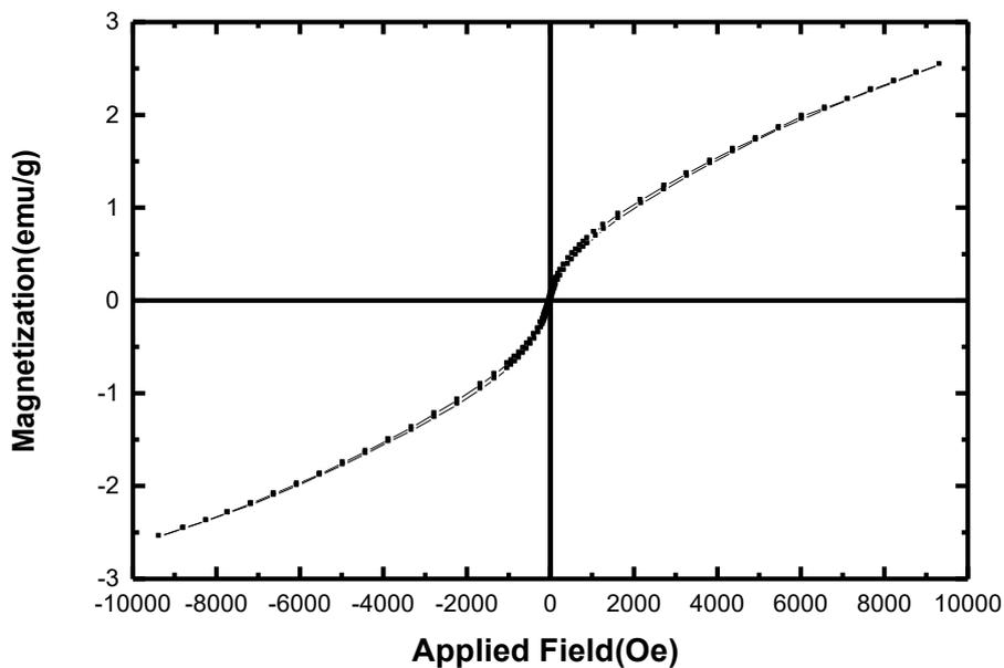
Fig. 12. VSM curve of calcium ferrite nanoparticles calcined at  $500\text{ }^\circ\text{C}$
