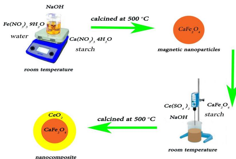
Fig. 1. Schematic of ferrite preparation nanocomposite.
