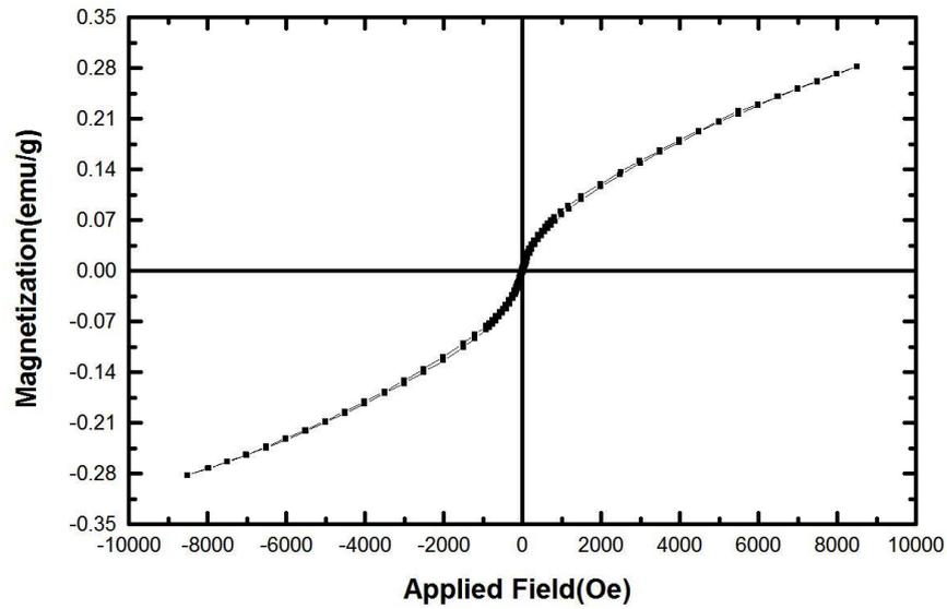
Fig. 13. VSM curve of  $\text{CaFe}_2\text{O}_4\text{-CeO}_2$  nanocomposite
