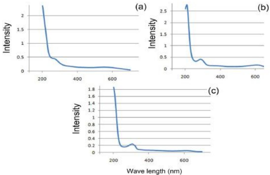
Fig. 14. UV-Vis absorption (a) acid black (b) acid blue (c) acid violet
