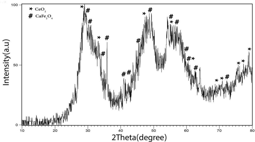
Fig. 4. XRD pattern of  $\text{CaFe}_2\text{O}_4$ - $\text{CeO}_2$  nanocomposite.
