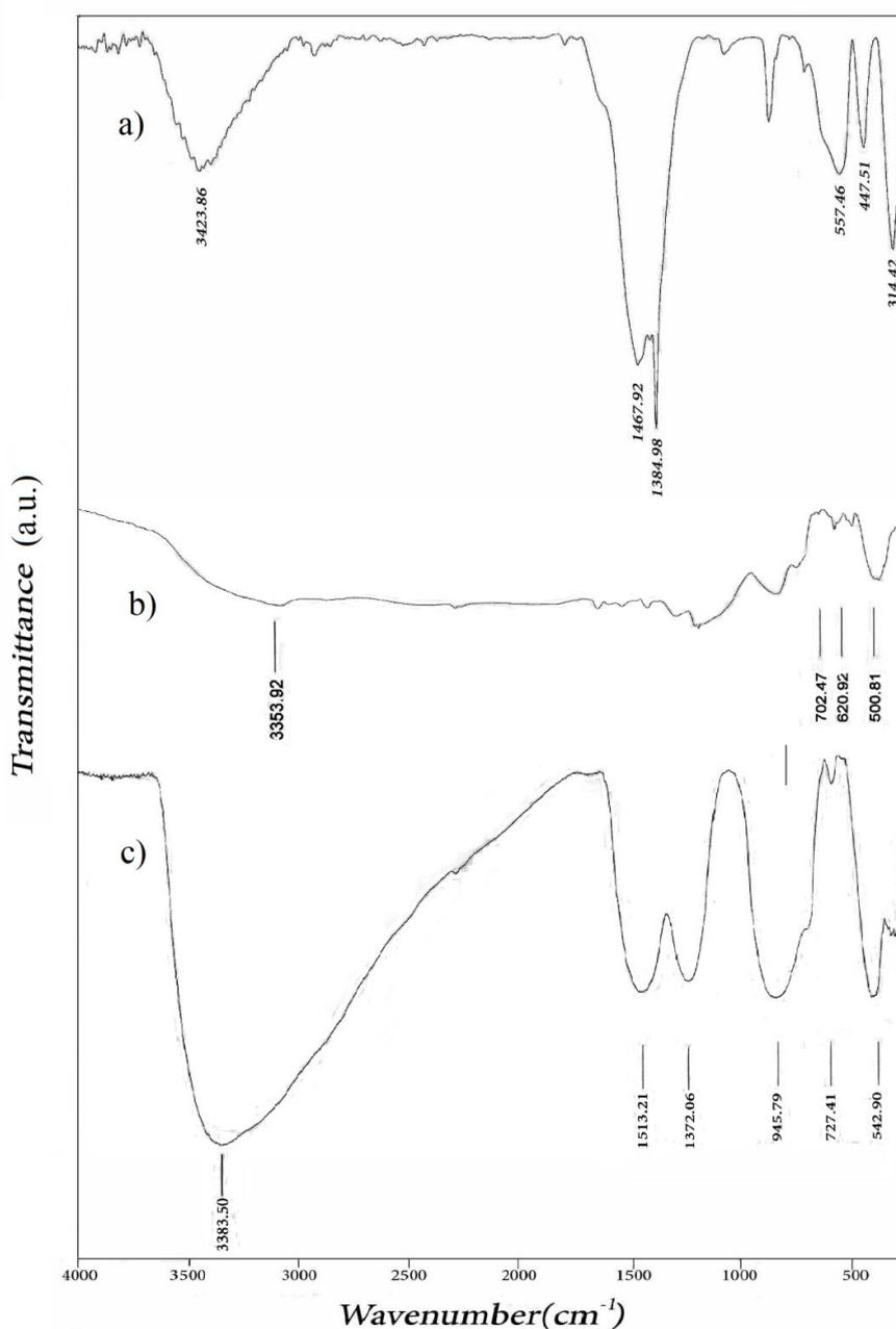
Fig. 10. FT-IR spectrum of a)  $\text{CaFe}_2\text{O}_4$  nanoparticles, b)  $\text{CeO}_2$  nanoparticles and c)  $\text{CaFe}_2\text{O}_4\text{-CeO}_2$  nanocomposite.
