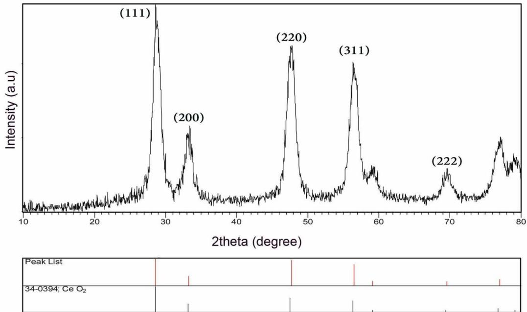
Fig. 3. XRD pattern of  $\text{CeO}_2$  nanoparticles.
