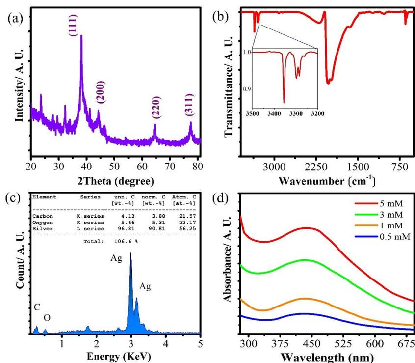
Fig. 1. Typical (a) XRD diffraction pattern, (b) FTIR spectrum, (c) EDX analysis, and (d) UV-Vis spectra of a typical Ag-NPs synthesized by plant extract.
