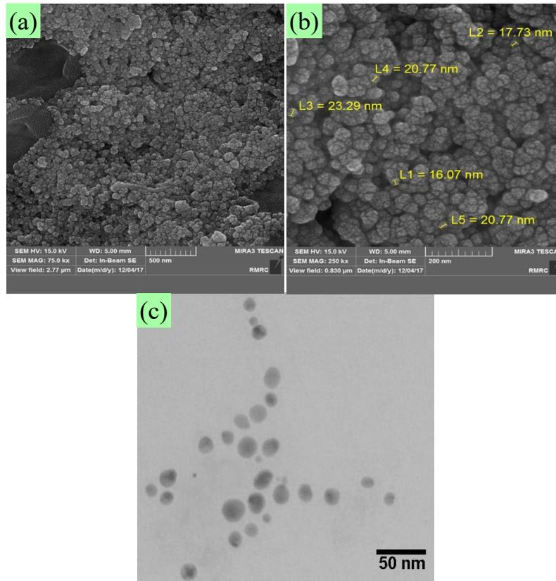
Fig. 2. (a, b) FE-SEM images of the bio-synthesized Ag-NPs at different magnifications. (c) TEM image of the same sample of Ag-NPs.
