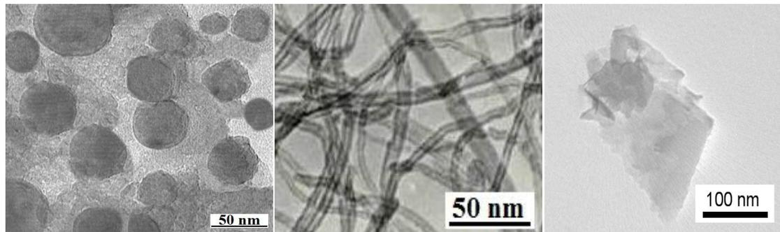
Fig. 1. TEM of a) SiO<sub>2</sub> b) CNT c) Graphene
