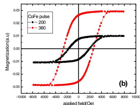
**Fig. 4.** The hysteresis loops of (a) as-prepared and (b) annealed samples with 300 Cu pulse and 200, 400 CoFe pulse.
