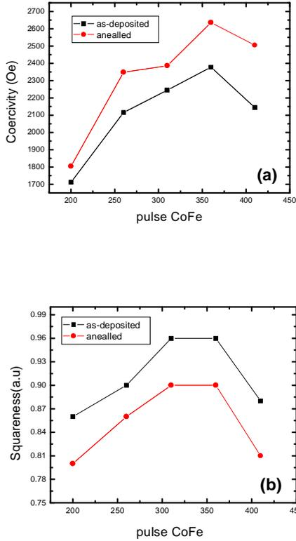
**Fig. 5.** (a) coercivity ( $H_c$ ) and (b) The squaresness ( $S_q$ ) of prepared and annealed samples as a function of CoFe pulses.
