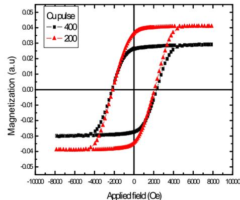
**Fig. 9.** The hysteresis loops of as-prepared samples with 360 CoFe pulse and 200, 400 Cu pulse.
