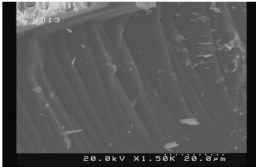
Fig. 3. SEM of silicon nanowires obtained by the chemical etching (EMACE) technique [62].
