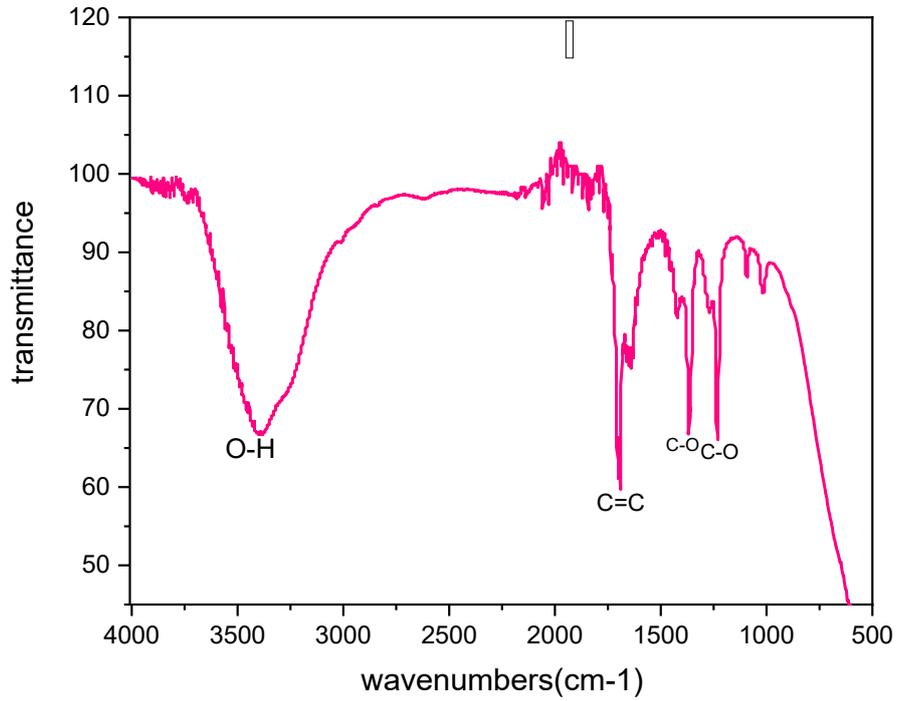
Fig. 9. FTIR spectra of GNPs /Chl. Nanocomposite.
