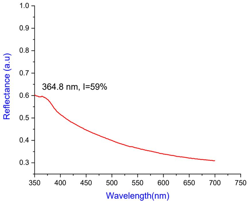
Fig. 11. The reflectance spectrum of GNPs/Chl./SiNWs nanocomposite.
