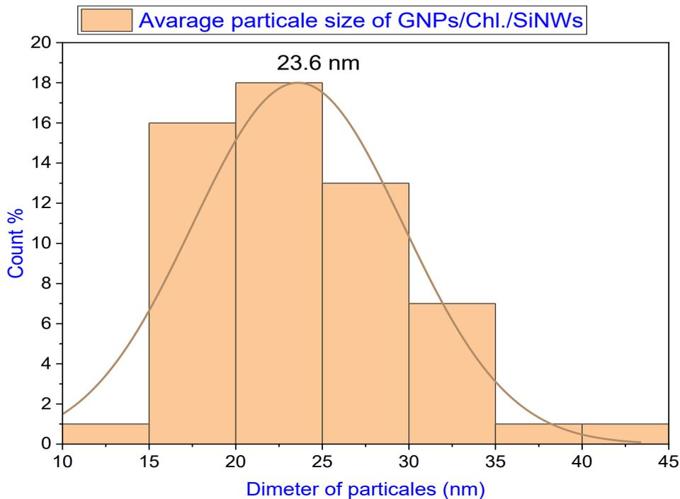
Fig. 8. The average particles size of GNPs/Chl./SiNWs Nanocomposite at PH=3.
