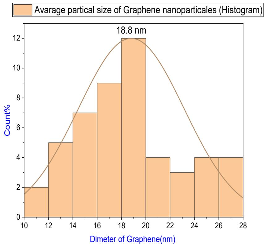
Fig. 6. The average particles size of GNPs.
