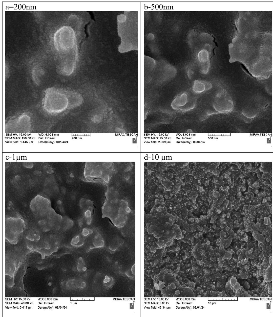
Fig. 7. The FESEM of GNPs/ Chlorophyll/ / SiNWs nanocomposite, a-200nm b-500nm c- 1µm d-10 1µm.
