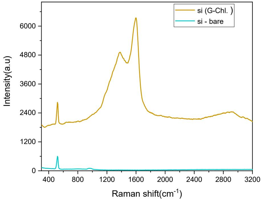
Fig. 12. The Raman spectrum of GNP/Chl./SiNWs nanocomposite.
