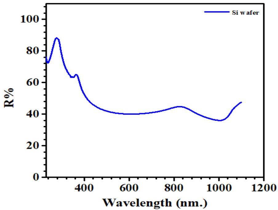
Fig. 10. The reflectance spectrum of Silicon wafer [58].
