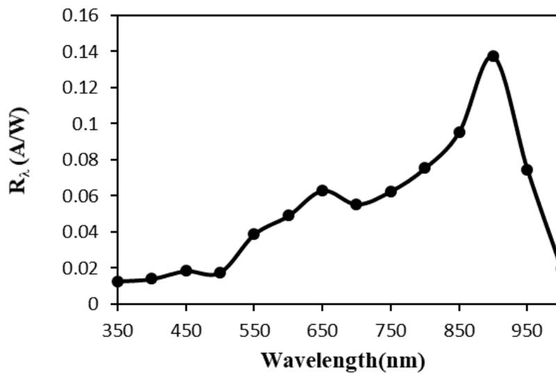
Fig. 13. The spectral responsivity as a function of wavelength.
