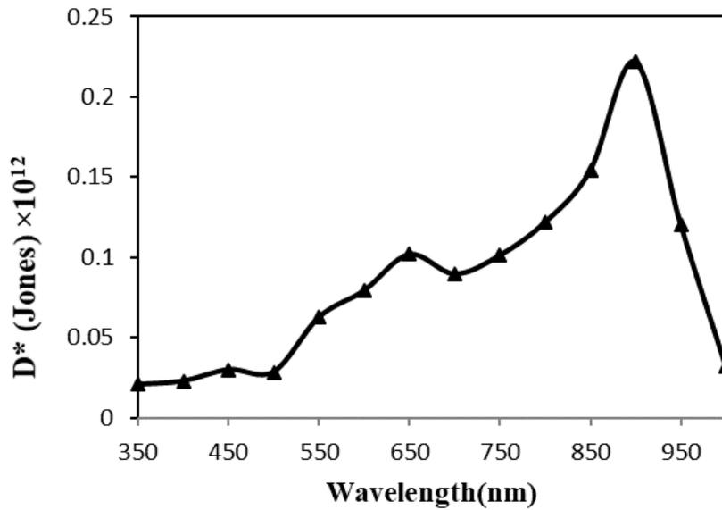
Fig. 14. The specific detectivity as a function of wavelength.
