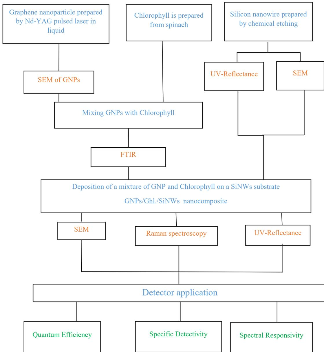
Fig. 1. Flow chart showing the steps for preparing and measurements of GNP/Ghl./SiNWs nanocomposite.
