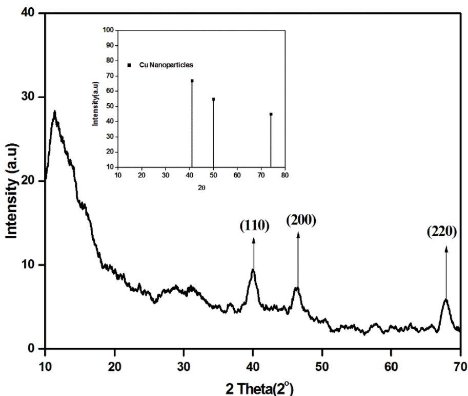
Fig. 3. XRD of copper Nanoparticles and JCPDS data of CuNPs (insert).
