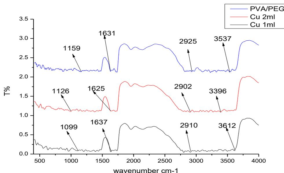
Fig. 9. FTIR analysis of PEG/PVA + CuNPs nanocomposite
