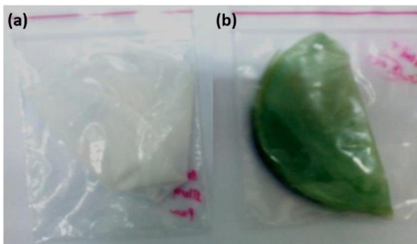
Fig. 2. (a) PVA/PEG and (b) PVA/PEG blended with CuNPs
