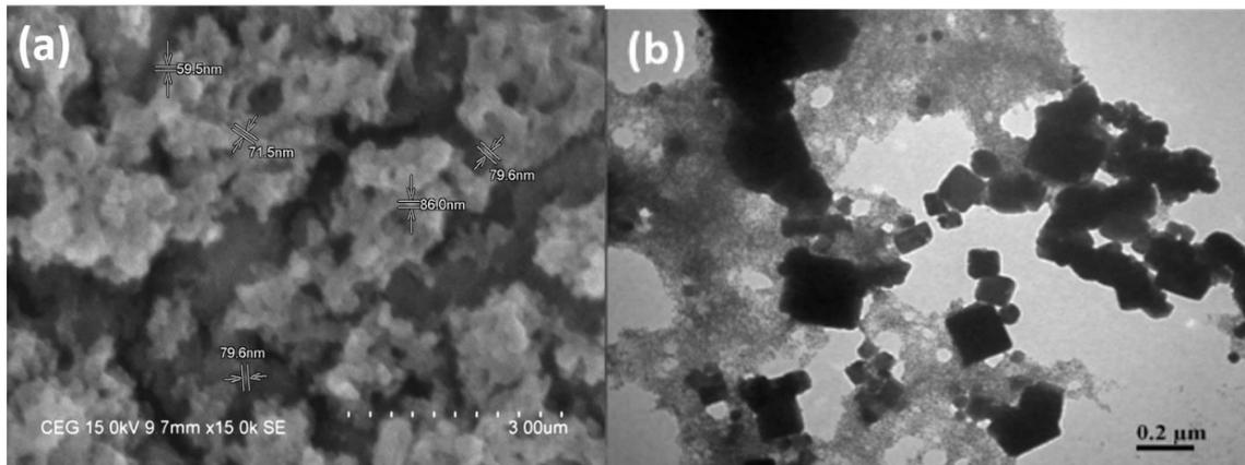
Fig. 6. (a) SEM and (b) TEM micrograph of CuNPs.
