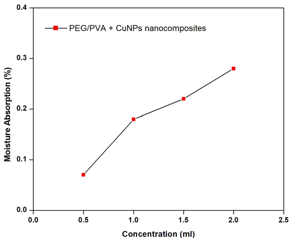
Fig. 10. Moisture absorption analysis of PEG/PVA + CuNPs nanocomposite.
