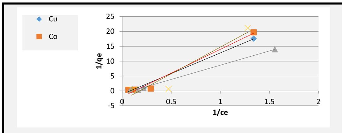
Fig. 8. Langmuir adsorption isotherm for metals adsorption by (NM semi IPN's) at pH=6, shaking rate 180 rpm, amount of adsorbent 0.05g)
