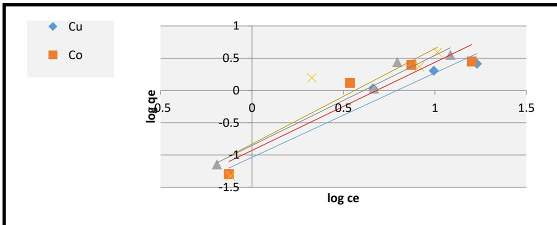
Fig. 9. Freundlich adsorption isotherm for metals adsorption by (NM semi IPN's) pH=6, shaking rate 180 rpm, amount of adsorbent 0.05g)
