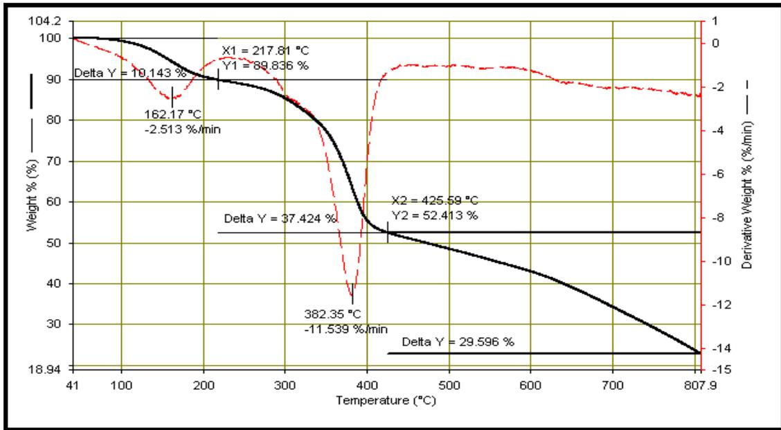
Fig. 2. TGA curve of (NM – IPN's)
