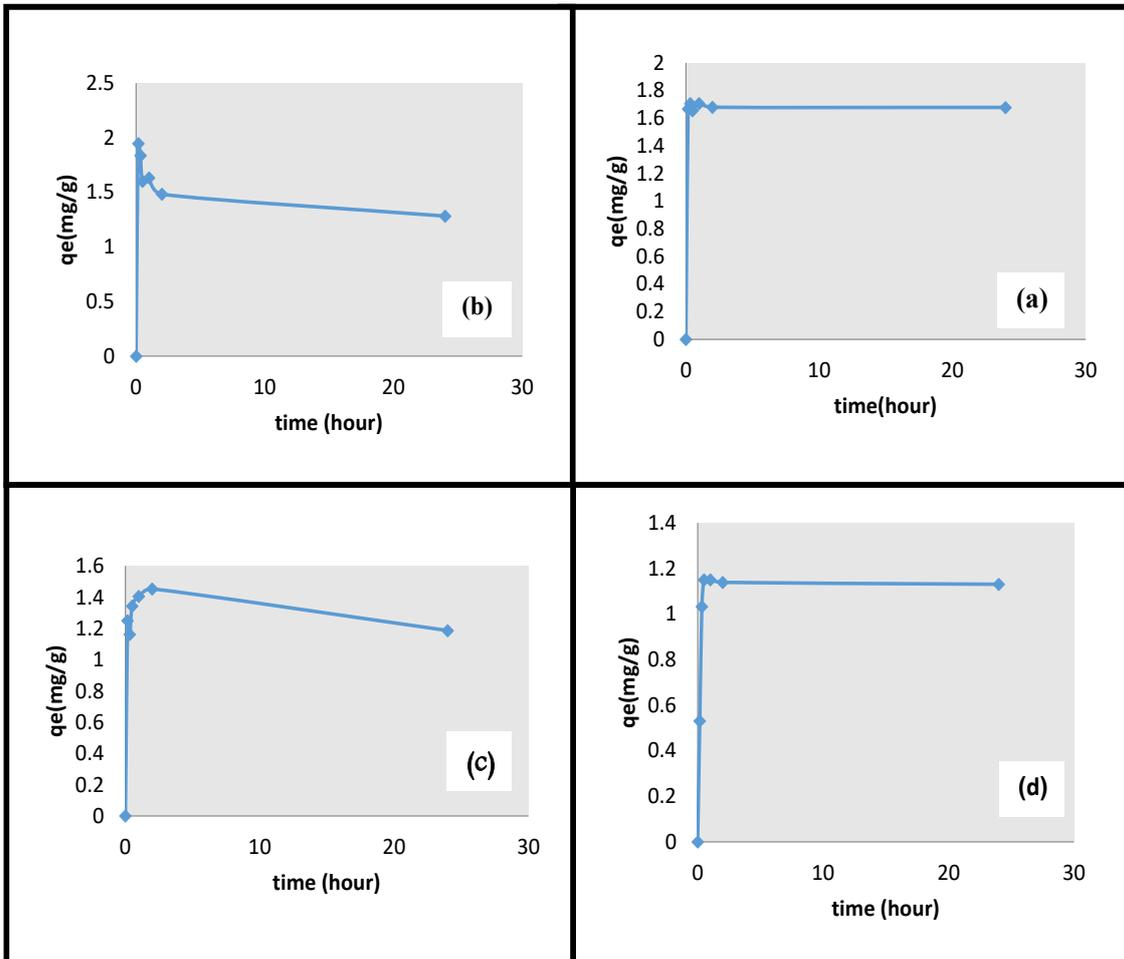
Fig. 7. Effect of contact time on metals removal by (NM semi IPN's) at pH=6: (a)  $Pb^{2+}$  (b)  $Cd^{2+}$  (c)  $Cu^{2+}$  (d)  $Co^{2+}$
